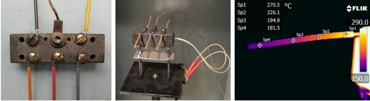
Figure 1. Photographs of pre-flaming smoke source with insulated conductors attached (thermocouple connection shown top center). Left photo shows plan view, center photo shows assembly installed in cabinet with heater cartridge installed, right photo shows thermal image of attached insulated conductor with temperature measurements at specific locations.
