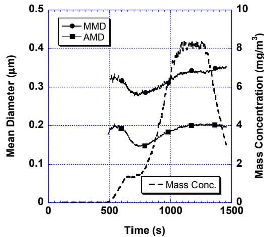
Figure 3. Mass mean diameter (MMD), arithmetic mean diameter (AMD) and mass concentration for XLPE wire and a 15-min heating ramp, with estimated combined relative uncertainties of  $\pm 20\%$  for MMD, AMD, and mass concentration.
