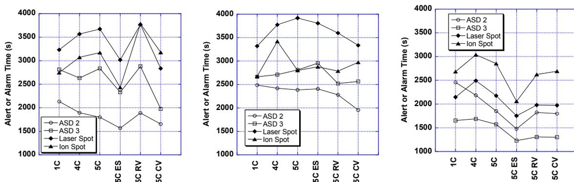
Figure 4. Alert and Alarm times for various full-scale experimental configurations for XLPE (left), PVC (center) and CSPE (right)
