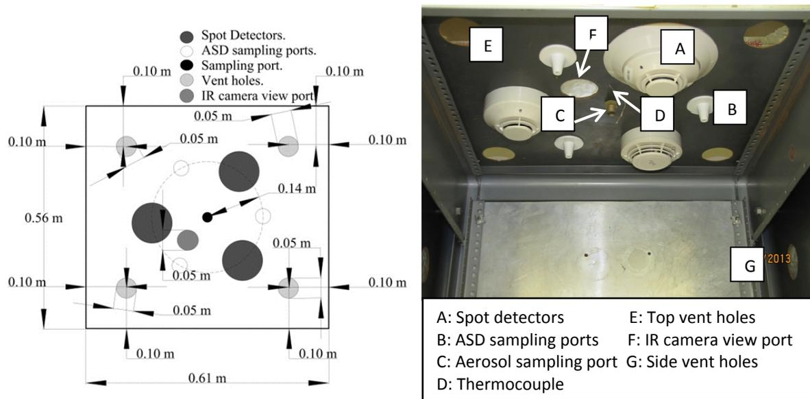
Figure 2. Illustration and photograph of in-cabinet smoke detection layout
