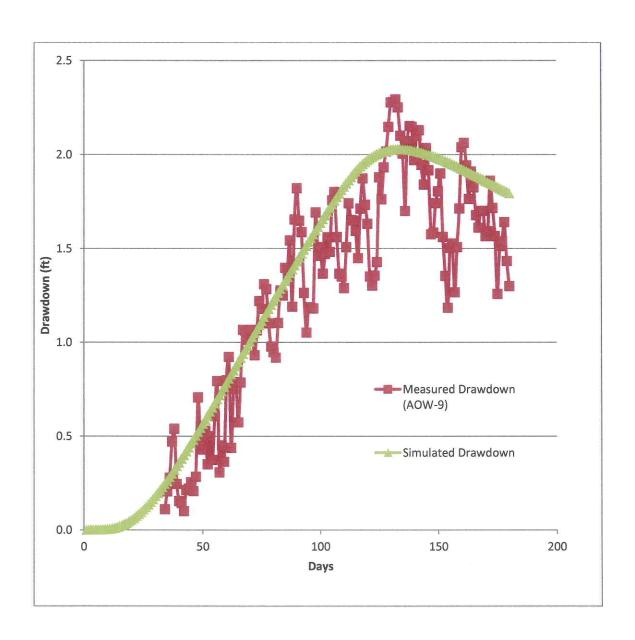
Figure 2. Simulated vs. Observed Drawdown in shallow monitoring well AOW-09, Irrigation Well 732 calibration .
