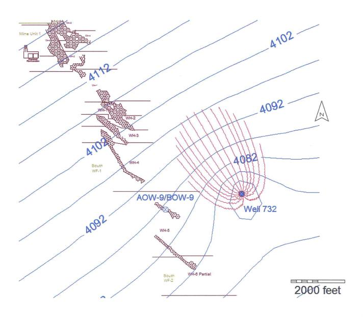
Figure 3. 30-year capture zone of Irrigation Well 732.
