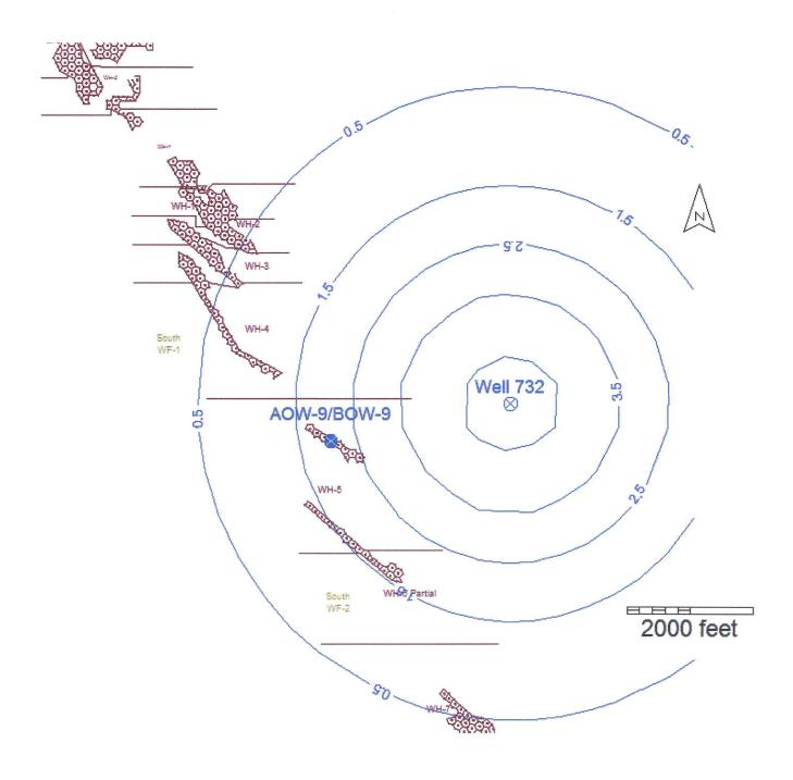
Figure 1. Calibrated maximum drawdown contour map, 2014 Irrigation Season.
