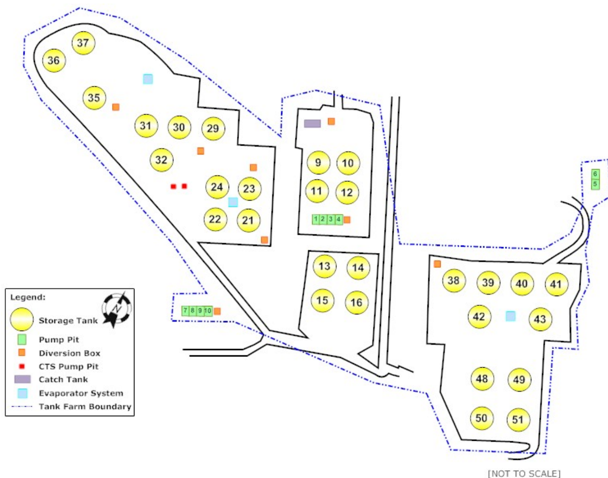
Figure 3.2-3: General Layout of H-Tank Farm
