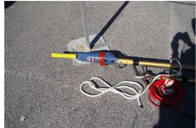
Sampling devise used in sampling of Tank 16 annulus
