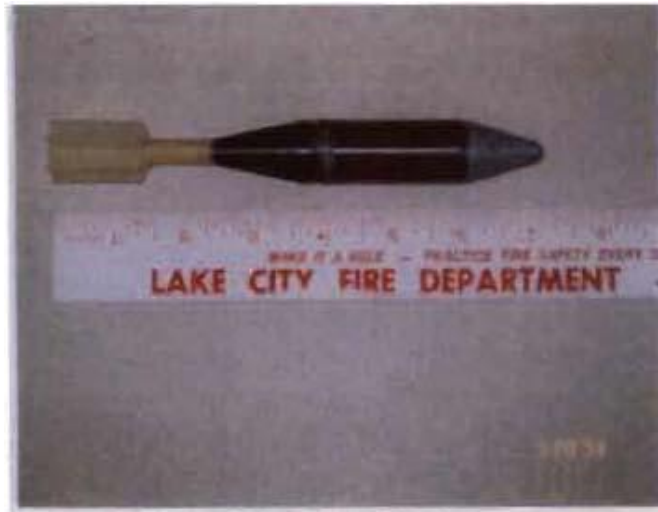
Figure 1-1 Davy Crockett M101 spotting round
