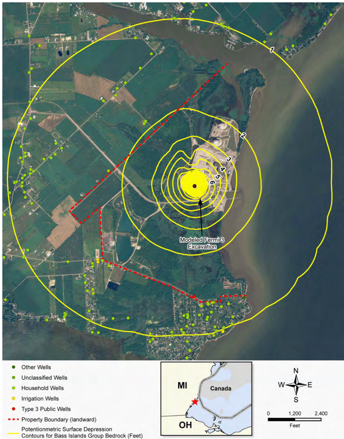
Figure 2.3-42 Dewatering Bass Islands Group: Drawdown Contours – Grout Curtain/Freeze Wall Combination with a Grouted Base
