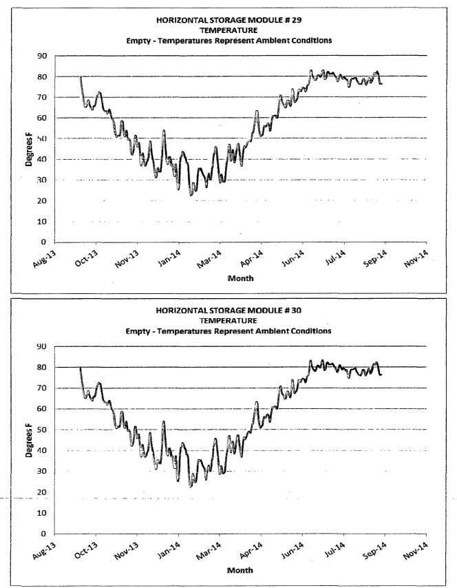
Enclosure 2 Oyster Creek Nuclear Generating Station Independent Spent Fuel Storage Installation Temperature Monitoring Graphs
