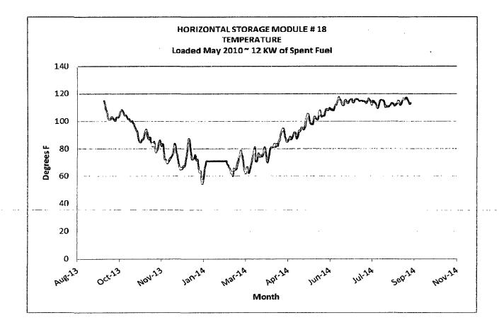
Enclosure 2 Oyster Creek Nuclear Generating Station Independent Spent Fuel Storage Installation Temperature Monitoring Graphs
