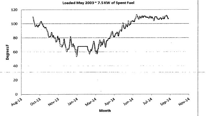
Enclosure 2 Oyster Creek Nuclear Generating Station Independent Spent Fuel Storage Installation Temperature Monitoring Graphs
