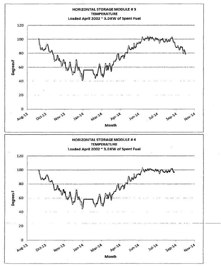
Enclosure 2 Oyster Creek Nuclear Generating Station Independent Spent Fuel Storage Installation Temperature Monitoring Graphs
