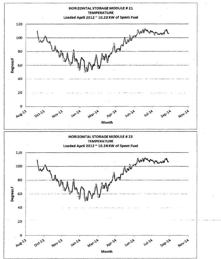
Enclosure 2 Oyster Creek Nuclear Generating Station Independent Spent Fuel Storage Installation Temperature Monitoring Graphs
