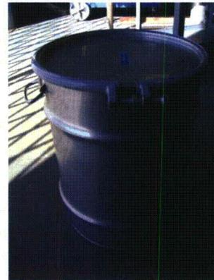
Figure 2: Drum With Handles Intact After Test
