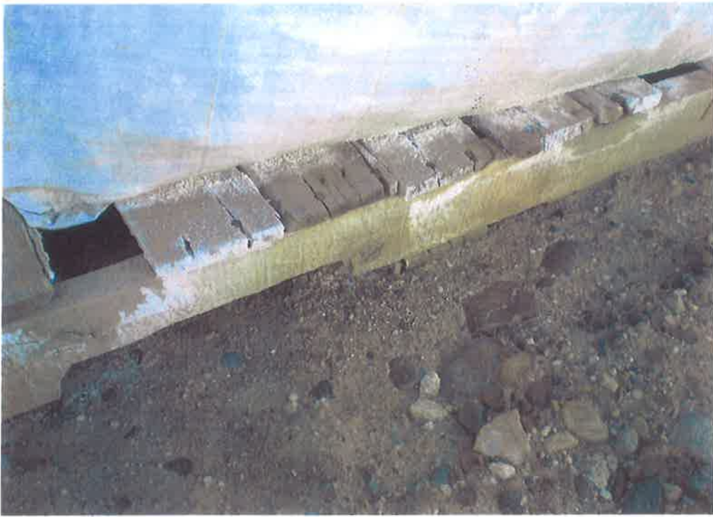
Photo 7 Third container – leached waste through container liner onto pallet.
