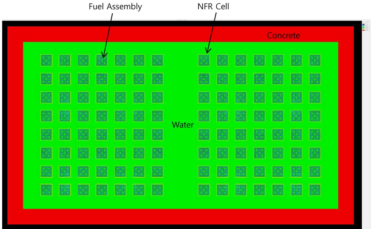
Figure 2.4-1 Criticality Calculation Model for the NFR in a New Fuel Storage Pit
