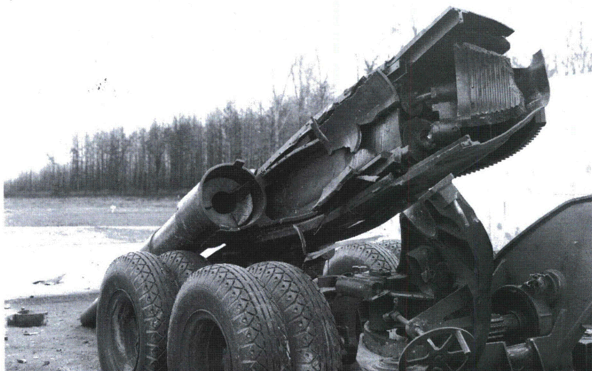
Why we test! Ammunition malfunction in the tube.
