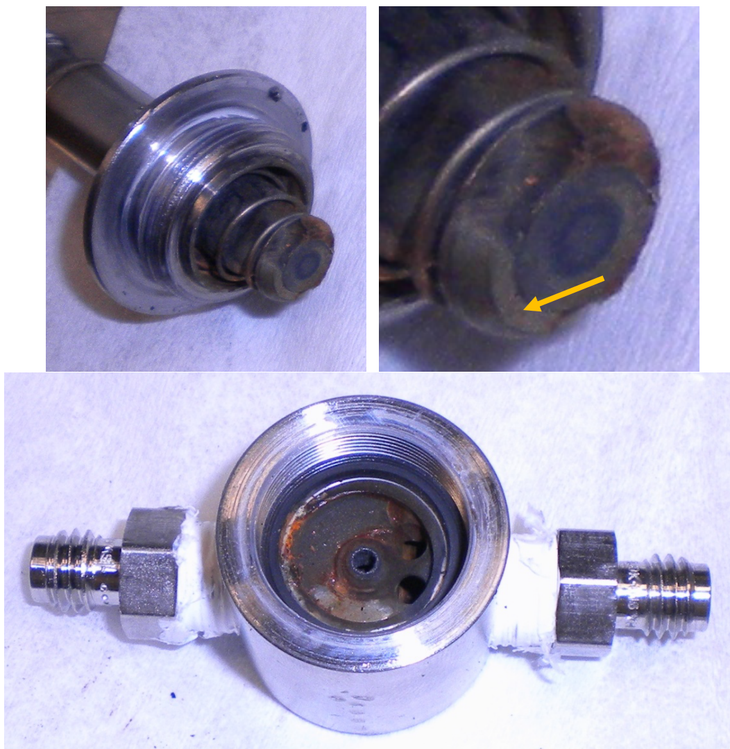
FIGURE 2 Interior of the Irradiated Peter Paul Direct-Acting Solenoid Valve (Top left: Plunger [piston] and outer assembly showing the spring that holds pressure on the plunger to maintain a seal between the rubber insert and the orifice. Top right: Magnified view of the tip of the plunger with an arrow showing the interface between the rubber seal and plunger body. Bottom center: Body interior showing the orifice [center hole] that is sealed by the rubber seal on the plunger.)
