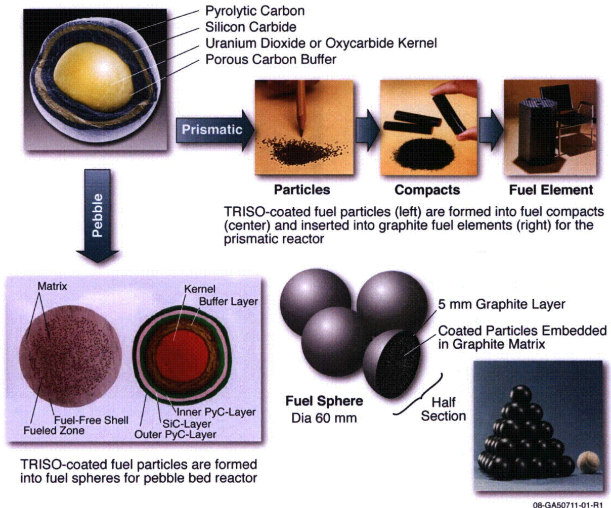
Figure 9. Prismatic and Pebble Bed TRISO Fuel.
