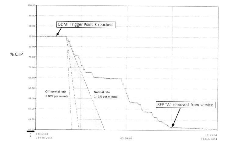
The reduction in power to 40% to remove RFP "A" from service is shown in the figure below.
