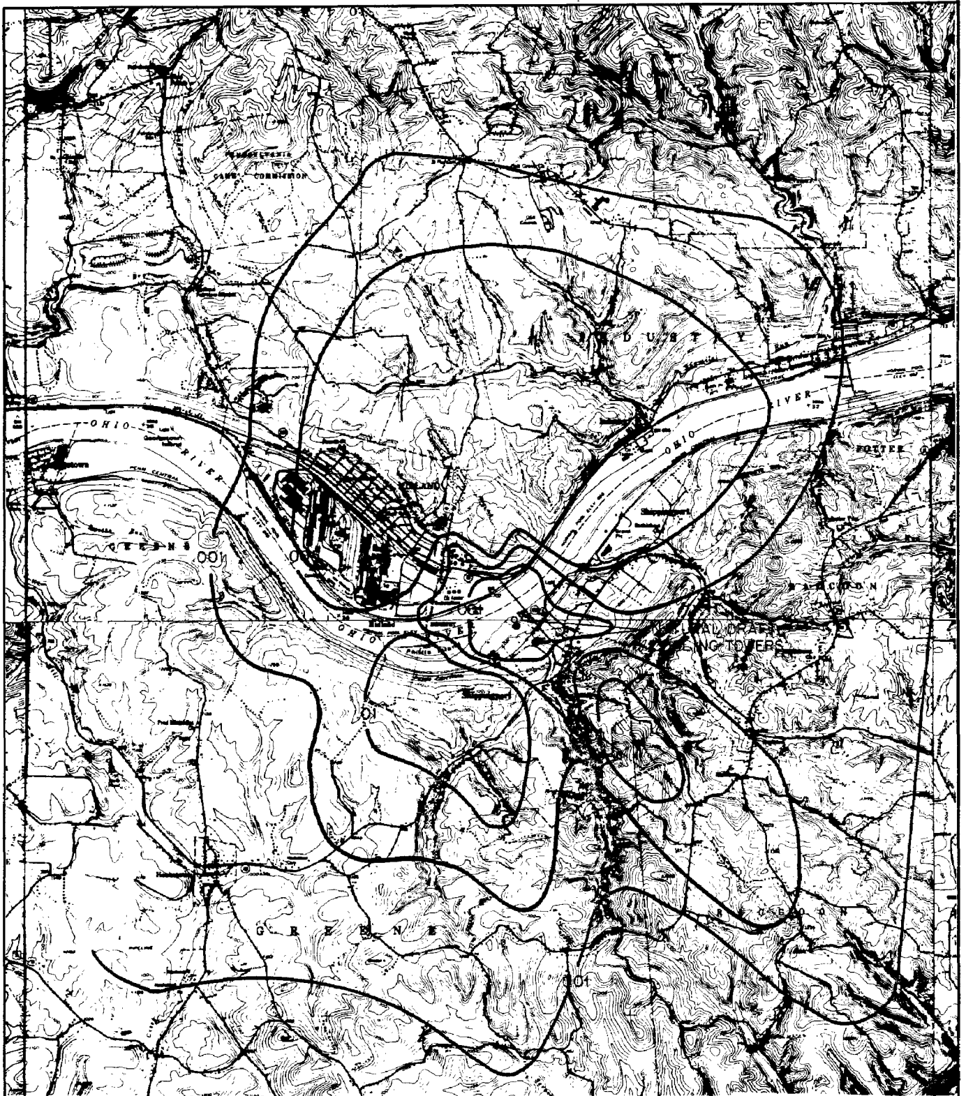
FIGURE 2.3-12 ICING DUE TO DRIFT FROM BVPS-1 AND BVPS-2 (INCHES/YEAR) NATURAL DRAFT COOLING TOWERS BEAVER VALLEY POWER STATION-UNIT 2 FINAL SAFETY ANALYSIS REPORT
