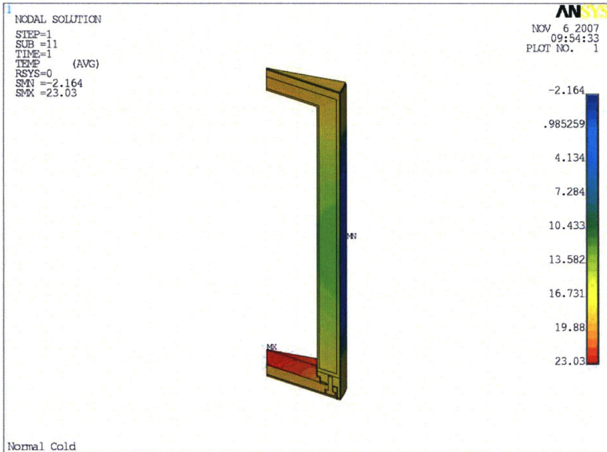
Figure 3-7 - Temperature Distribution – Normal Cold
