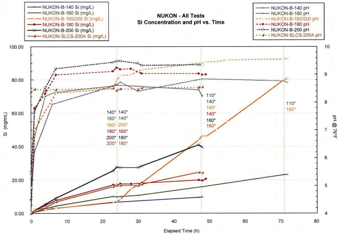
Figure 39 – NUKON-B Test Series ICP Data - Si
