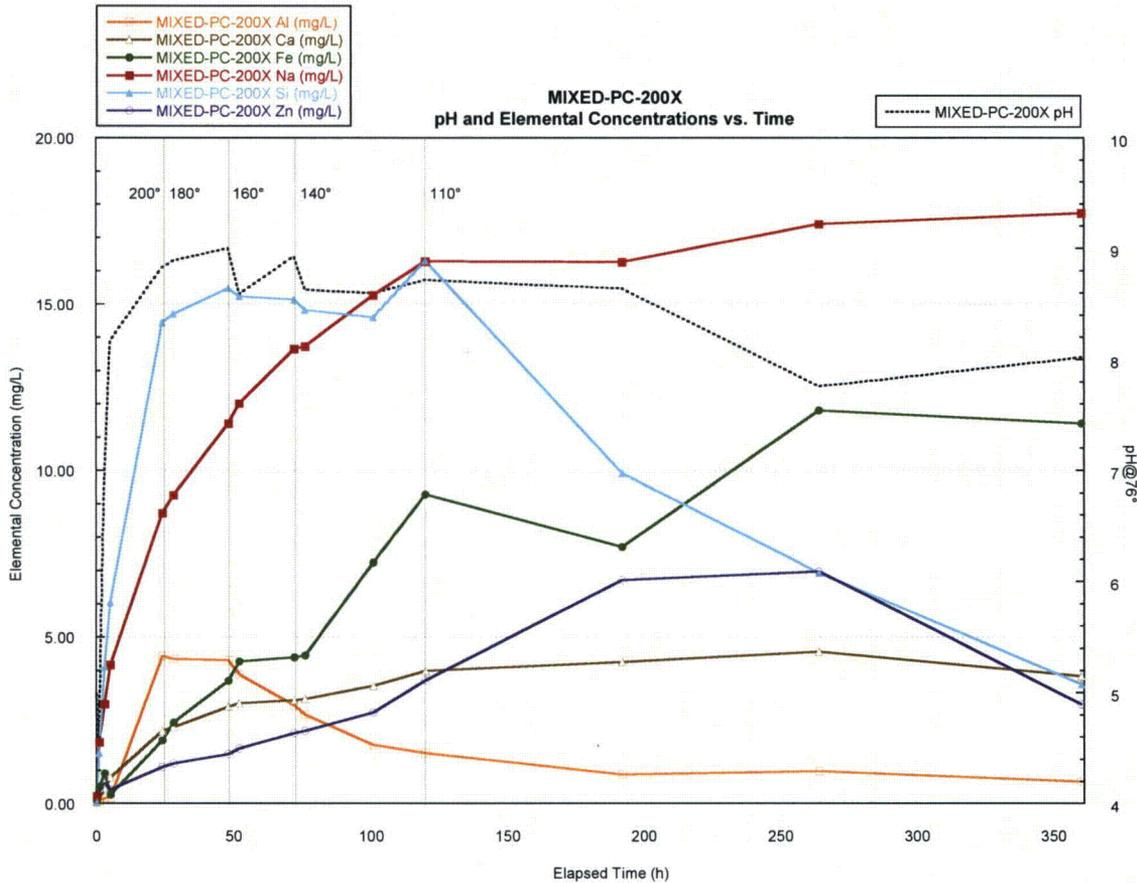
Figure I01 – Plot of ICP Data from Test MIXED-PC-200X
