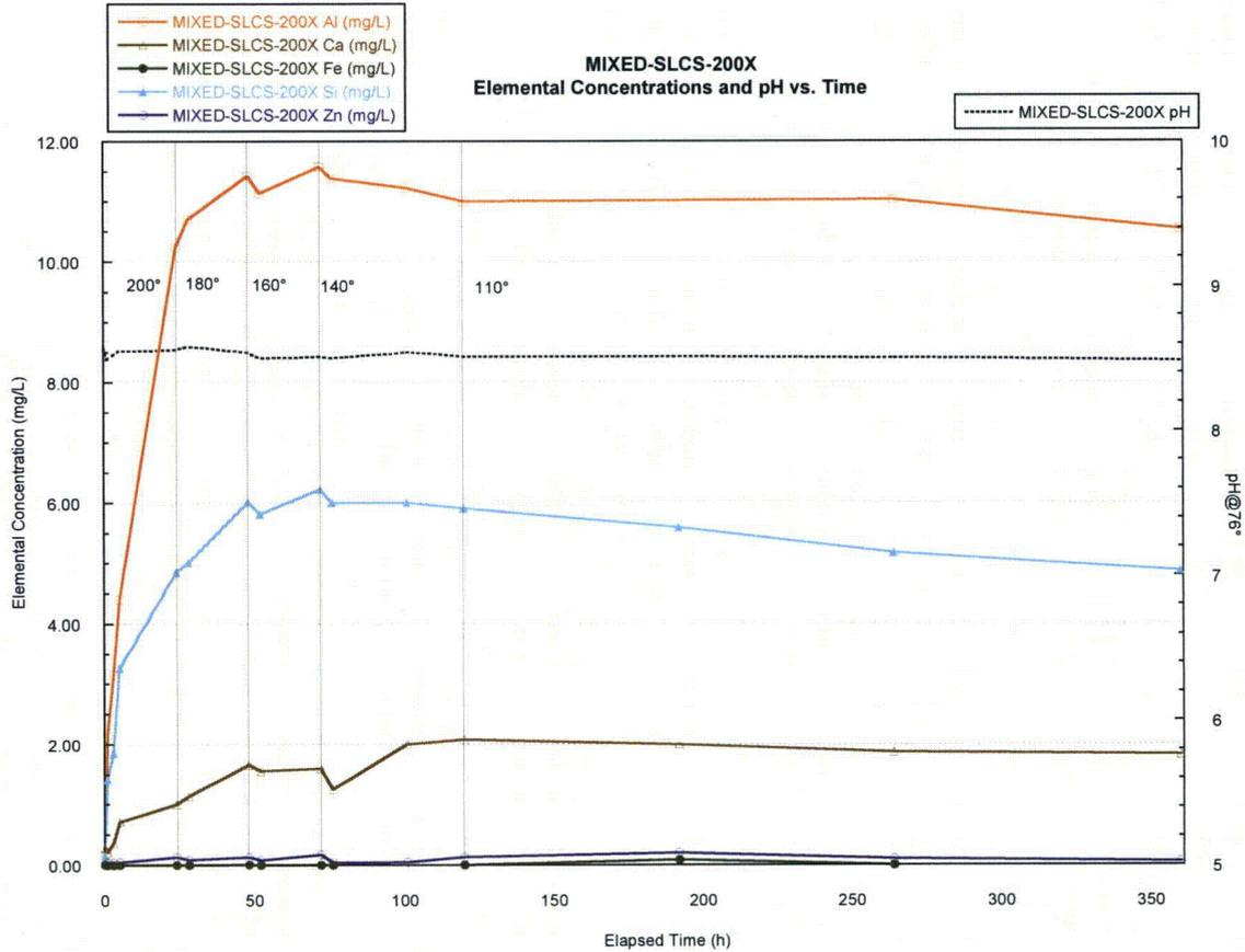
Figure I21 – Plot of ICP Data from Test MIXED-SLCS-200X
