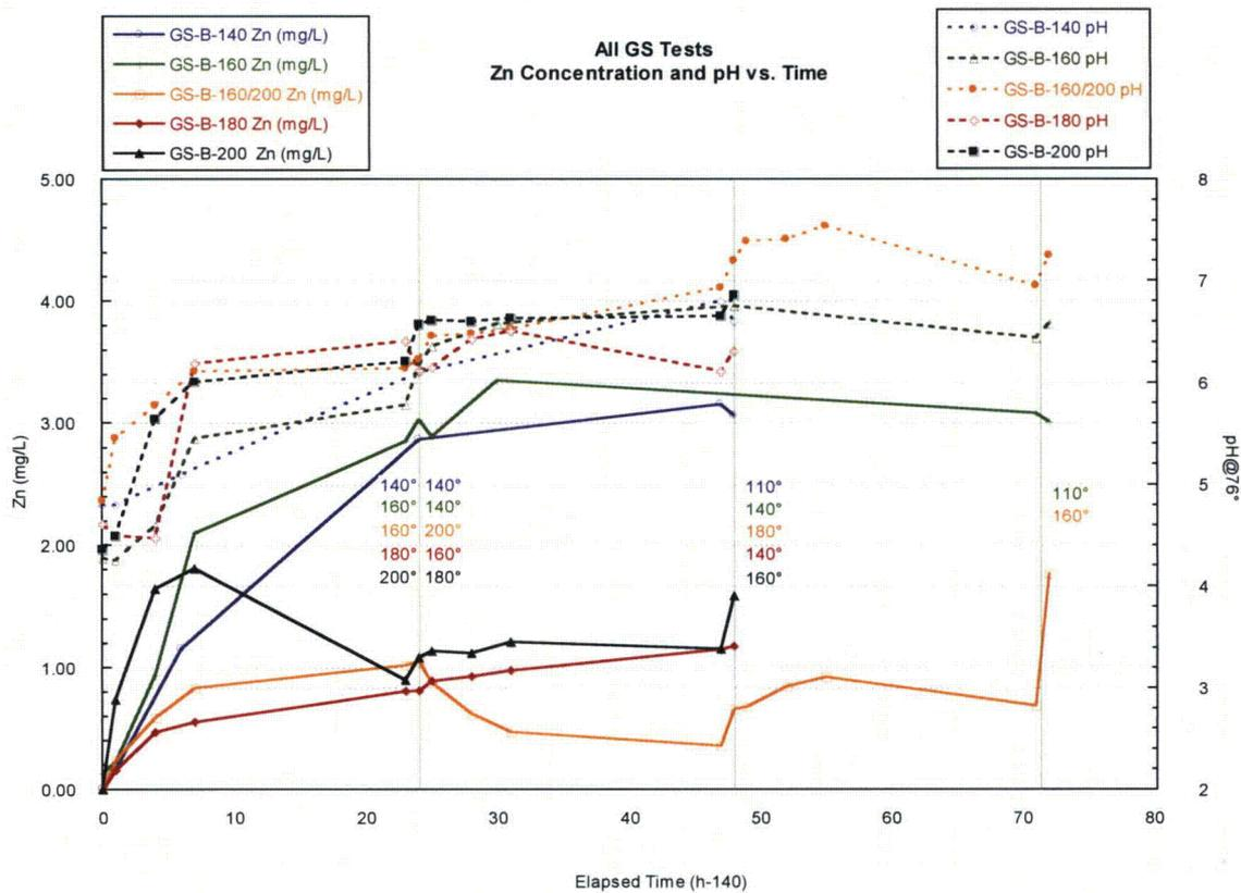
Figure 63 – GS Zinc Concentrations and pH vs. Time
