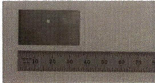
Figure 2 – Sample Pre-Test Metallic Coupon
