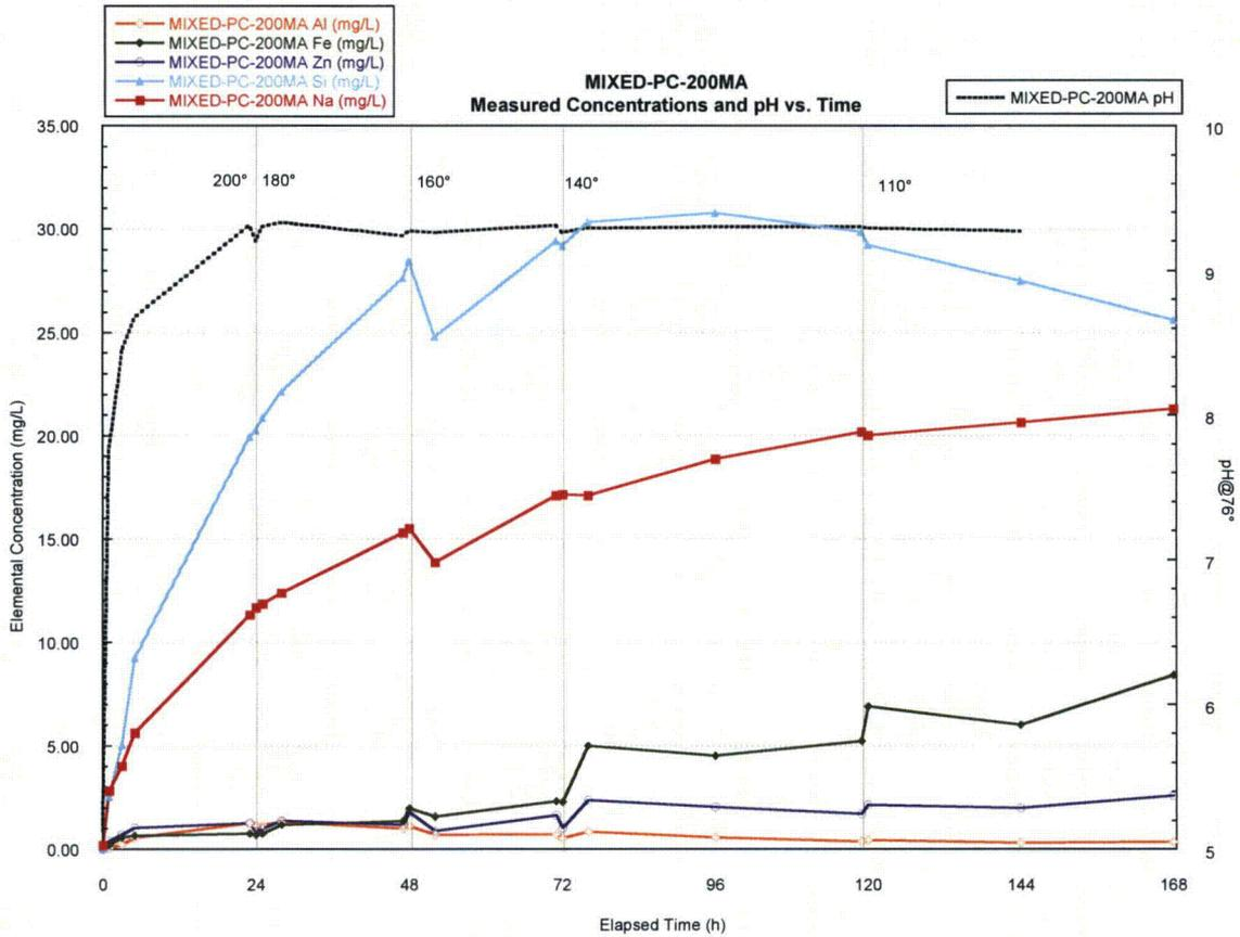
Figure 77 – Plot of ICP Data from Test MIXED-PC-200MA
