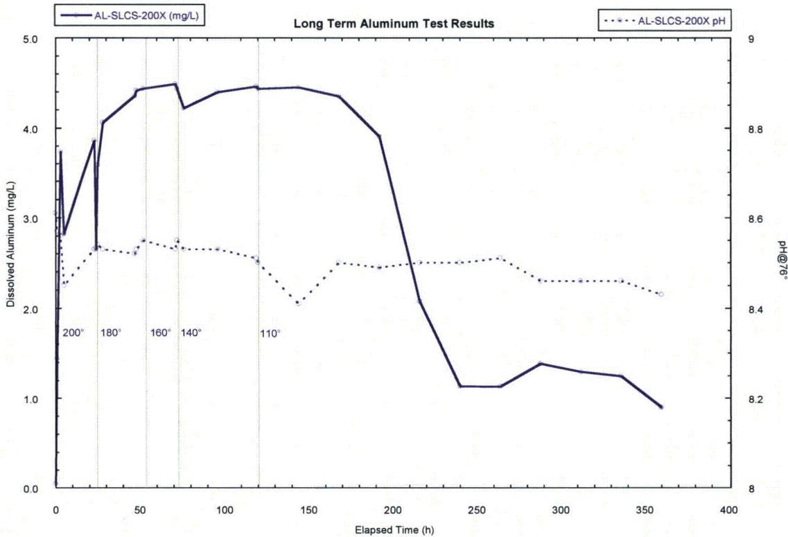
Figure 13 – Long Term Aluminum SLCS Test Results – AL-SLCS-200X
