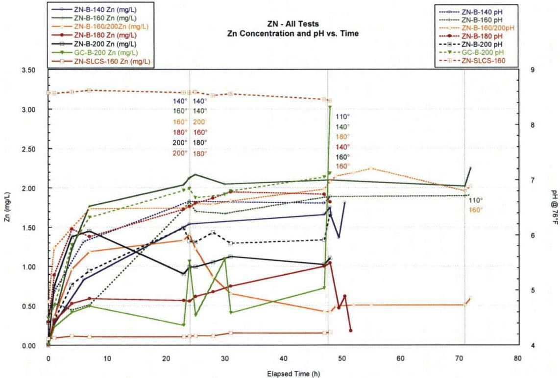
Figure 44 – Zinc Concentrations and pH vs. Time
