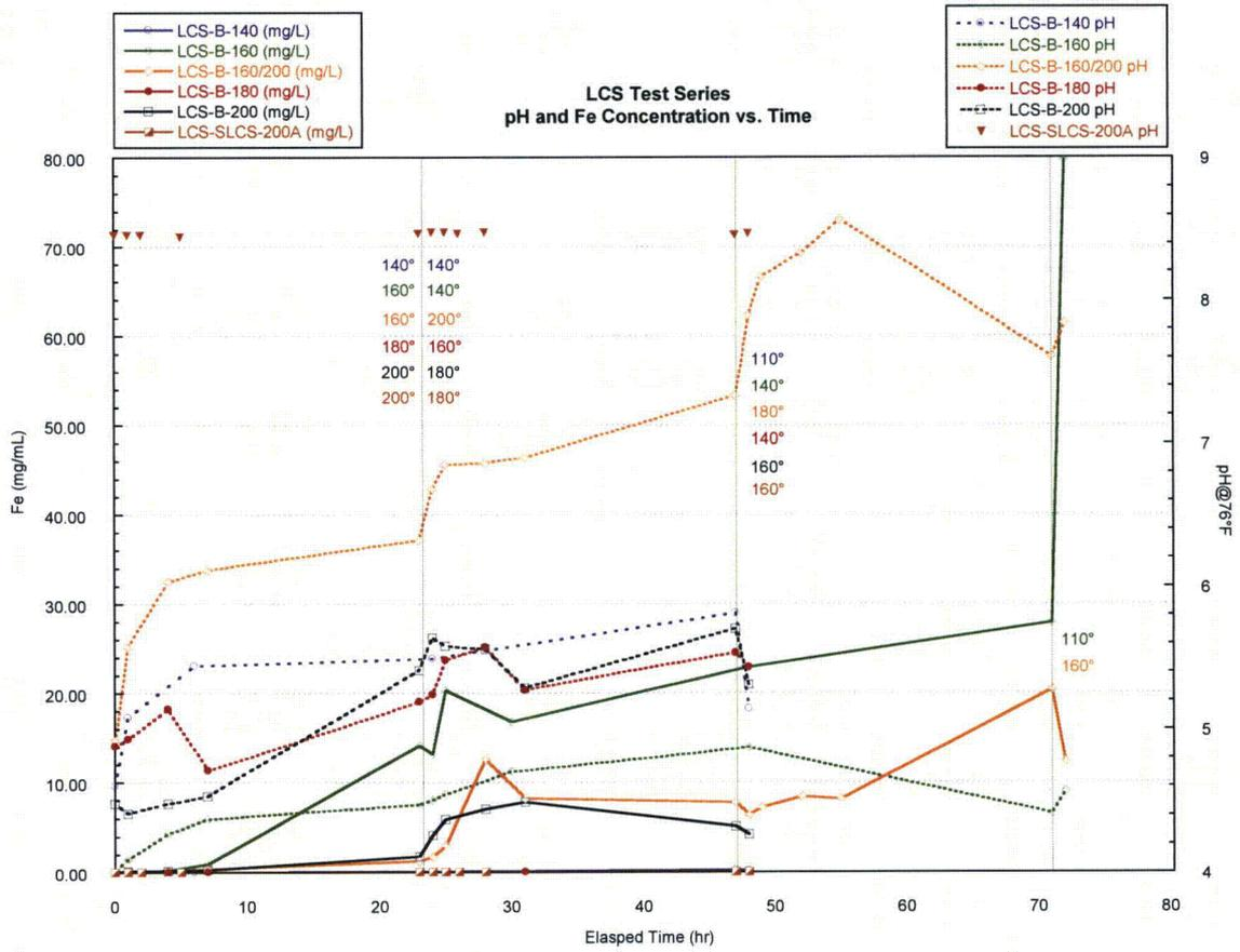
Figure 22 – Fe Concentrations and pH vs. Time
