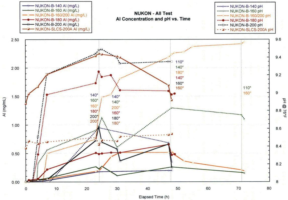
Figure 35 – NUKON-B Test Series ICP Data – Al – Higher Range for SLCS
