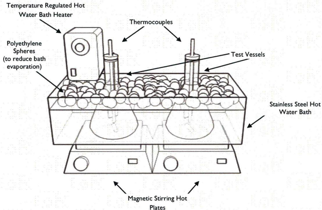
Figure 1 – Test Apparatus
