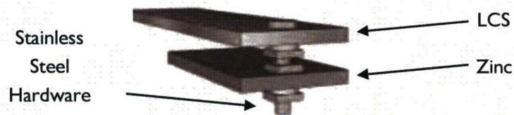
Figure 4 – Galvanic Cell Construction
