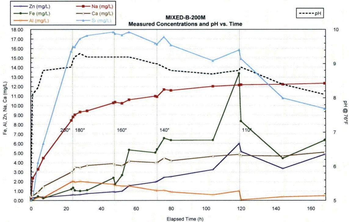
Figure 68 – MIXED-B-200M – Concentrations and pH vs. Time
