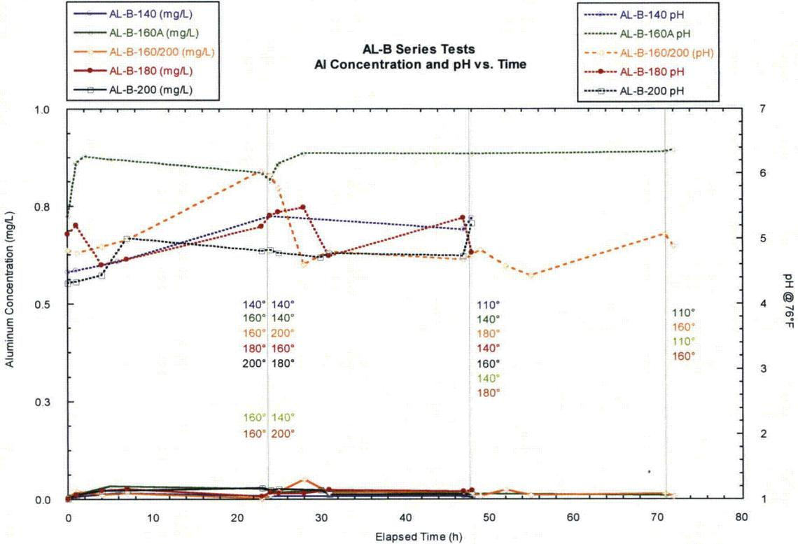
Figure 10 – Aluminum Concentrations and pH vs. Time – AL-B Series Tests
