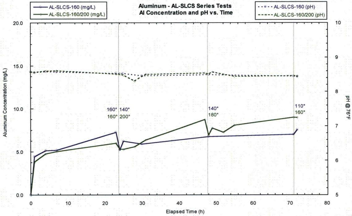
Figure 11 – Aluminum Concentrations and pH vs. Time – SLCS Series
