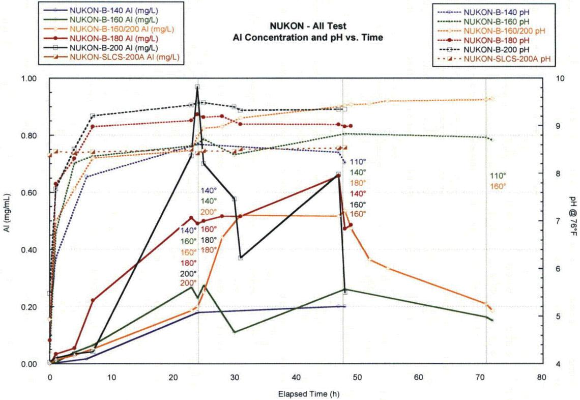
Figure 36 – NUKON-B Test Series ICP Data – Al
