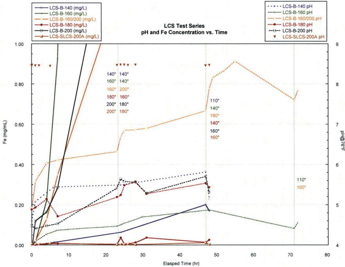
Figure 23 – Fe Concentrations and pH vs. Time – Detail
