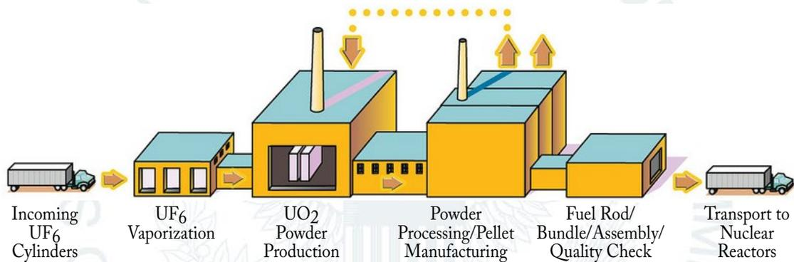
Fabrication of commercial light-water reactor fuel consists of the following three basic steps:
