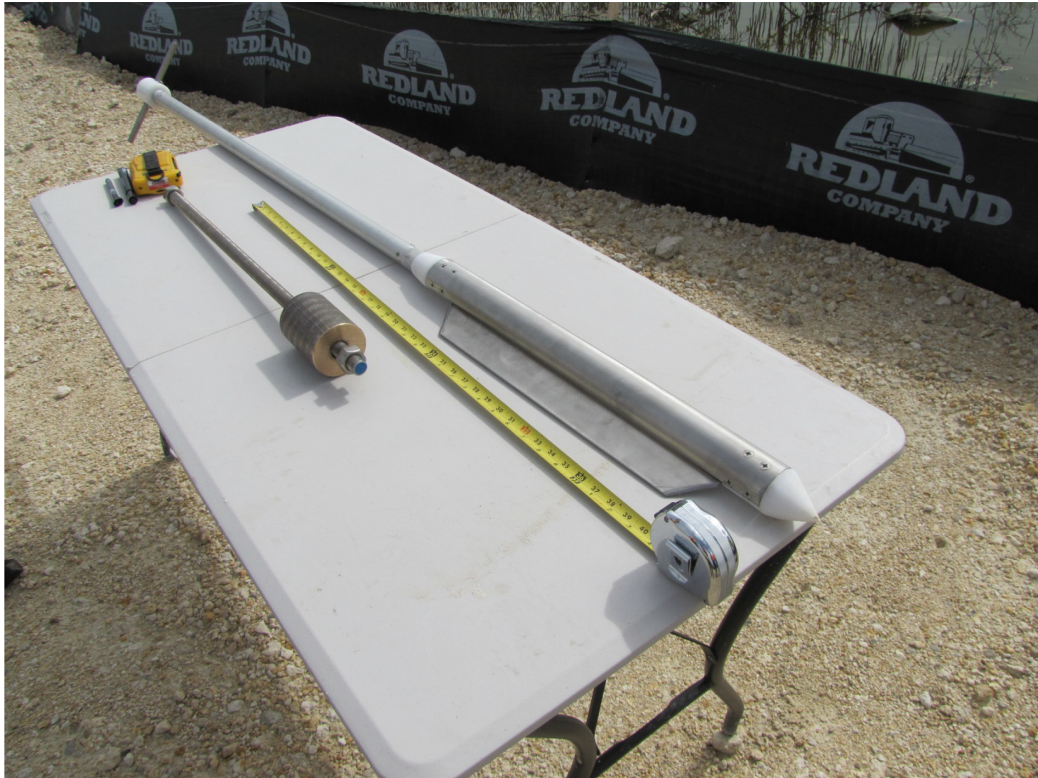
Figure 2-4 Core Barrel in Locked Finishing Position Prepared for Florida Power & Light Miami-Dade County, Florida
