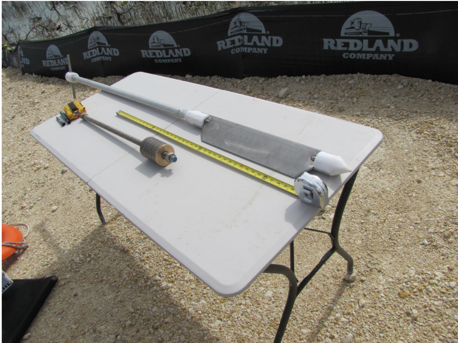
Figure 2-2 Core Barrel in Locked Starting Position Prepared for Florida Power & Light Miami-Dade County, Florida
