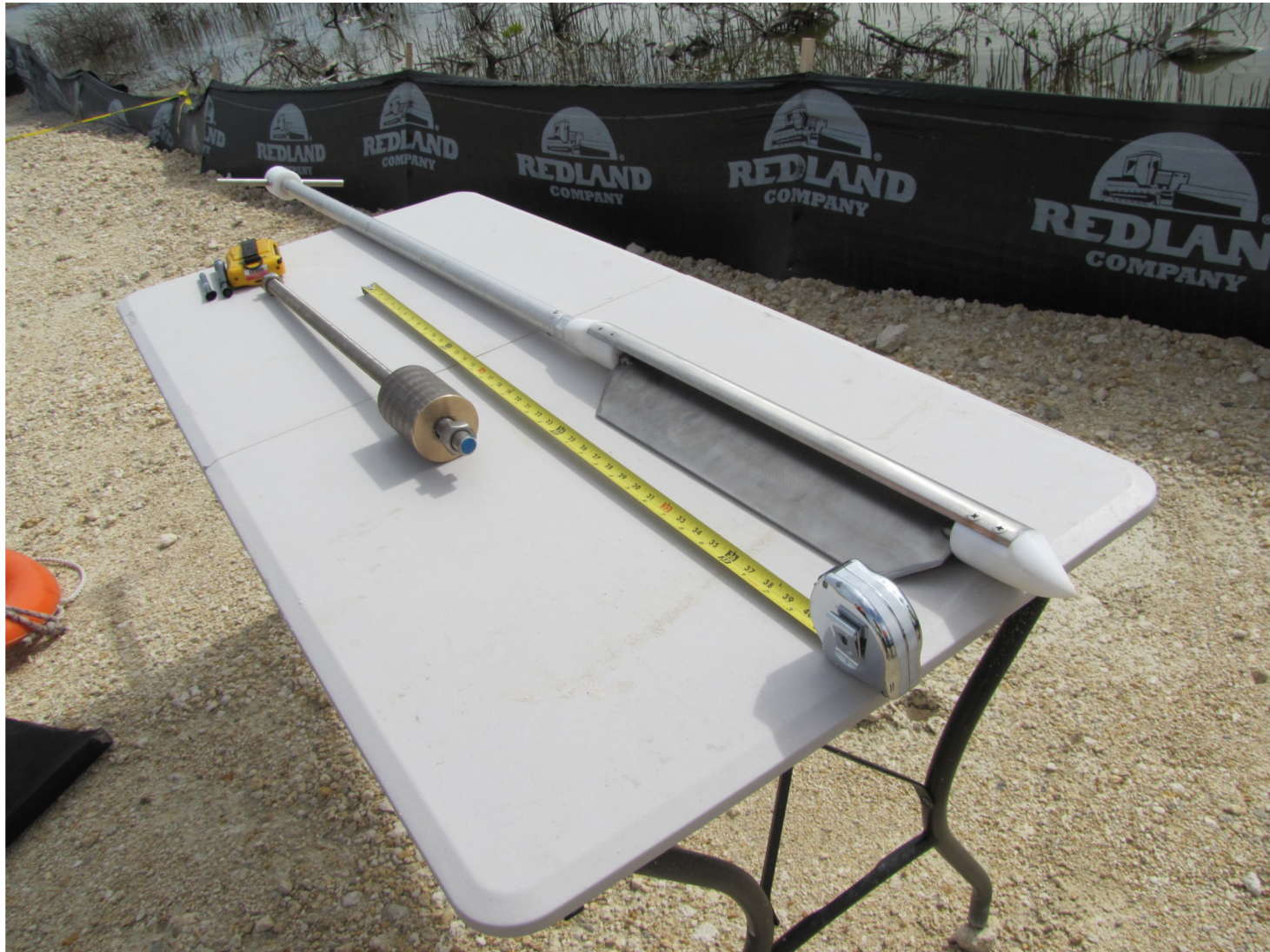
Figure 2-3 Core Barrel During Cutting Process Prepared for Florida Power & Light Miami-Dade County, Florida
