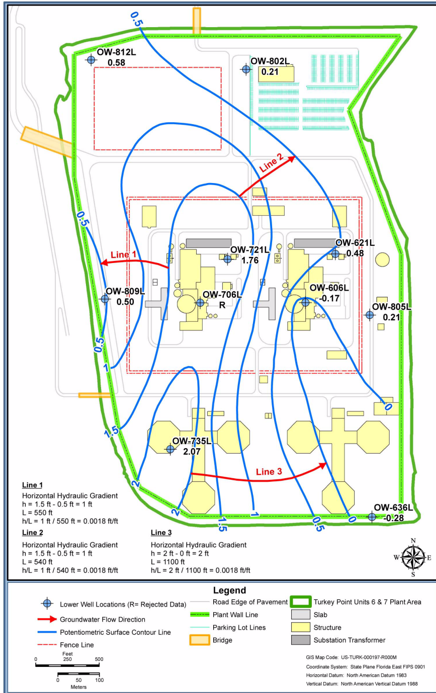
Figure 2.3-29 Biscayne Aquifer Potentiometric Surface Map, Lower Monitoring Interval, June 29, 2008 (Sheet 2 of 2) Low Tide
