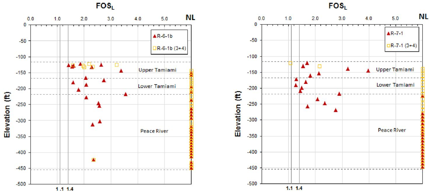
Note: NL corresponds to Non-Liquefiable locations  $(N_1)_{60} \geq 30$ . No numerical FOS value is obtained.
