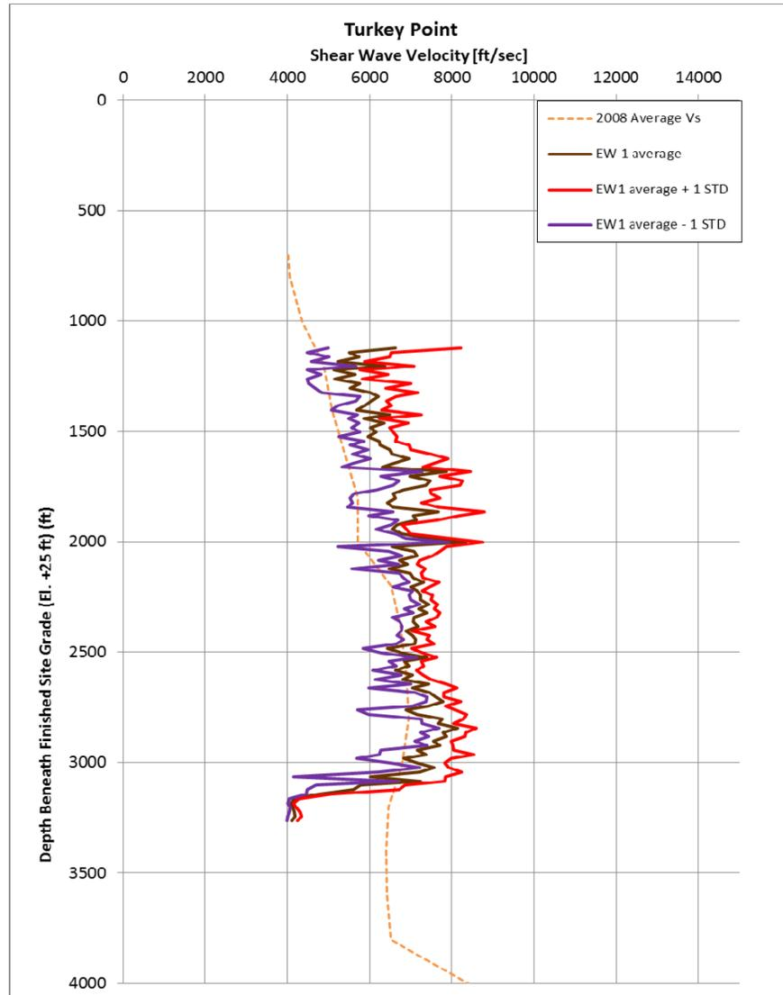
Note: The calculated averages for the “2008 Average  $V_s$ ” values are computed in 100-foot and 200-foot intervals. The EW-1 calculated average  $V_s$  values are in 20-foot intervals.
