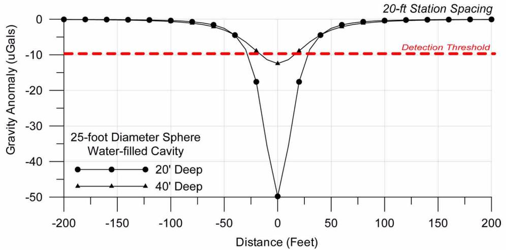
**Figure 2.5.4-224 Microgravity Models for Water-Filled Spherical Cavities in Limestone (Sheet 2 of 2)**
