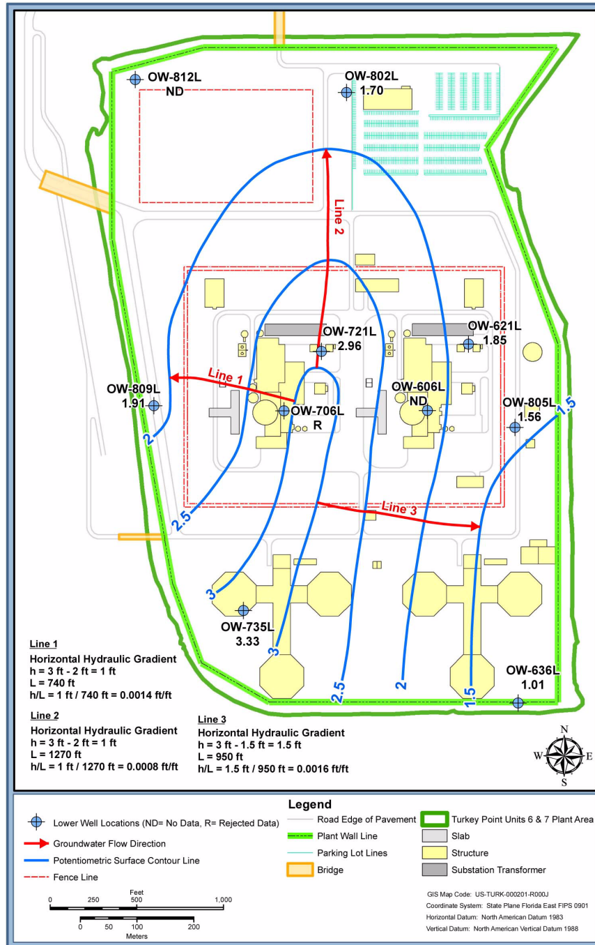
Figure 2.4.12-226 Biscayne Aquifer Potentiometric Surface Map, Lower Monitoring Interval, October 5, 2008 (Sheet 2 of 2) Low Tide
