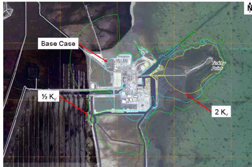
Figure 2CC-253 RCW Drawdown within the Top Layer - Sensitivity Case Biscayne Bay Vertical Hydraulic Conductivity
