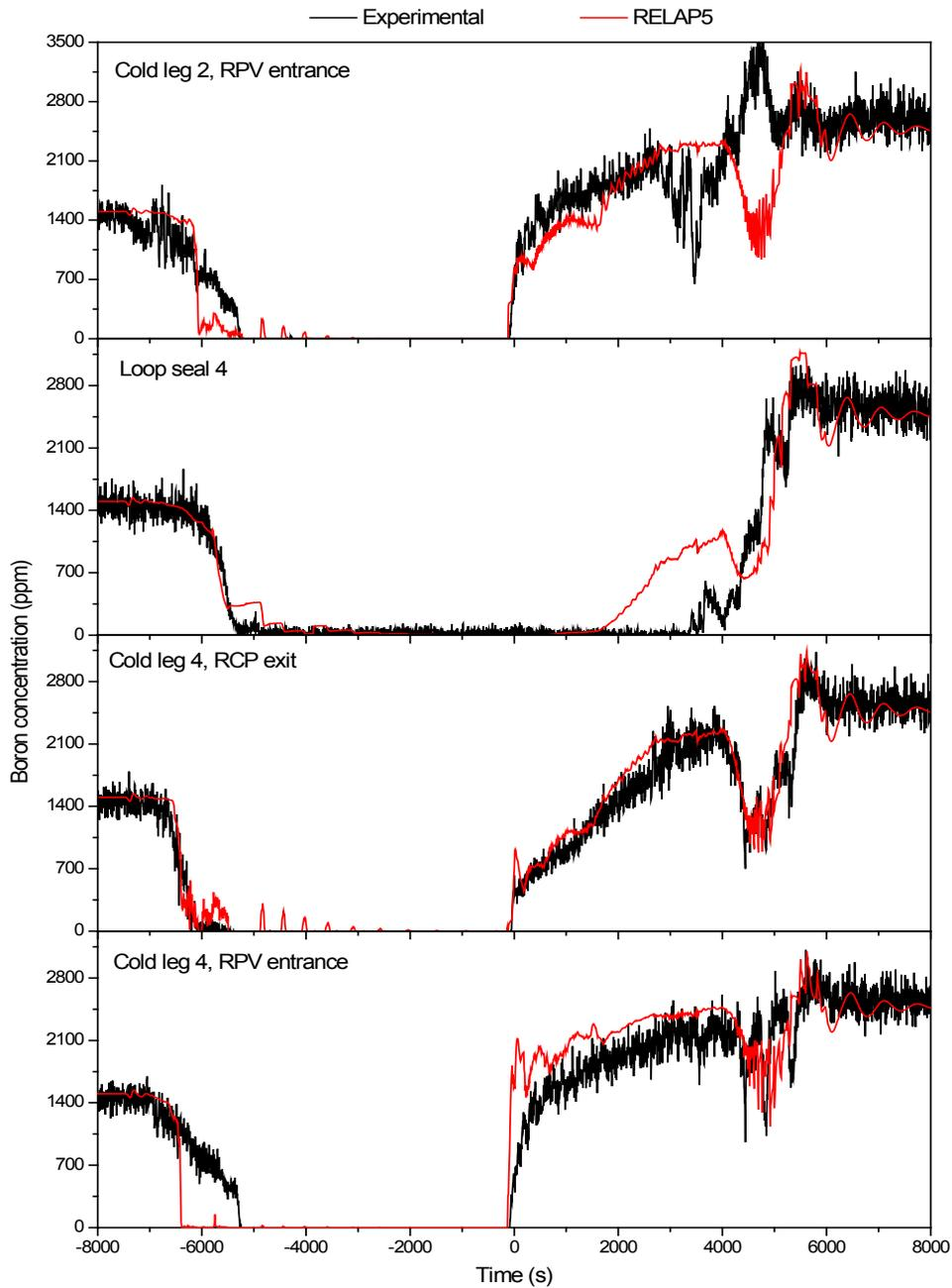
**Figure 2.9** Boron concentration at the COMBOs located in: cold leg 2, LS 4 and both sides of cold leg 4. Test F1.1
