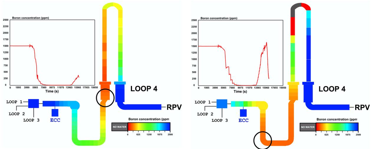
**Figure 2.13 Post test calculation of test F1.1, evolution of boron concentration in loop 4. Left: upward displacement of the slug continues. Right: the slug is moved back to the LS.**
