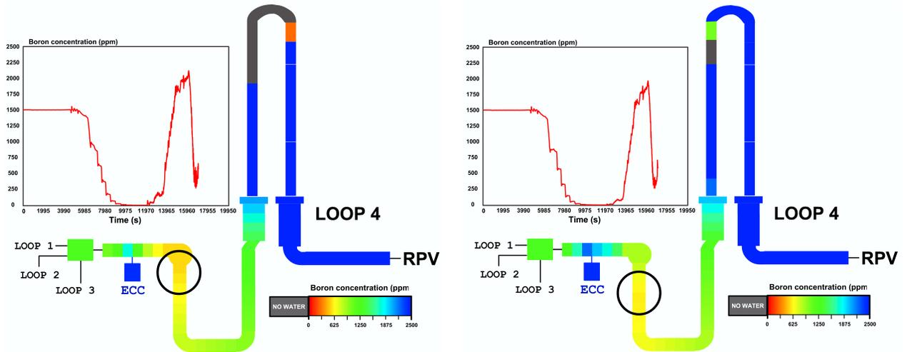
**Figure 2.15** Post test calculation of test F1.1, evolution of boron concentration in loop 4. Left and right: intermittent forward and backward movements of the slug.
