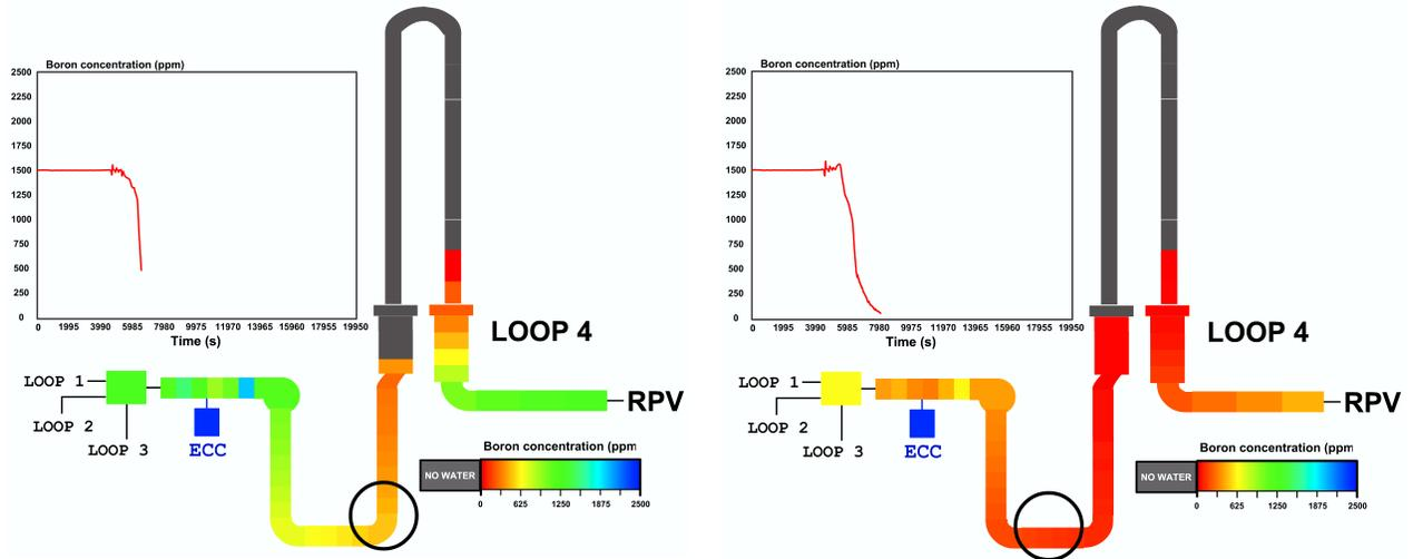
**Figure 2.11 Post test calculation of test F1.1, evolution of boron concentration in loop 4. Left and right: Boron dilution in hot leg and LS**
