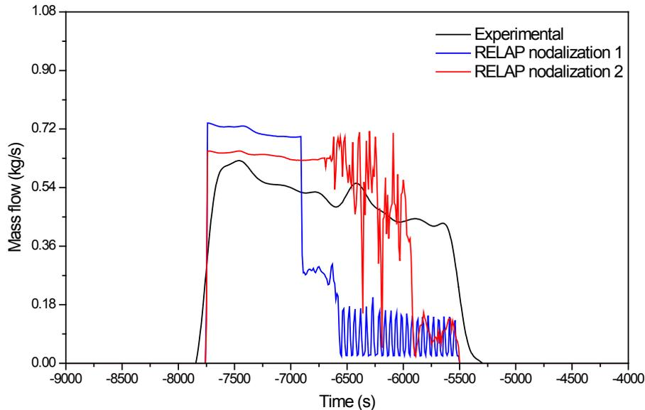
**Figure 4.1 Break mass flow during conditioning phase of Test F1.1, upper head bypass sensitivity**
