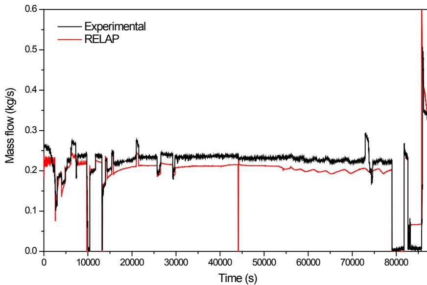
**Figure 3.3 Total main steam flow for Test F1.2**
