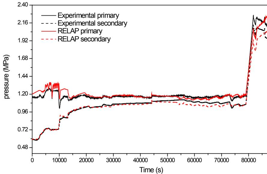
**Figure 3.1 Primary and secondary pressures for Test F1.2**
