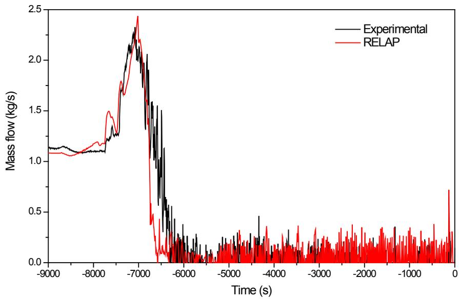
**Figure 2.2 Mass flow in loop 4, conditioning phase**
