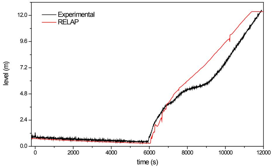
**Figure 2.6 Pressurizer level for test F1.1**
