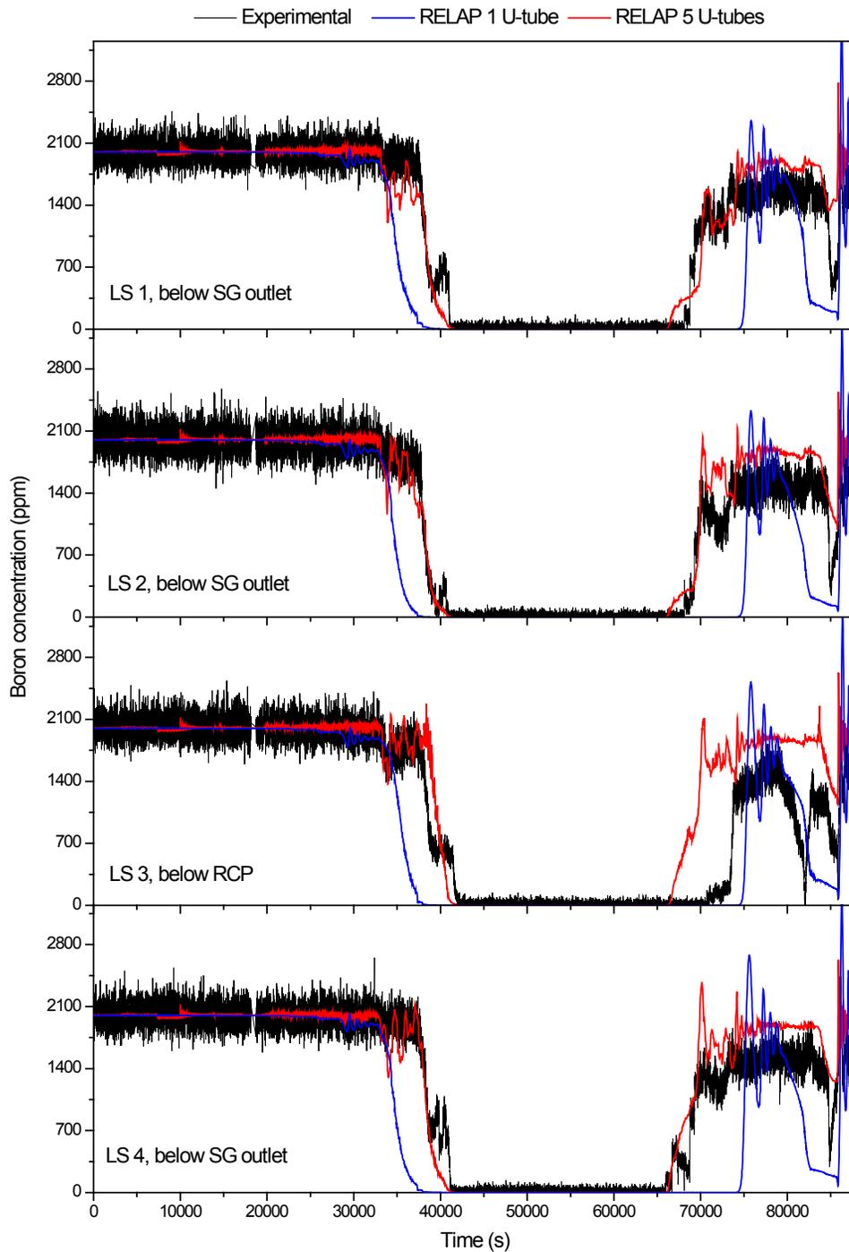
**Figure 4.7 Boron concentration in all LSs for Test F1.2 with 1 and 5 U-tubes**
