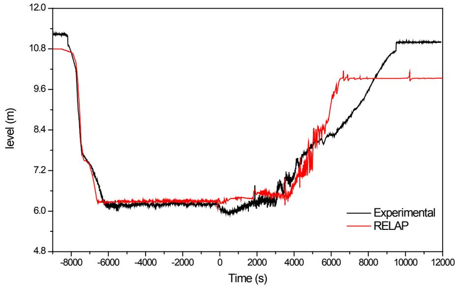
**Figure 2.5 RPV level for test F1.1 during the conditioning and the test phases**
