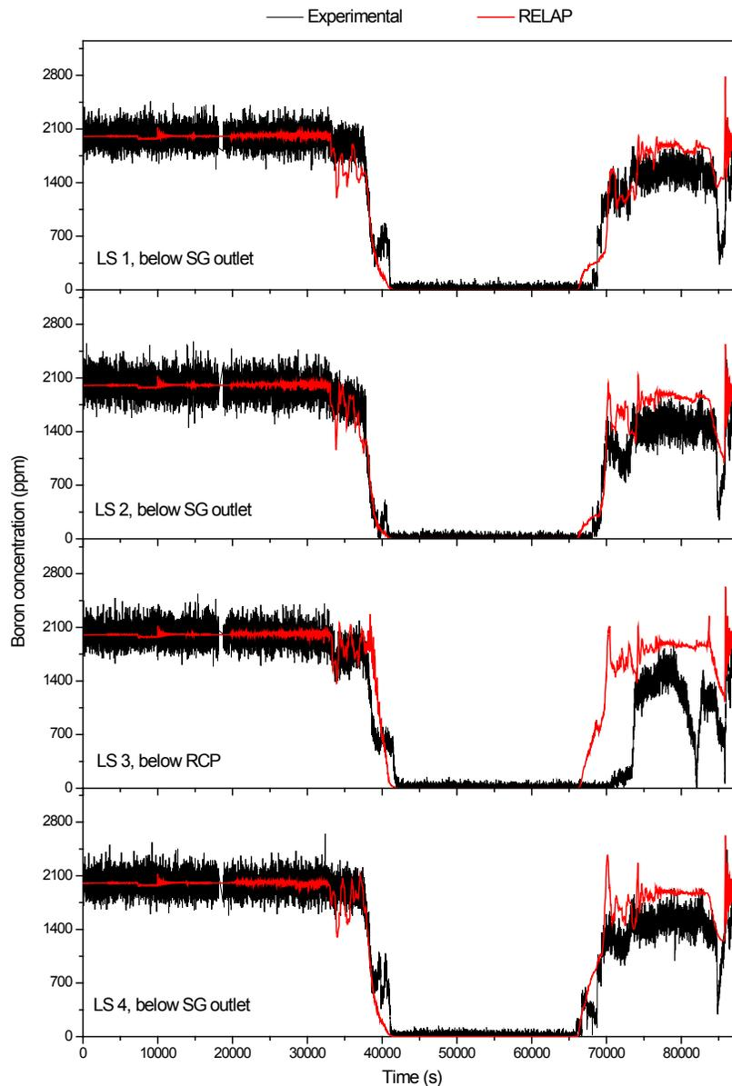
Figure 3.9 Boron concentration at each COMBO measurement for Test F1.2
