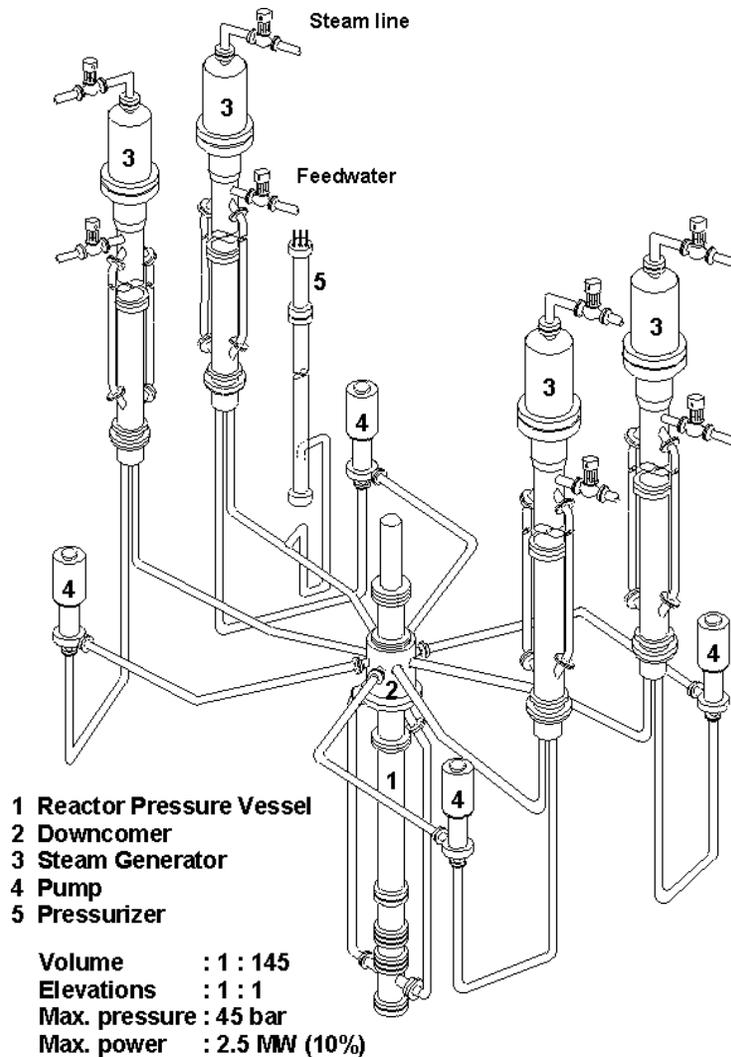
**Figure 1.1 Diagram of the PKL test facility**
