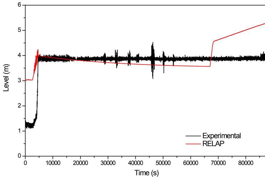
**Figure 3.2 Pressurizer collapsed water level for Test F1.1**
