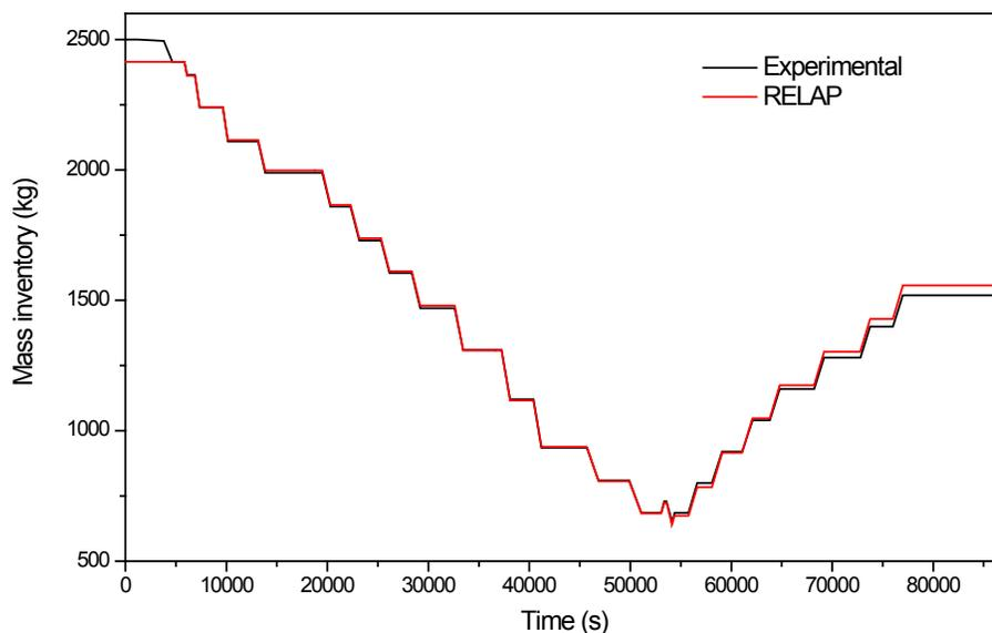
**Figure 3.4 Primary mass inventory for Test F1.2**
