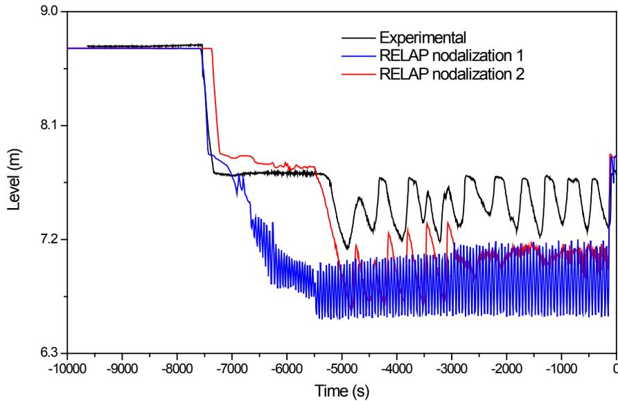
**Figure 4.2 Downcomer Collapsed water level during the conditioning phase of Test F1.1, upper head bypass sensitivity**
