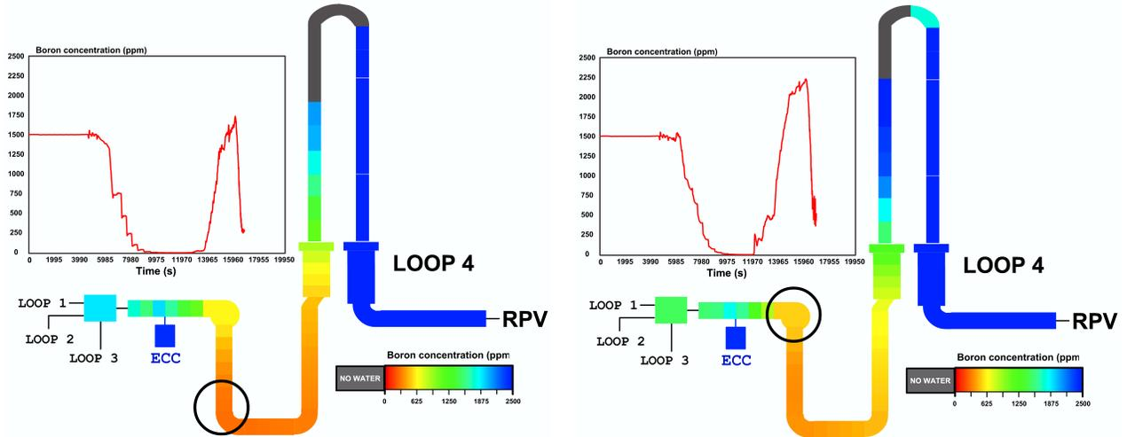
**Figure 2.14** Post test calculation of test F1.1, evolution of boron concentration in loop 4. Left and right: intermittent forward and backward movements of the slug.
