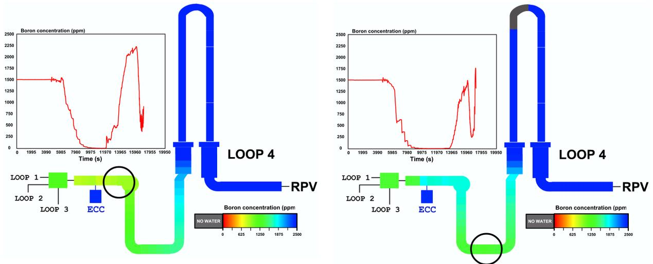
**Figure 2.16 Post test calculation of test F1.1, evolution of boron concentration in loop 4. Left and right: establishment of natural circulation.**
