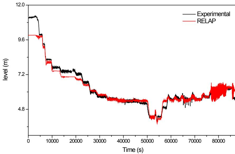
**Figure 3.6 RPV collapsed water level for Test F1.2**
