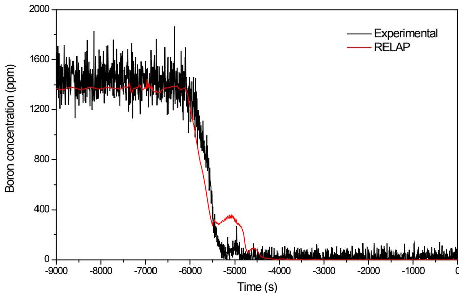
**Figure 2.3 Boron concentration in the loop seal of loop 4, conditioning phase**
