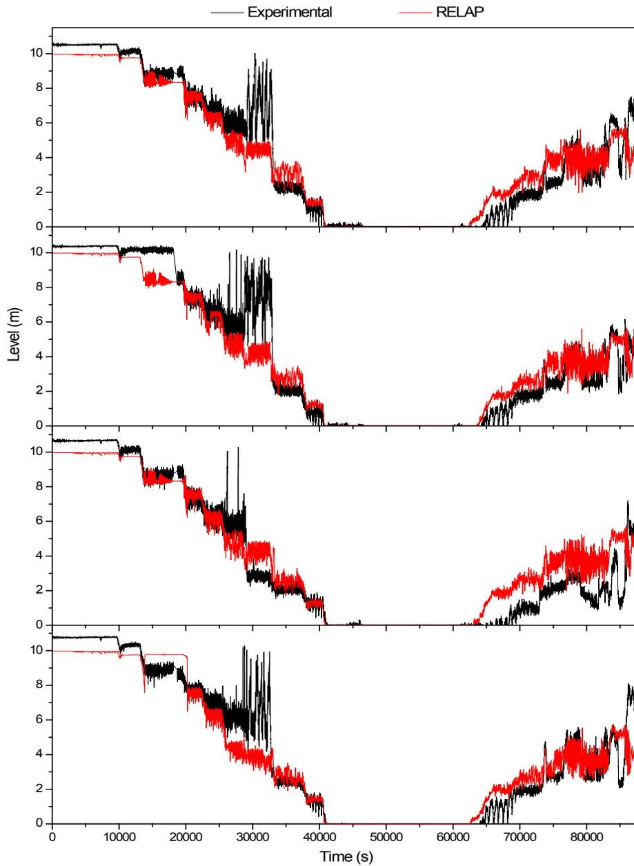
**Figure 3.8 U-tube collapsed water levels of loops 1 to 4 for Test F1.2**
