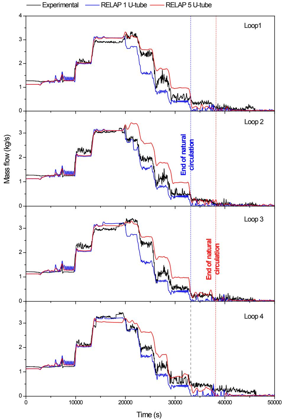
**Figure 4.6 Loop mass flows for Test F1.2 with 1 and 5 U-tubes**
