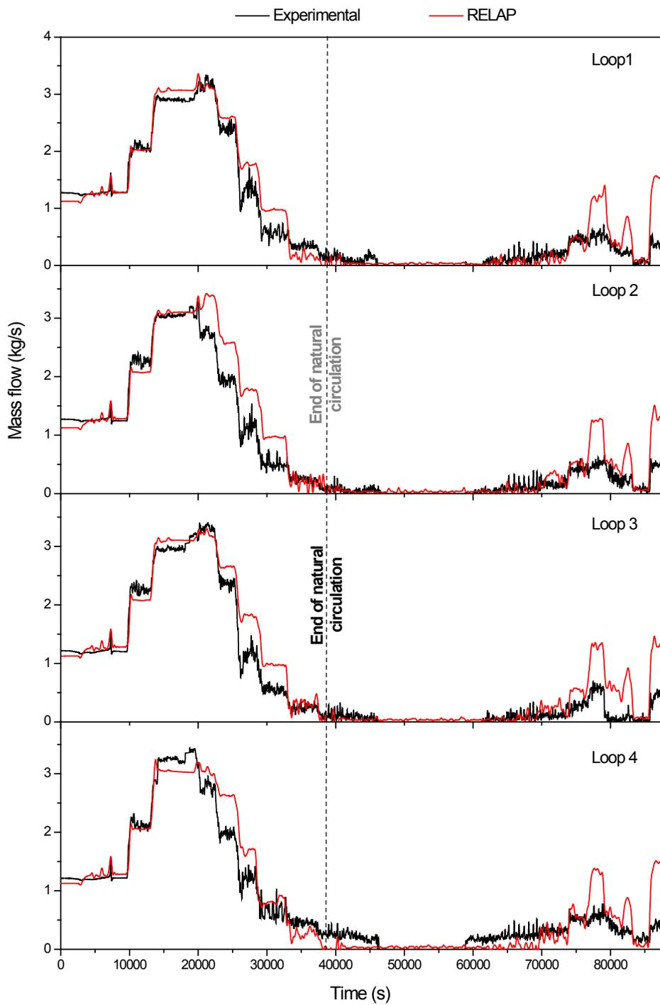
Figure 3.7 Mass flow of loops 1 to 4 for Test F1.2
