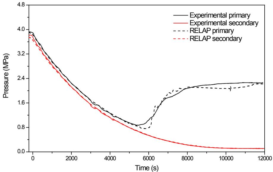
**Figure 2.4 Primary and secondary pressures for test F1.1**
