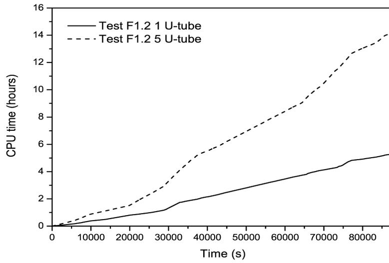
**Figure 6.2 CPU time usage for Test F1.2 using 1 and 5 pipes to simulate the U-tube bundle**
