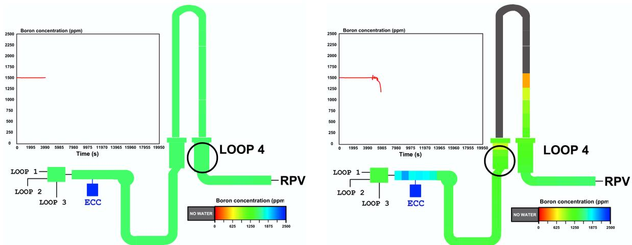
**Figure 2.10 Post test calculation of test F1.1, evolution of boron concentration in loop 4. Left: start of transient. Right: reflux-condenser conditions established**
