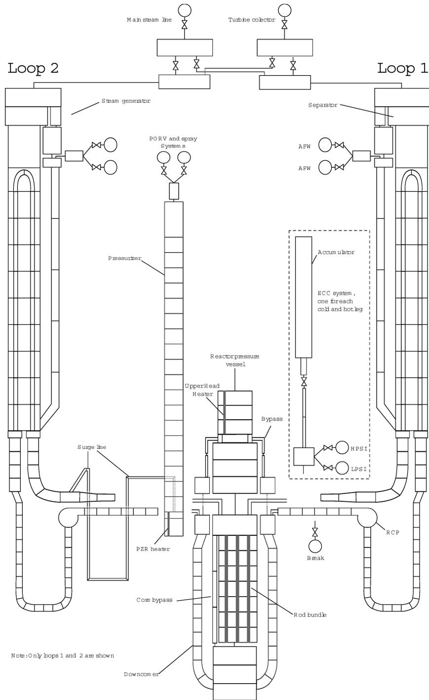
**Figure 1.2 RELAP5 nodalization for the PKL test facility. Only loops 1 and 2 are shown.**
