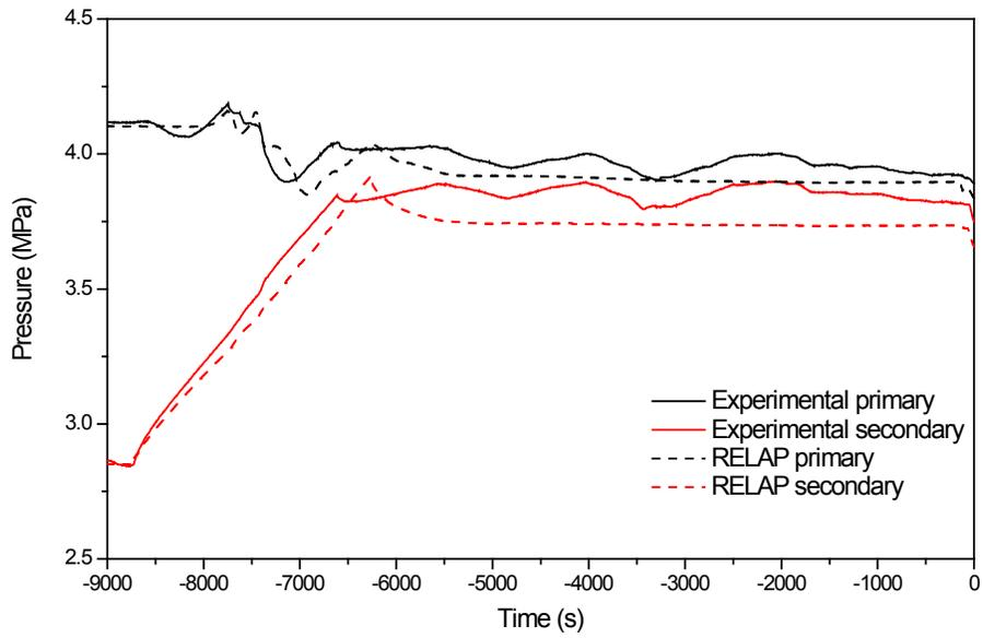
**Figure 2.1 Primary and secondary pressures, conditioning phase of test F1.1**
