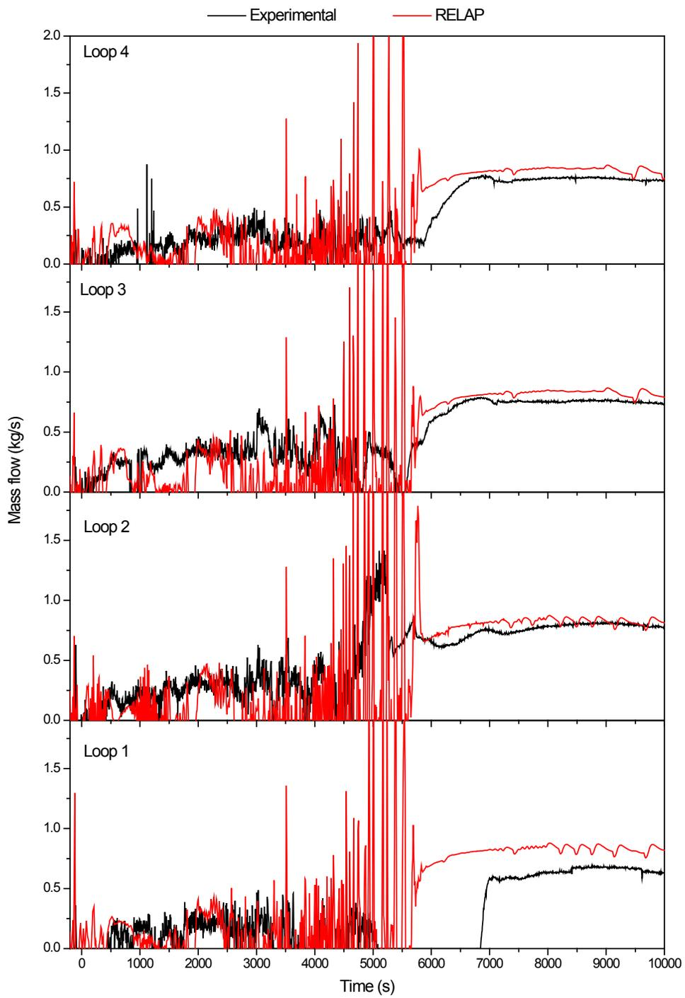
**Figure 2.8 Mass flow in all loops for test F1.1**
