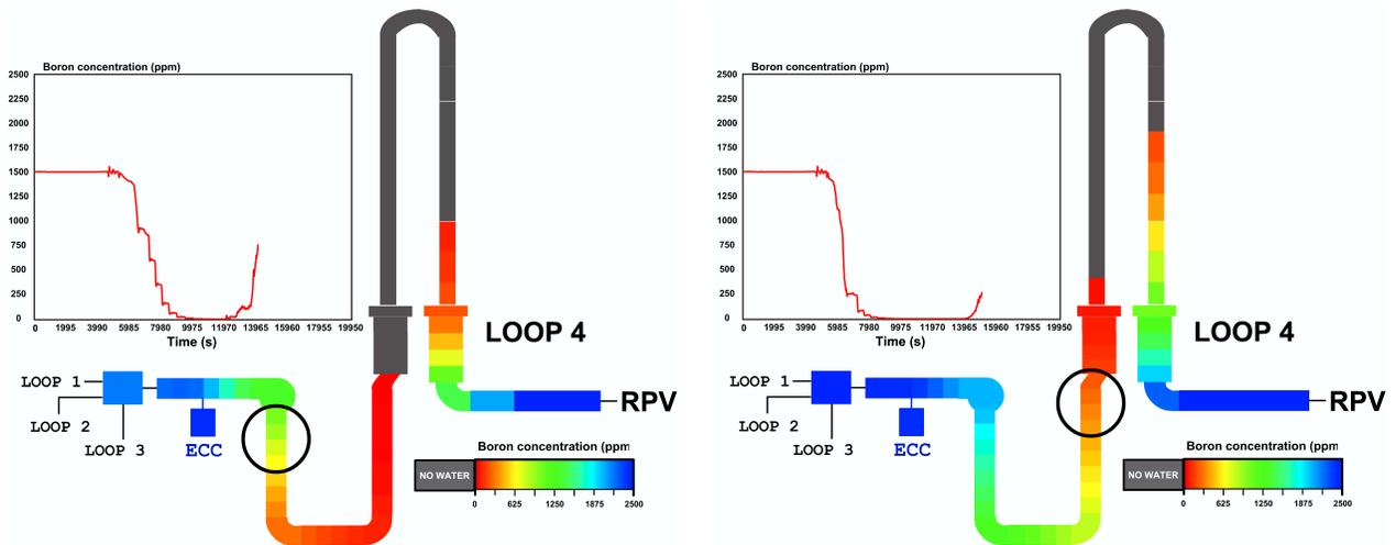
**Figure 2.12 Post test calculation of test F1.1, evolution of boron concentration in loop 4. Left: ECC flows to LS. Right: upward displacement of the slug**
