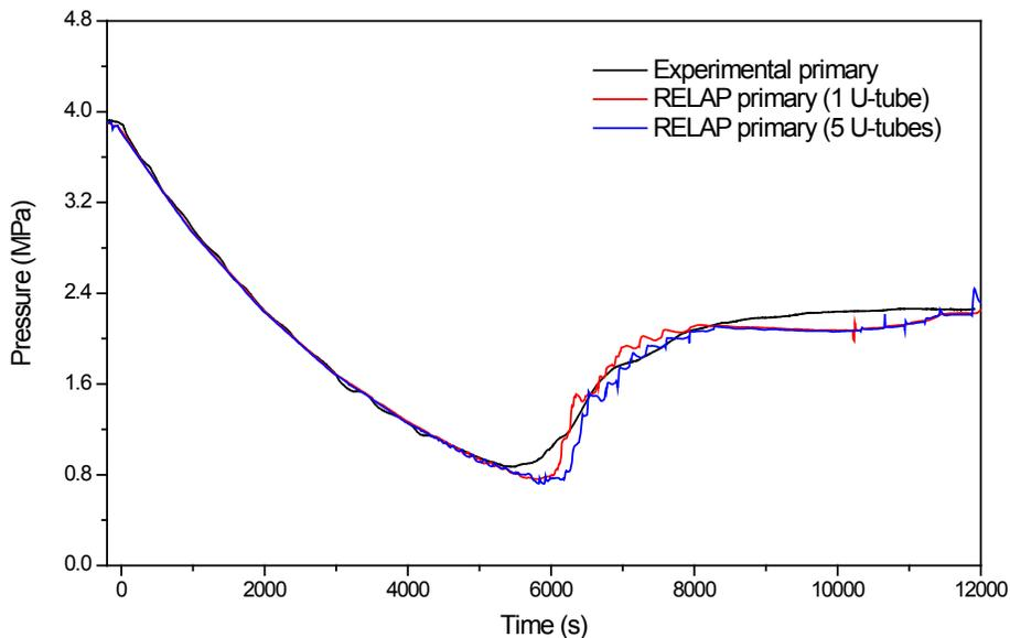
**Figure 4.4 Primary pressure for Test F1.1 with 1 and 5 U-tube elevations**
