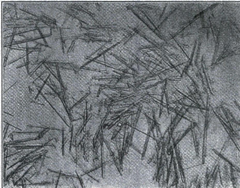
FIGURE 7.—*Synthetic wollastonite.*
