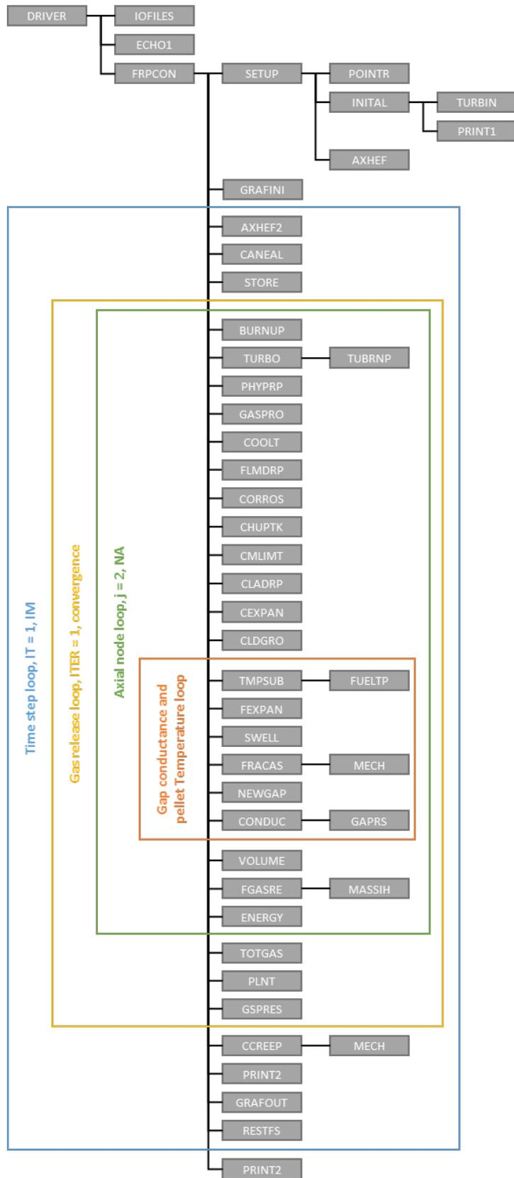
**Figure 3.2** Calling sequence for FRAPCON-3 subroutines
