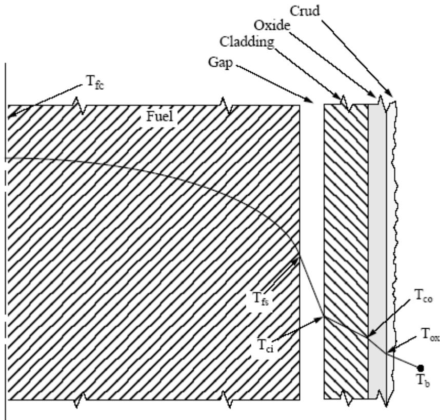
**Figure 2.3** Schematic of the fuel rod temperature distribution
