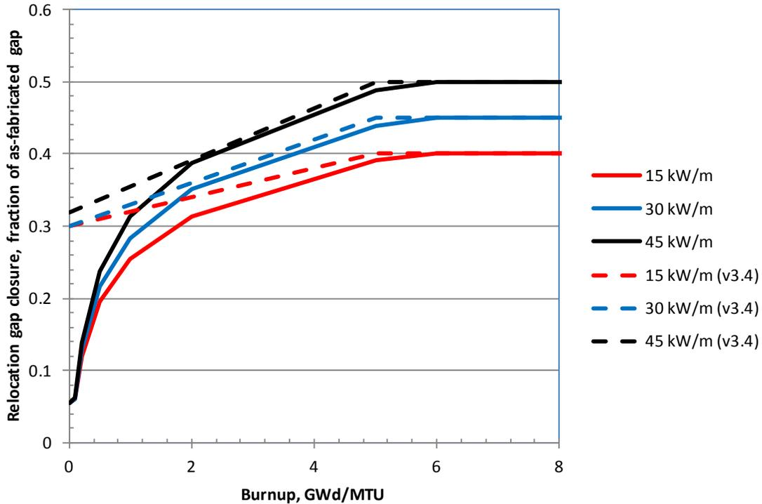
**Figure 2.16** Power and burnup dependence of the FRAPCON-3.5 relocation model with the old relocation model (v3.4) shown for reference.
