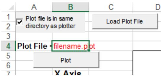
2. If the plot file is in a different folder from the plotter, make sure the 'Plot file is in same directory as plotter' box is unchecked, and type the file name including its path in cell B4, then press enter and click 'Load Plot File'.
