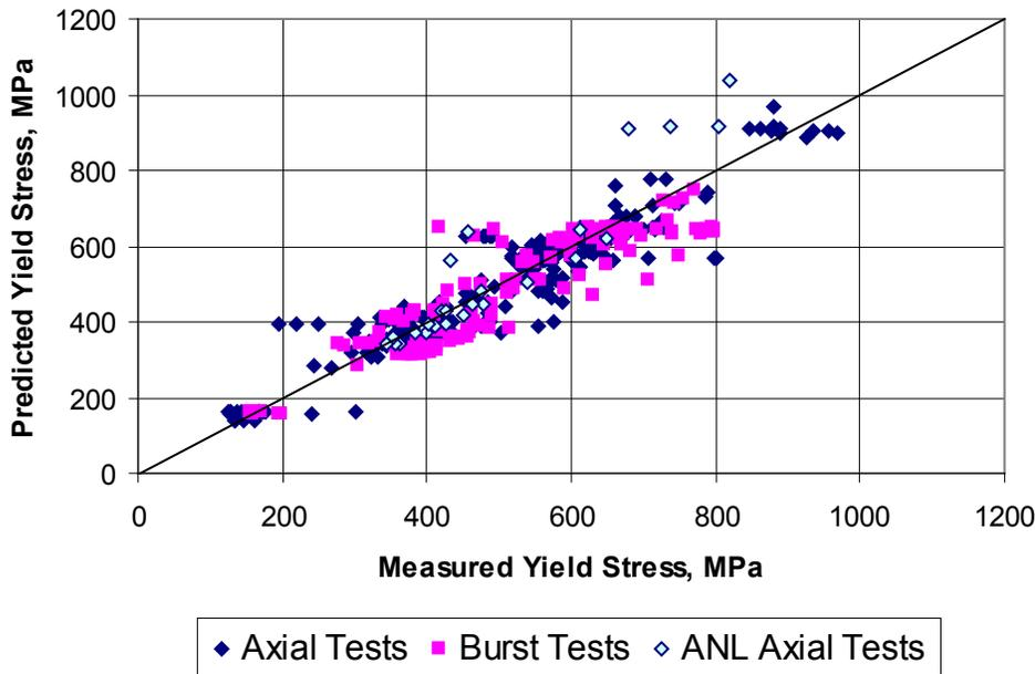
**Figure 2.14** Predicted vs. measured yield stress from the PNNL database ( $293\text{K} \leq T \leq 755\text{K}$ ),  $0 \leq \Phi \leq 14 \times 10^{25} \text{ n/m}^2$ ,  $0 \leq H_{\text{ex}} \leq 850 \text{ ppm}$
