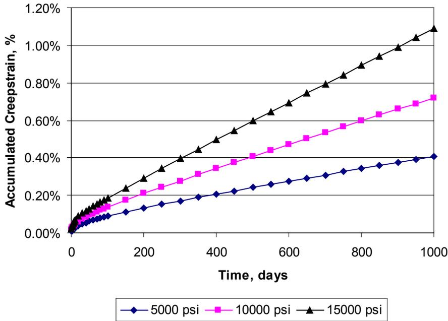
**Figure 2.9** Cladding creep strain as a function of time and hoop stress for 630°F and flux= $10^{18}$  n/m<sup>2</sup>/s for (a) SRA Zircaloy and (b) RZA Zircaloy
