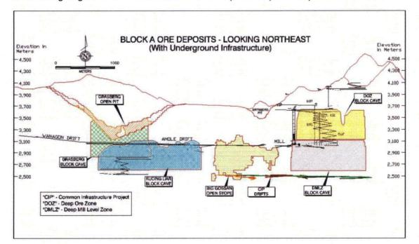
The following diagram indicates the relative elevations (in meters) of our reported ore bodies.
