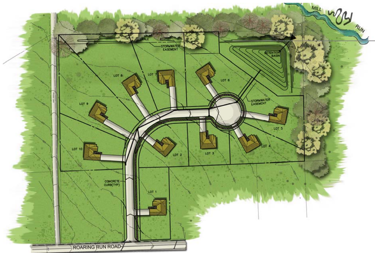
Figure 8.3. Traditional Subdivision Layout (Designed for Peak Rate Control)
