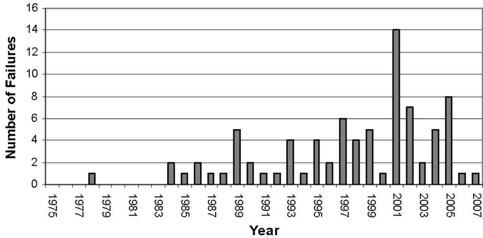
Figure 3.1. Cables that failed while in service. Source: GL 2007-01 Summary Report (Figure 2) [1].
