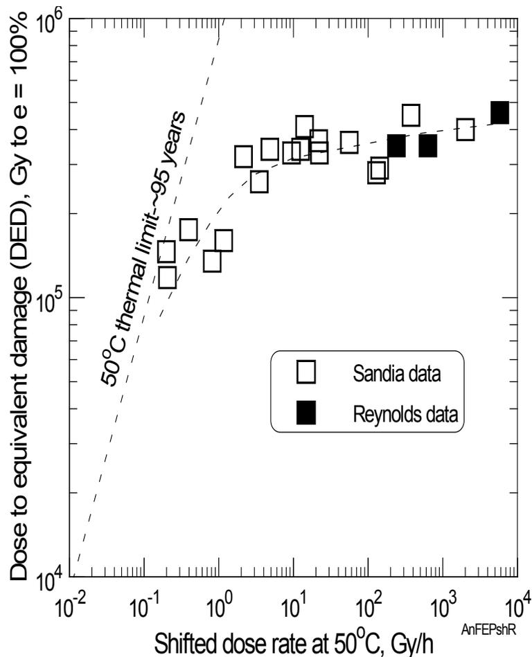
**Figure 5.14. Time-temperature-dose rate superposition at 50 °C (122 °F) for Anaconda Flameguard EPR insulation (limited crystallinity) for the dose required to reach 100% elongation under combined radiation/thermal environments [90].**
