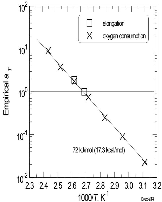
**Figure 5.15. Arrhenius plot of the shift factors for elongation and oxygen consumption for Brandrex CLPO insulation [75, 90].**
