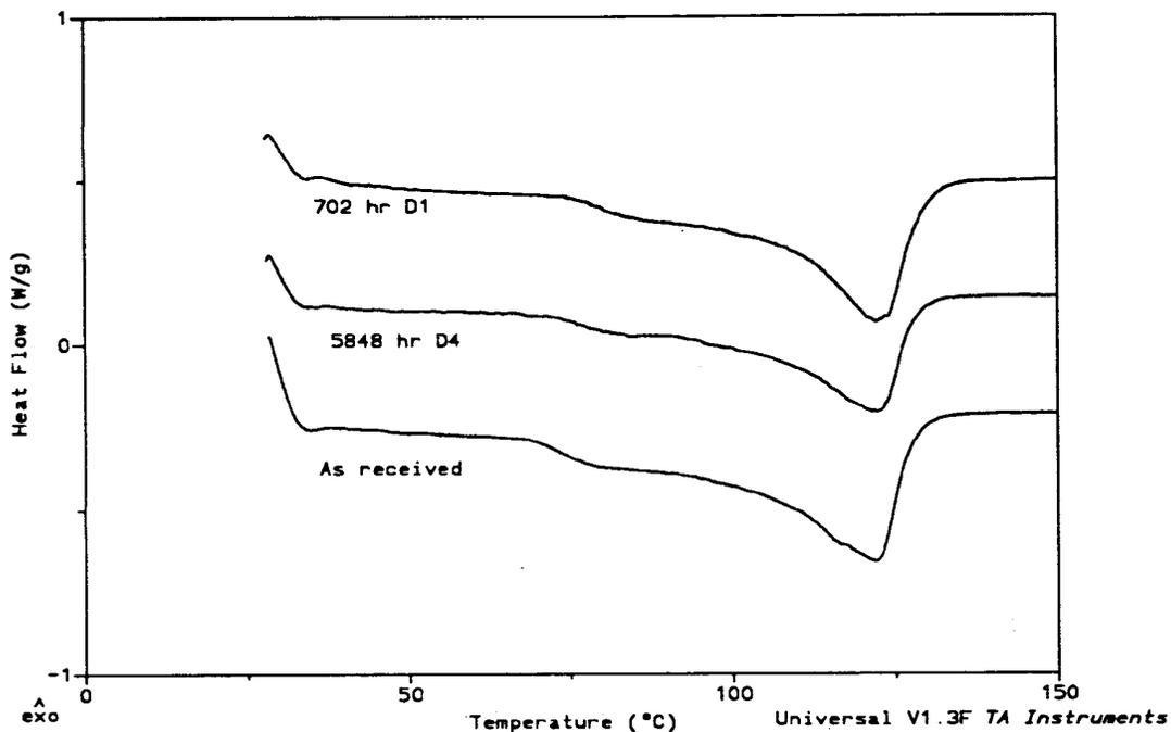
**Figure 5.16. DSC traces for a XLPE insulation material, showing the crystalline melting endotherm in both unaged and aged material [31].**
