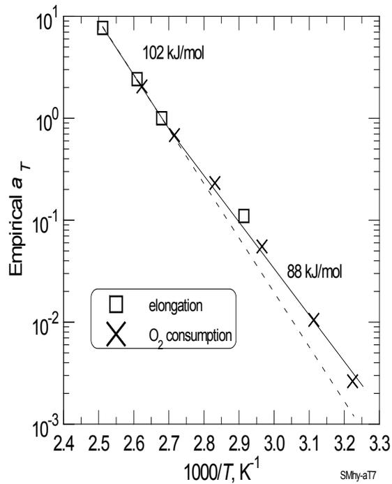
**Figure 5.3. Arrhenius plot for the shift factors for elongation at break and oxygen consumption data for the Samuel Moore Dekoron CSPE jacket material [75].**
