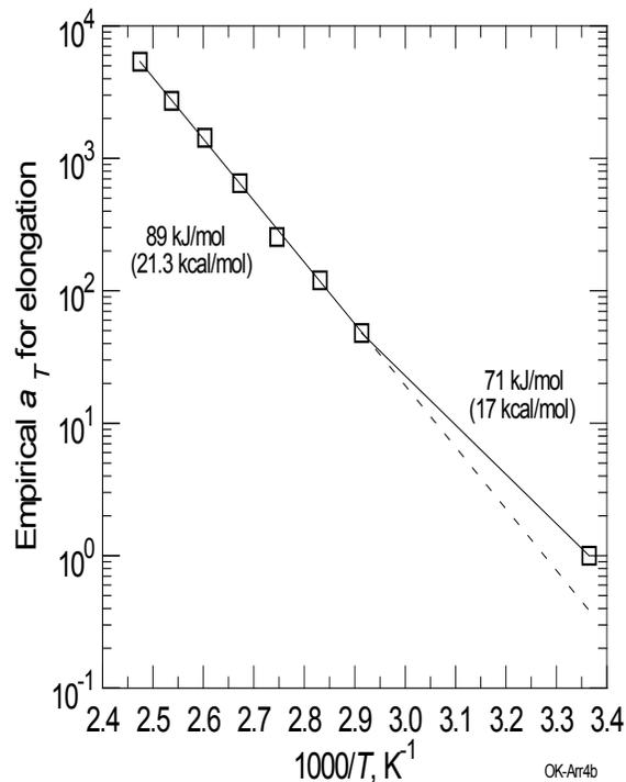
**Figure 5.1. Arrhenius plot for the shift factors for elongation at break aging data for the Okonite neoprene jacket material [75].**
