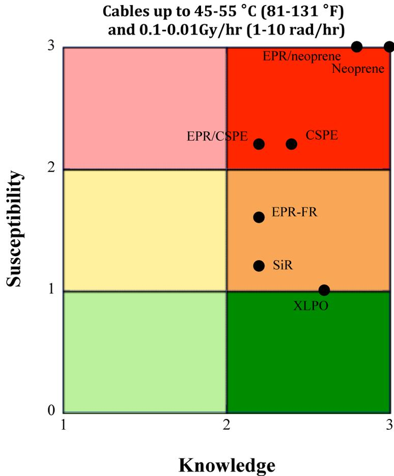
Figure A.4. Susceptibility-Knowledge plot for cables at 45–55 °C (81–131 °F) and 0.1–0.01 Gy/hr (1–10 rad/hr) (inside containment).
