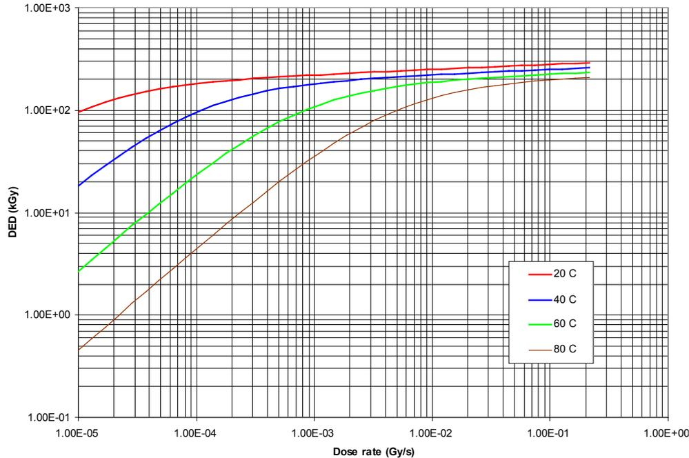
**Figure 5.11. Generic shapes of the dose required to reach a specific level of degradation (dose-equivalent damage) as a function of dose rate at different temperatures for a typical polymeric cable material [75, 91].**
