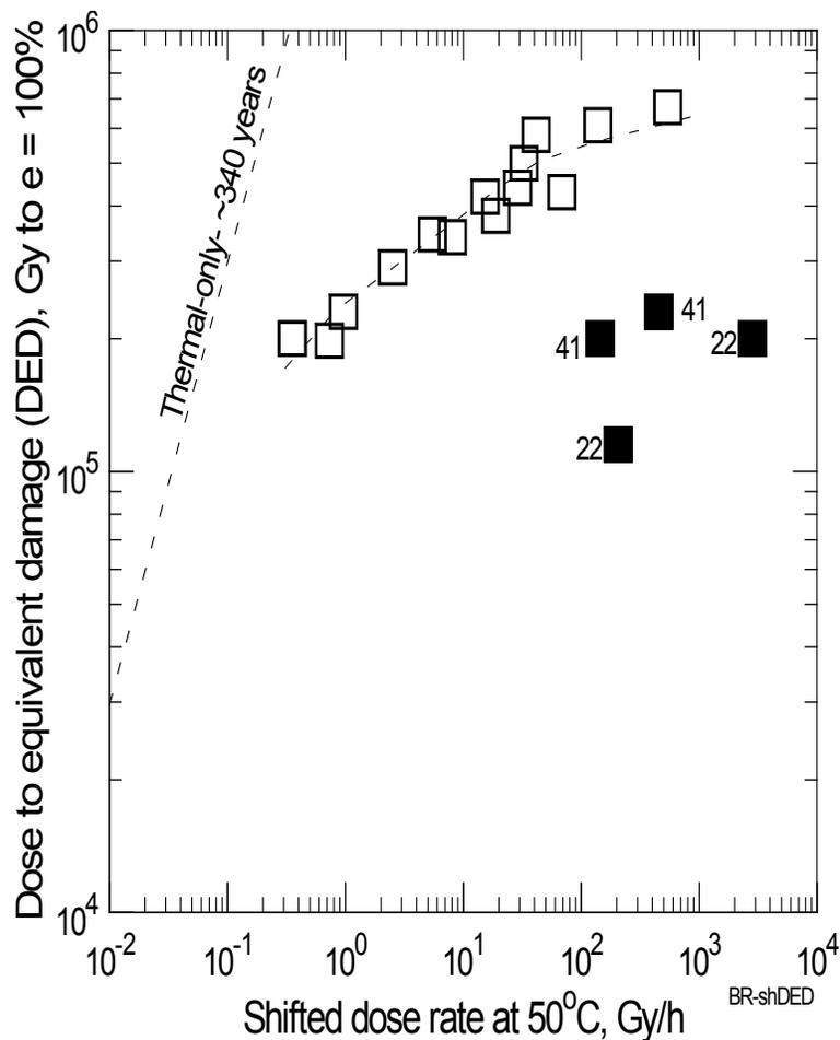
**Figure 5.12. Time-temperature-dose rate superposition at 50 °C (122 °F) for Brandrex CLPO insulation for the dose required to reach 100% elongation under combined radiation/thermal environments. The numbers by the filled squares denote the aging temperatures in °C [90].**
