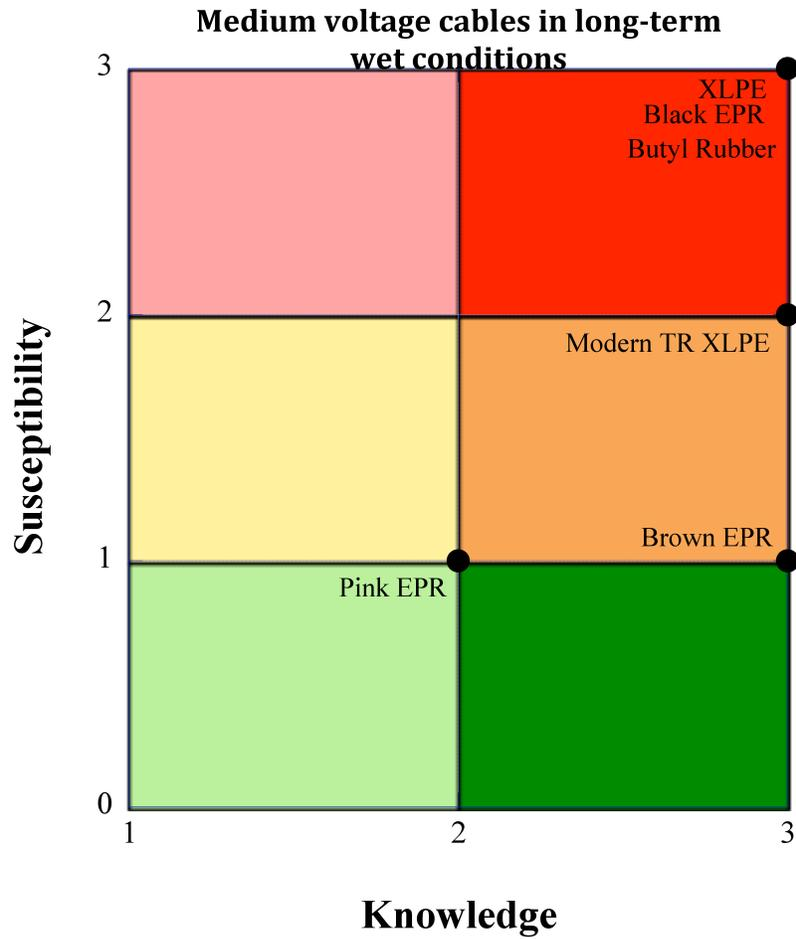
**Figure A.7. Susceptibility–Knowledge plot for medium-voltage cables in long-term wet conditions.**
