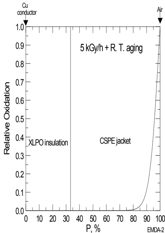
**Figure 5.7. Estimated oxidation profile [69] across a “generic” 3/C cable with a 60-mil-thick CSPE jacket and 30-mil-thick XLPO insulations aged at room temperature and 5 kGy/h.**
