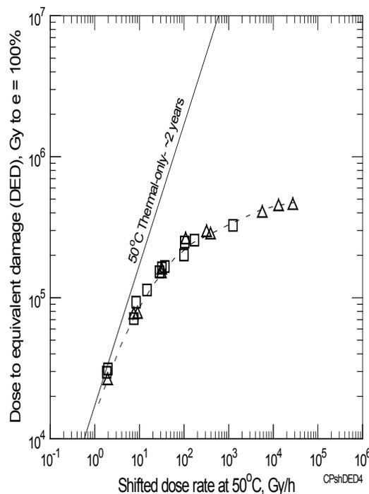
**Figure 5.8. Time-temperature-dose rate superposition at  $50\text{ }^{\circ}\text{C}$  ( $122\text{ }^{\circ}\text{F}$ ) for the Okonite neoprene for the dose required to reach 100% elongation under combined radiation/thermal environments [90]. The homogeneously aged results are plotted as squares whereas the non-homogeneous (DLO-affected) are plotted as triangles.**
