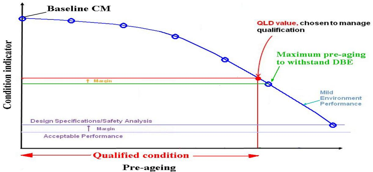
Figure 6.1. Schematic representation of the concept of condition-based qualification [31].
