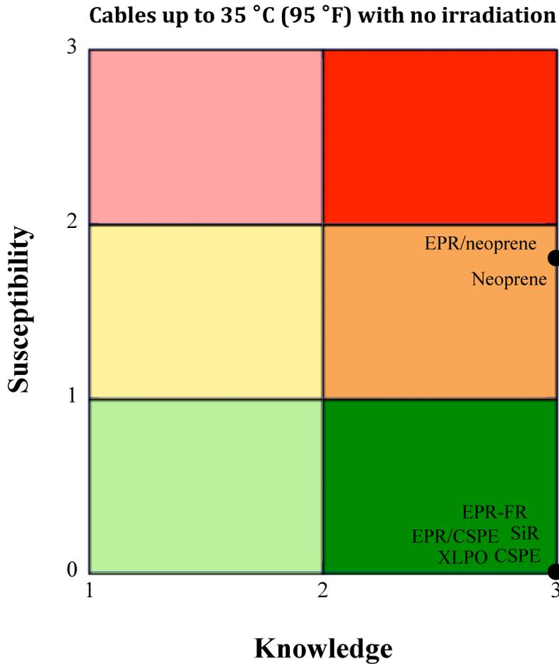
Figure A.2. Susceptibility–Knowledge plot for cables at up to 35 °C (95 °F) with no irradiation.
