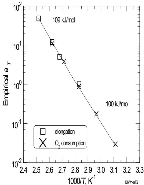
**Figure 5.4. Arrhenius plot for the shift factors for elongation at break and oxygen consumption data for the BIW Bostrad 7E CSPE jacket material [75].**
