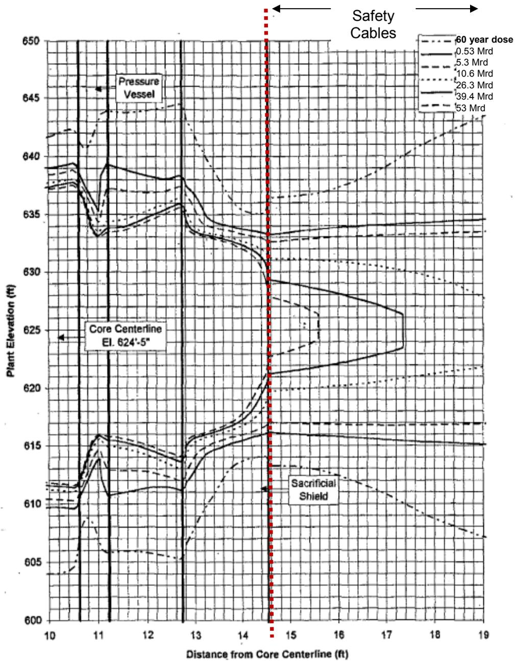
Figure 7.1. BWR IV Mark 1 containment gamma dose (rad carbon) unpenetrated sacrificial shield.
