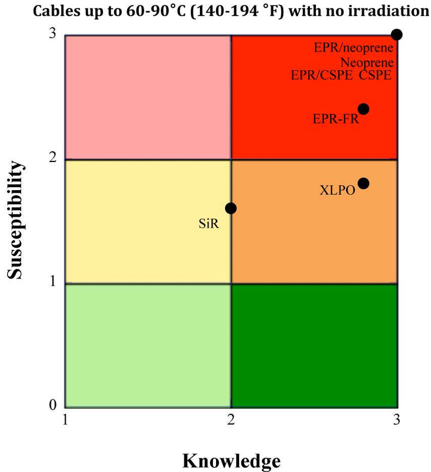
**Figure A.6. Susceptibility-Knowledge plot for cables at 60–90 °C (140–194 °F) with no irradiation.**
