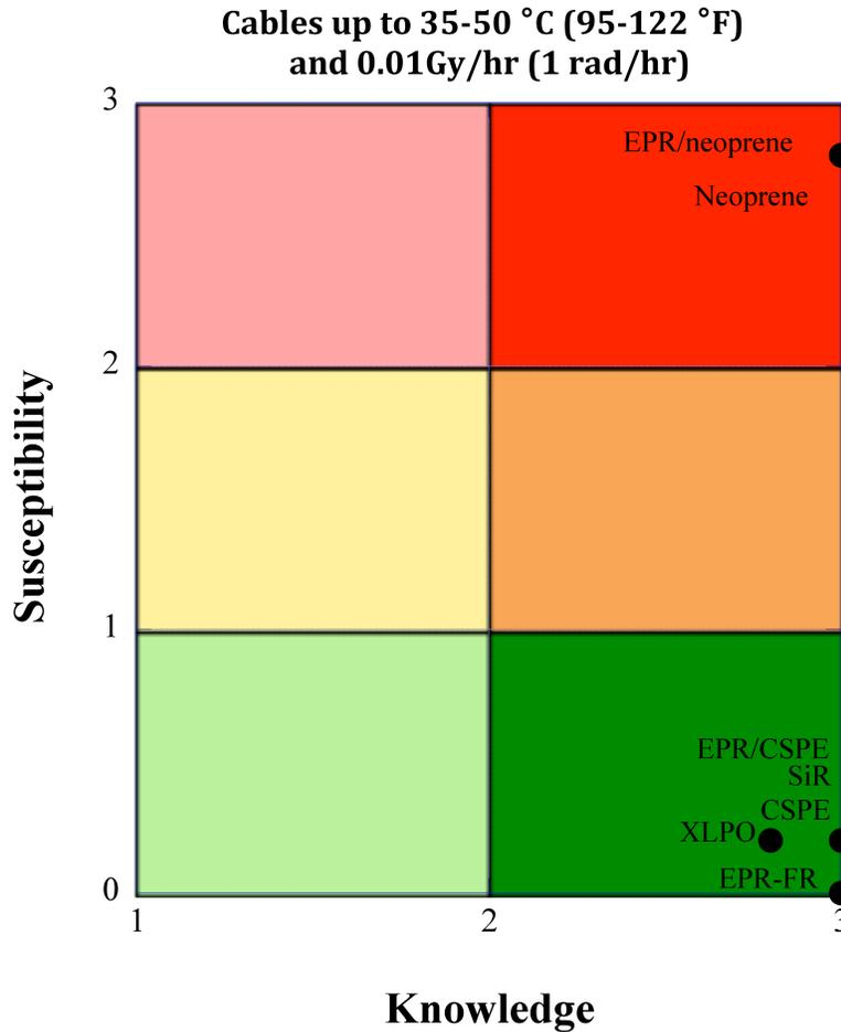
Figure A.3. Susceptibility–Knowledge plot for cables at 35–50 °C (95–122 °F) and up to 0.01Gy/hr (1 rad/hr).
