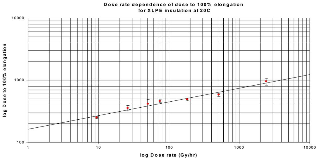
**Figure 5.10. Dose in kGy required to reach 100% elongation for a XLPE cable insulation material at 20 °C (68 °F) [90].**
