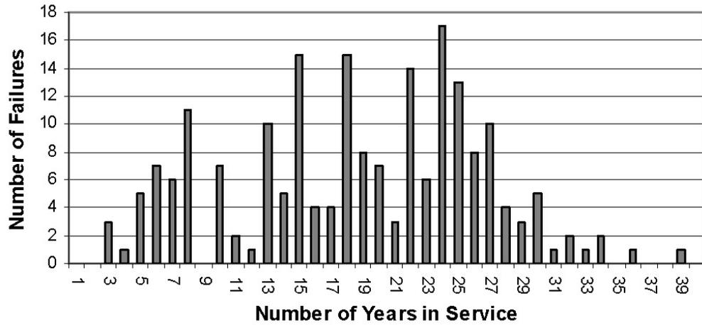
Figure 3.2. Failures per cable age (years in service). Source: GL 2007-01 Summary Report (Figure 4) [1].
