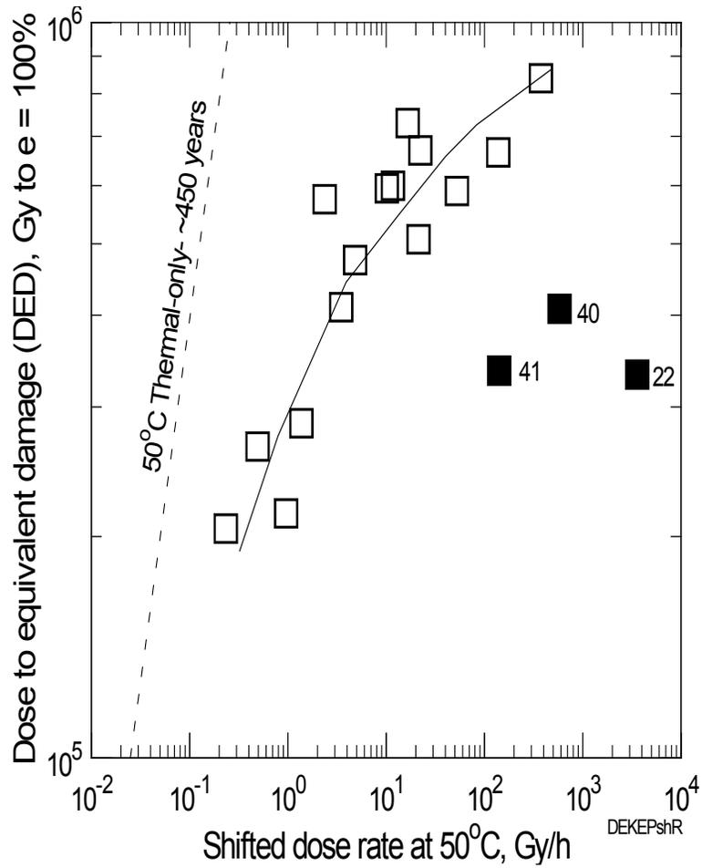
Figure 5.13. Time-temperature-dose rate superposition at 50 °C (122 °F) for Eaton Dekoron Elastoset EPR insulation (significant crystallinity) for the dose required to reach 100% elongation under combined radiation/thermal environments. The numbers by the filled squares denote the aging temperatures in °C [90].
