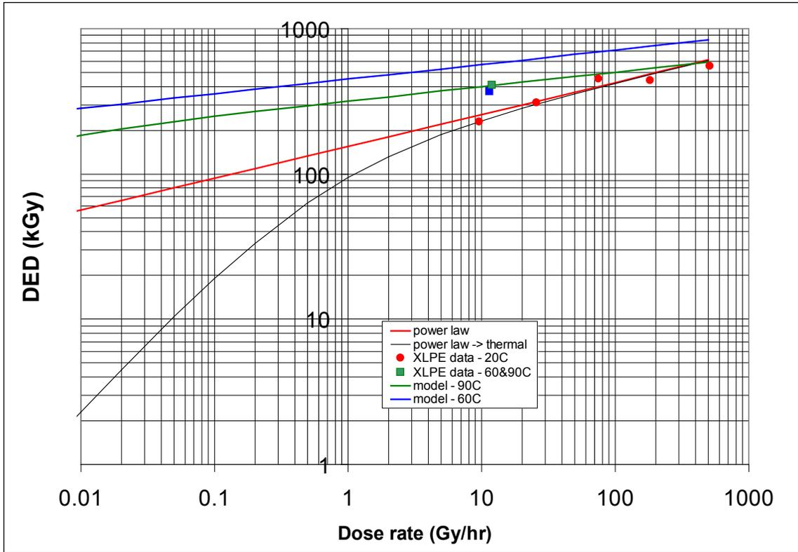
**Figure 5.17. Radiation aging data for a XLPE insulation material as a function of dose rate [31].**
