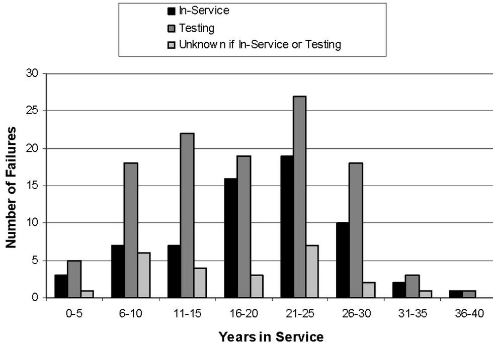
**Figure 3.4. Failures per five-year service intervals (in service, testing, unknown). Source: GL 2007-01 Summary Report (Figure 6) [1].**
