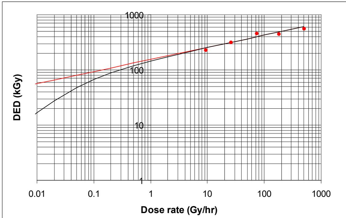
Figure 5.18. An illustration of how the degradation curve for this XLPE might behave at lower dose rates (black line), compared to the power law model (red line) [31].
