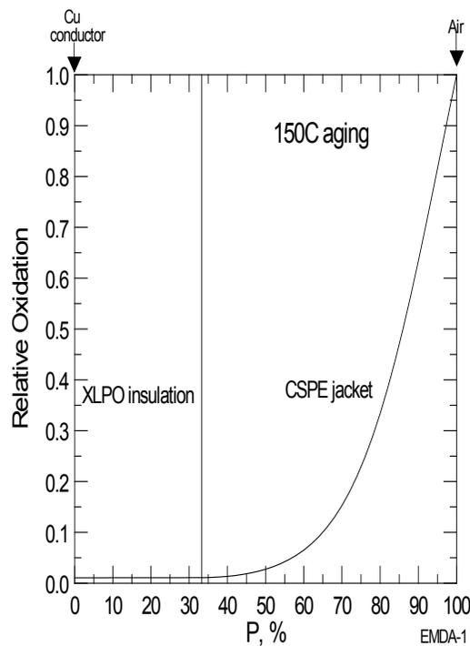
**Figure 5.6. Estimated oxidation profile [78] across a “generic” 3/C cable with a 60-mil-thick CSPE jacket and 30-mil-thick XLPO insulations aged at typical 150 °C (302 °F).**
