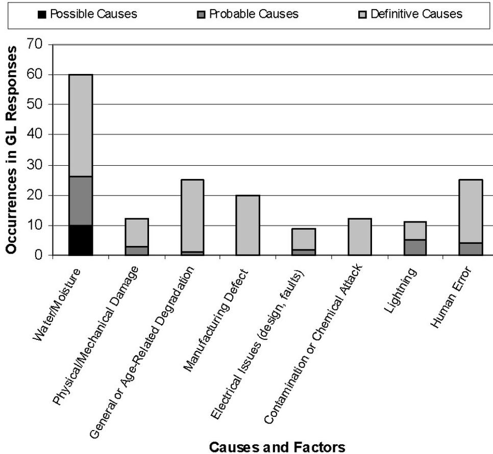
Figure 3.5. Causes and causal factors for all cable failures. Source: GL 2007-01 Summary Report (Figure 22) [1].
