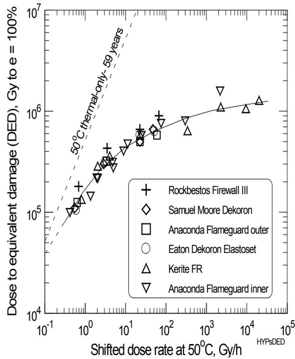
**Figure 5.9. Time-temperature-dose rate superposition at 50 °C (122 °F) for several CSPE materials for the dose required to reach 100% elongation under combined radiation/thermal environments [90].**
