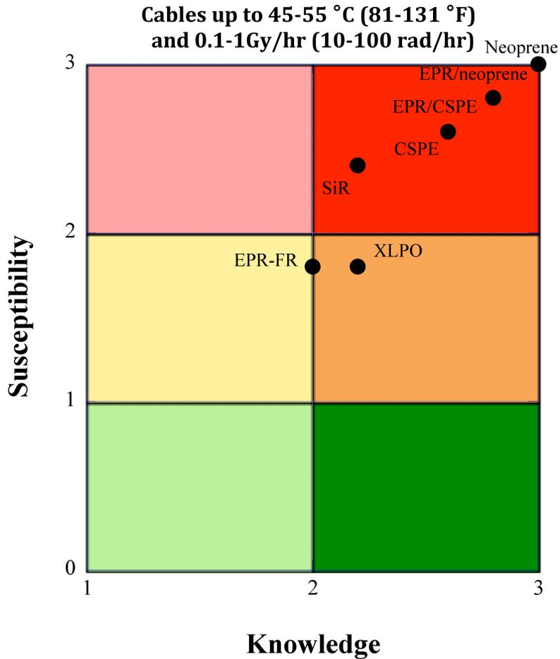
Figure A.5. Susceptibility–Knowledge plot for cables at 45–55 °C (81–131 °F) and 0.1 to 1 Gy/hr (10–100 rad/hr) (inside containment).
