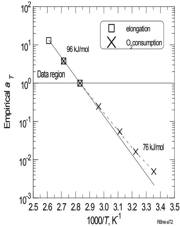
**Figure 5.2. Arrhenius plot for the shift factors for elongation at break and oxygen consumption data for the Rockbestos Firewall III neoprene jacket material [75].**
