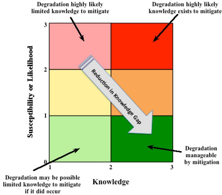
Figure A.1. Schematic illustrating the combinations of Susceptibility and Knowledge scores suggesting various life management responses.
