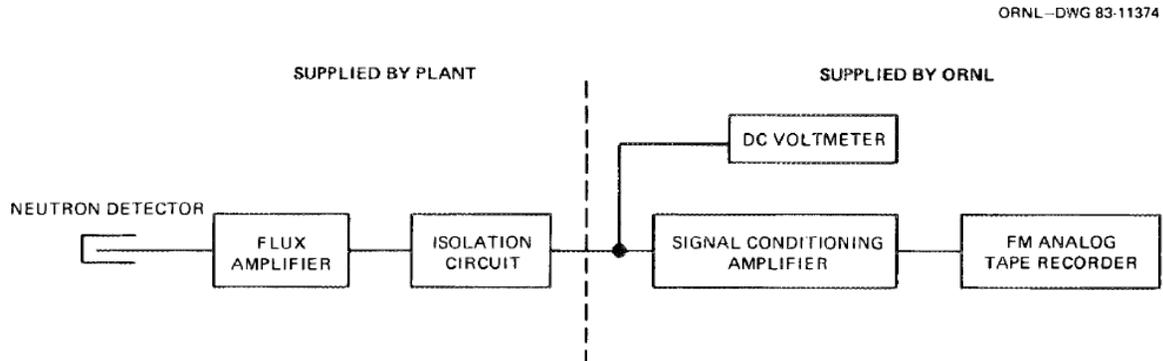
**FIGURE 4-8 DATA ACQUISITION FOR NEUTRON NOISE MEASUREMENT (FRY, ET AL., 1984)**
