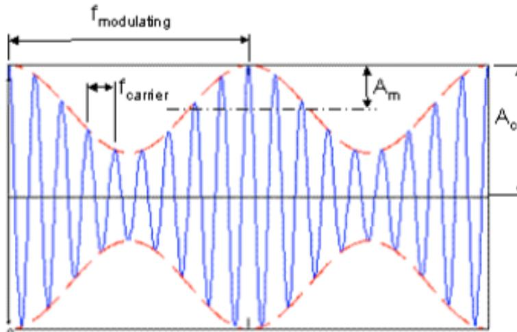
**FIGURE 4-4 AMPLITUDE MODULATED SIGNAL**
