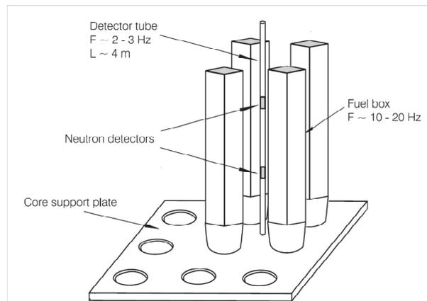
**FIGURE 4-7 DETECTOR TUBE IN A BWR CORE**
