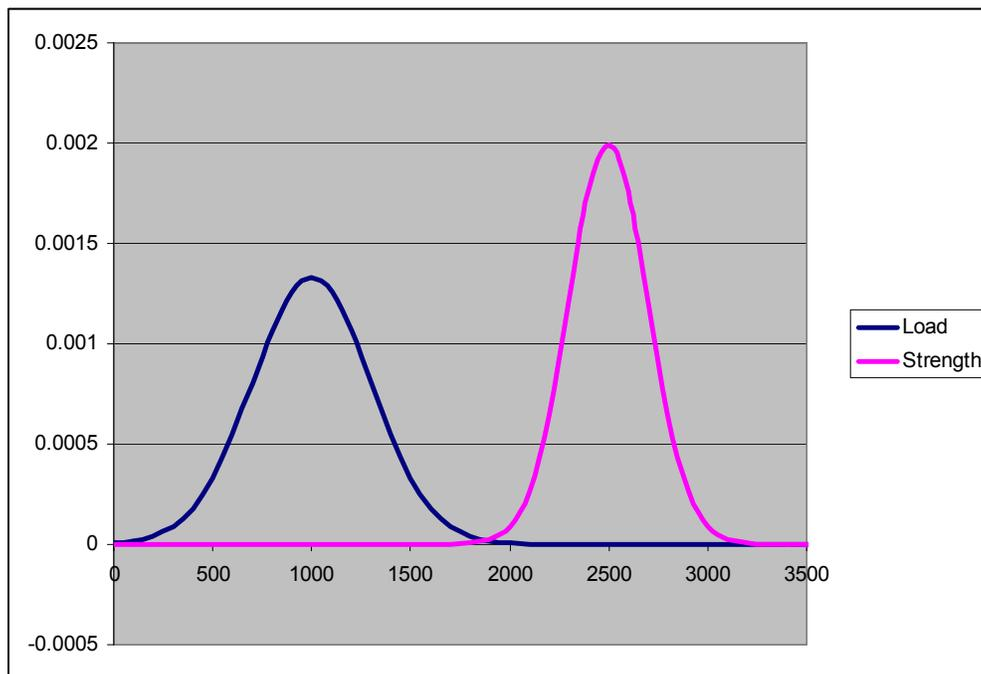
**FIGURE 2-1 PROBABILITY DENSITY OF LOAD AND STRENGTH**
