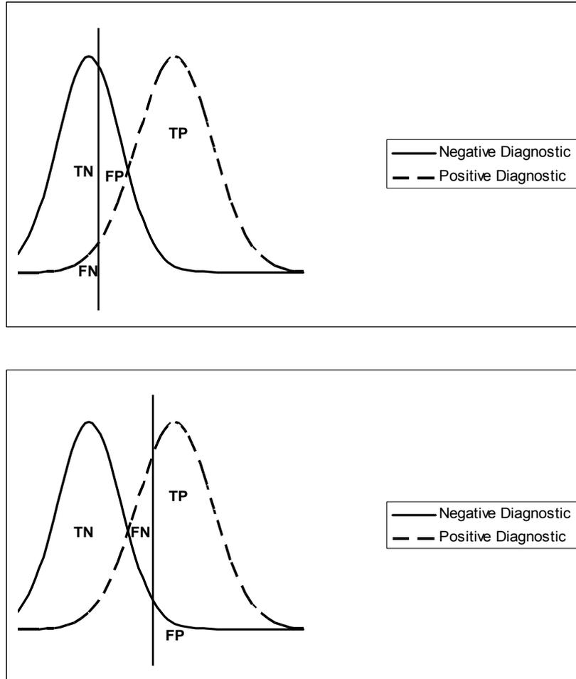
**FIGURE 5-3 DISTRIBUTIONS OF DIAGNOSTIC MEASUREMENT: (TOP) A LOW THRESHOLD WILL INCUR MORE FALSE POSITIVE (FP) RESULTS; (BOTTOM) A HIGH THRESHOLD WILL INCUR MORE FALSE NEGATIVE (FN) RESULTS.**
