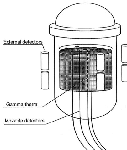
**FIGURE 4-6 EX-CORE ION CHAMBERS IN A PWR**
