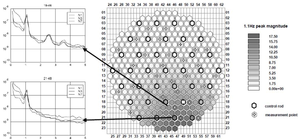
**FIGURE 4-5 NOISE MAP OF CONTROL ROD VIBRATION AT 1.1HZ (THIE, 1981)**
