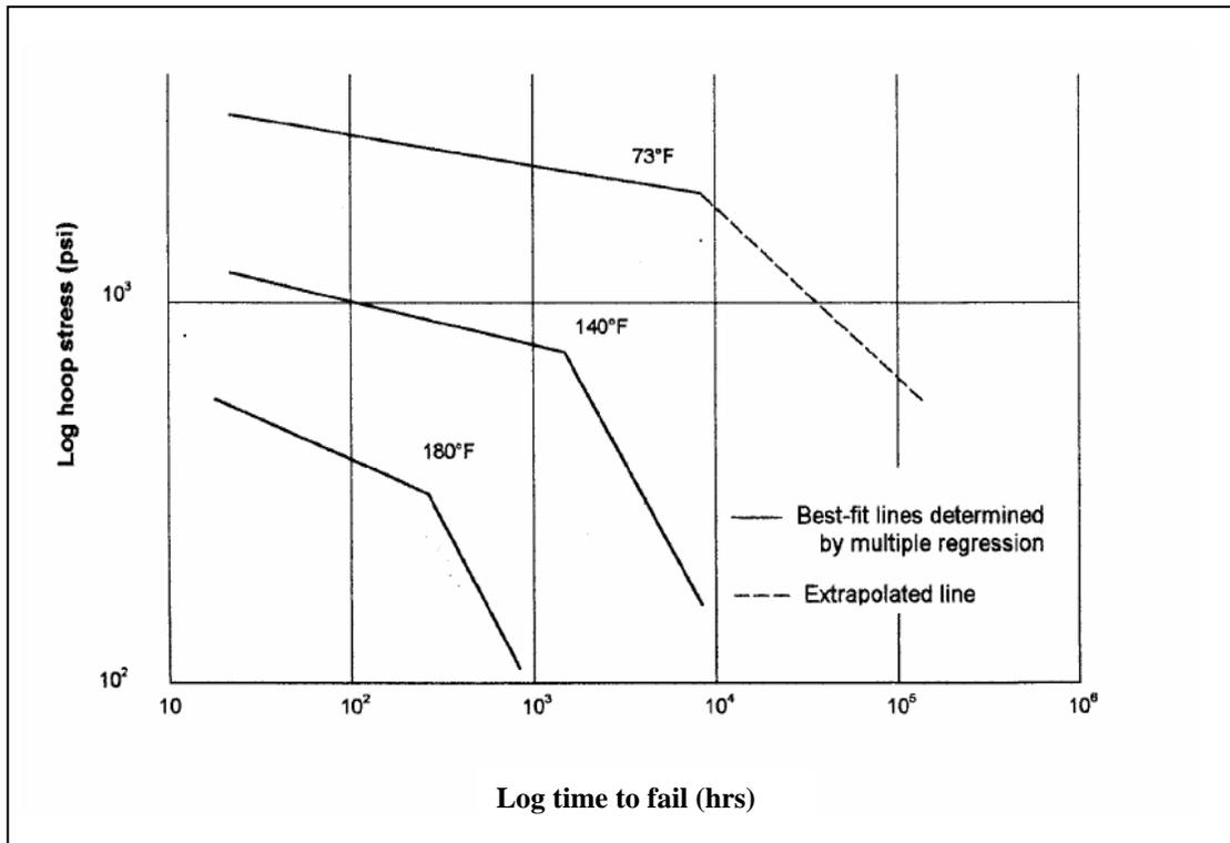
**Figure 9** Schematic of pipe stress rupture data at various temperatures shown as hoop stress versus time to failure [Ref. 16]
