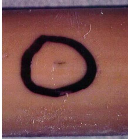
**Figure 8b** Photograph of typical “brittle” axial-slit type of failure during LTHS determination
