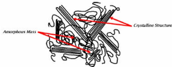
**Figure 3b Representation of the amorphous and semi-crystalline phases in PE microstructure**
