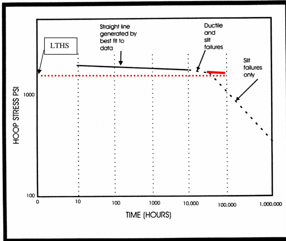
**Figure 7 Schematic of stress rupture data plot for plastic pipes tested to failure (LTHS = Long Term Hydrostatic Stress)**
