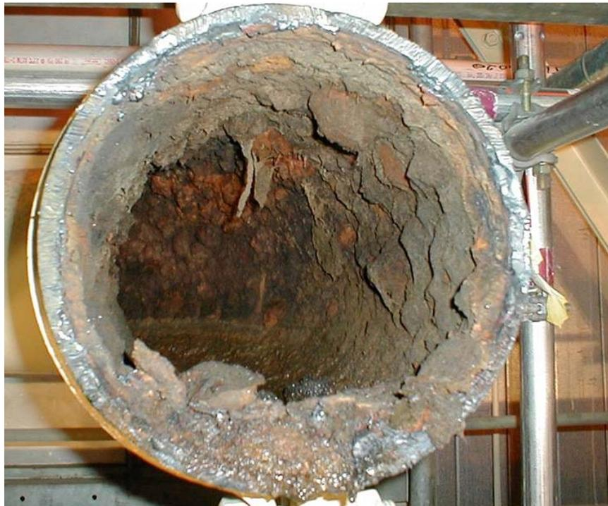
**Figure 1 Typical microbiological growth attaching to steel pipe creating flow restrictions**
