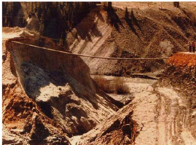
**Figure 11 Photograph of PE pipe after landslide**
