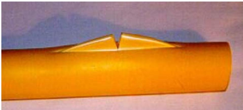
**Figure 8a Photograph of typical “ductile” failure during stress-rupture testing to determine LTHS**
