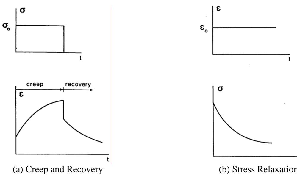
**Figure 6 Schematic of typical (a) creep-recovery under constant stress, and (b) stress relaxation under constant strain**
