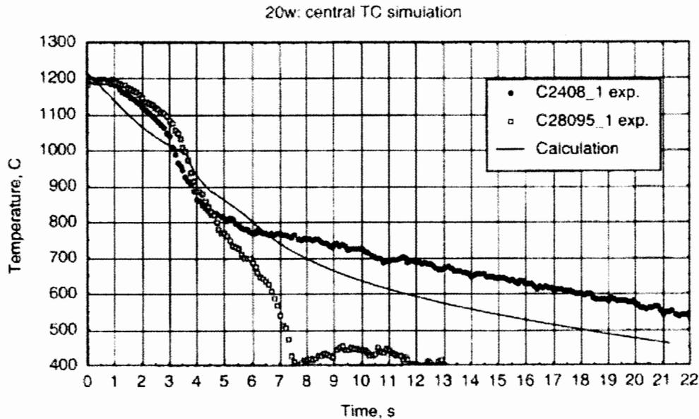
Figure 3 47: Temperature evolution of the central TC in the 20w type experiment (1200 °C, 0 μm pre-oxidation, water quenching) in the time interval 0–22 s.
