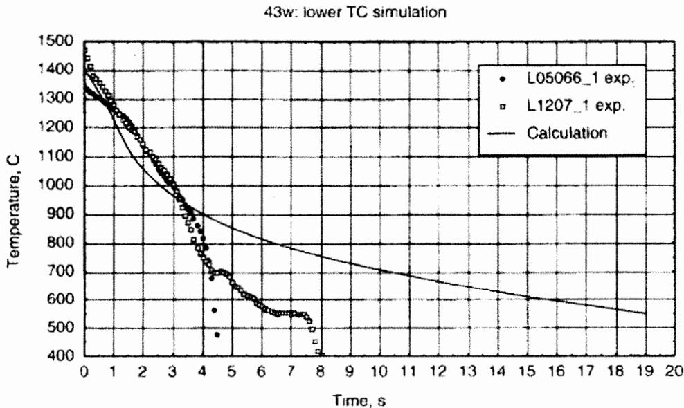
Figure 3.39: Temperature evolution of the lower TC in the 43w type experiment (1400 $^{\circ}\text{C}$ , 300  $\mu\text{m}$  pre-oxidation, water quenching) in the time interval 0-20 s.
