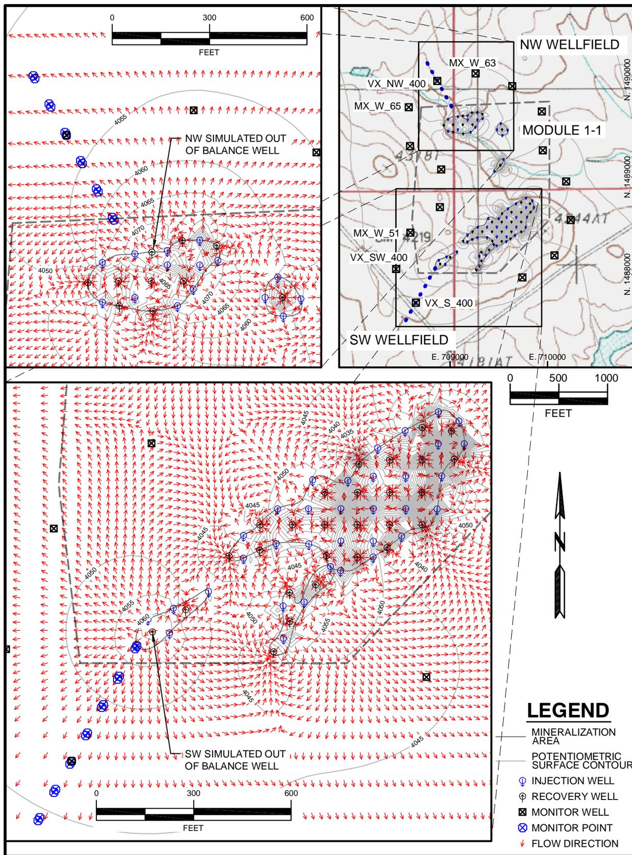
Figure 4.11-5. Groundwater Flow During Excursion in Module 1-1
