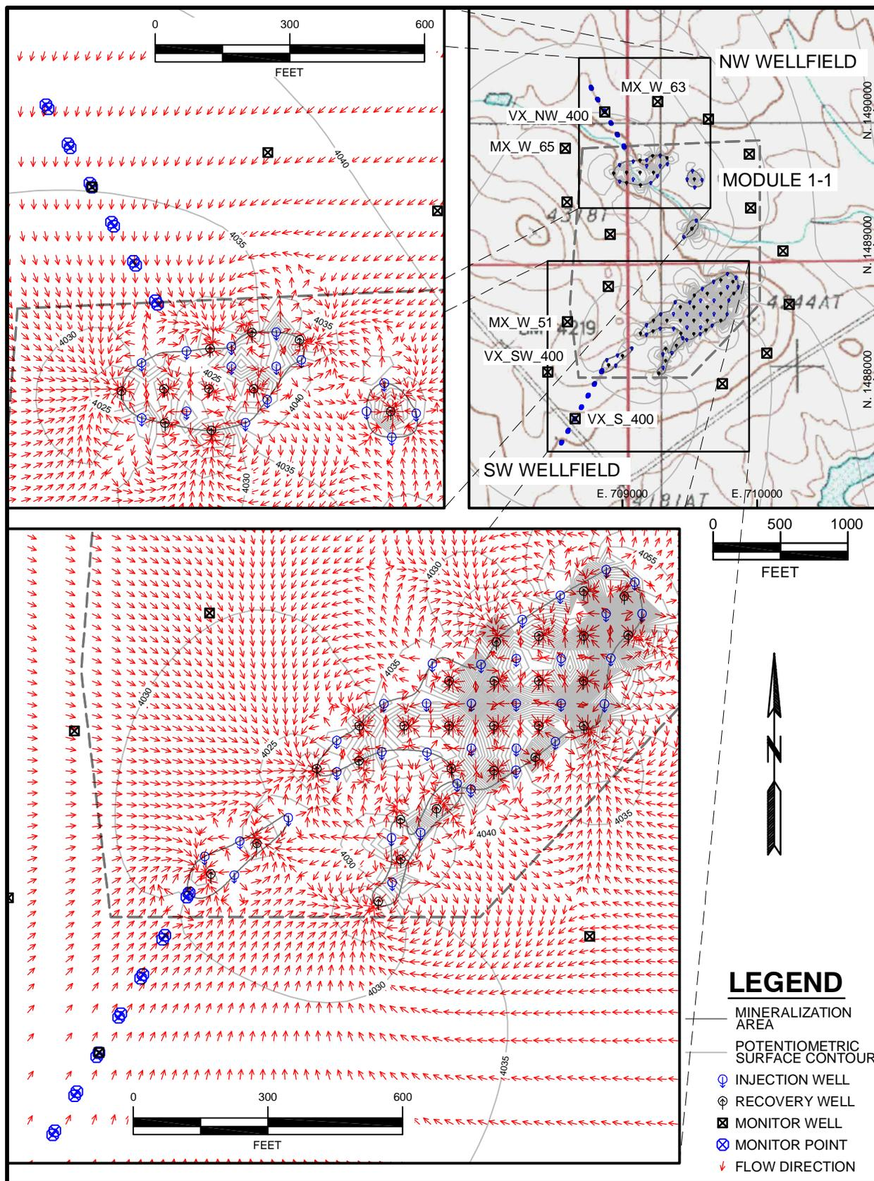
Figure 4.11-4. Groundwater Flow During Normal ISR in Module 1-1
