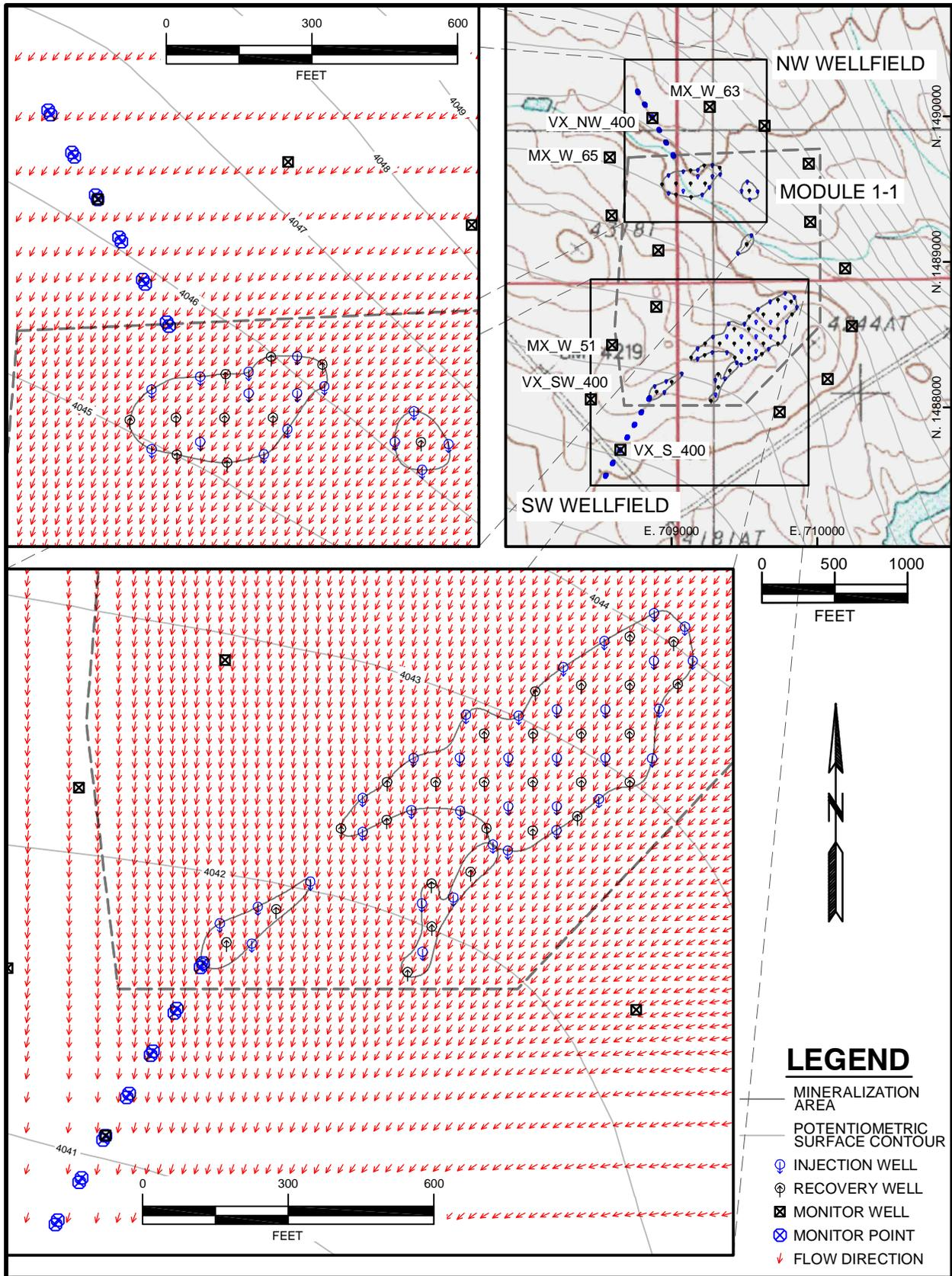
Figure 4.11-1. Pre-ISR Groundwater Flow in Module 1-1
