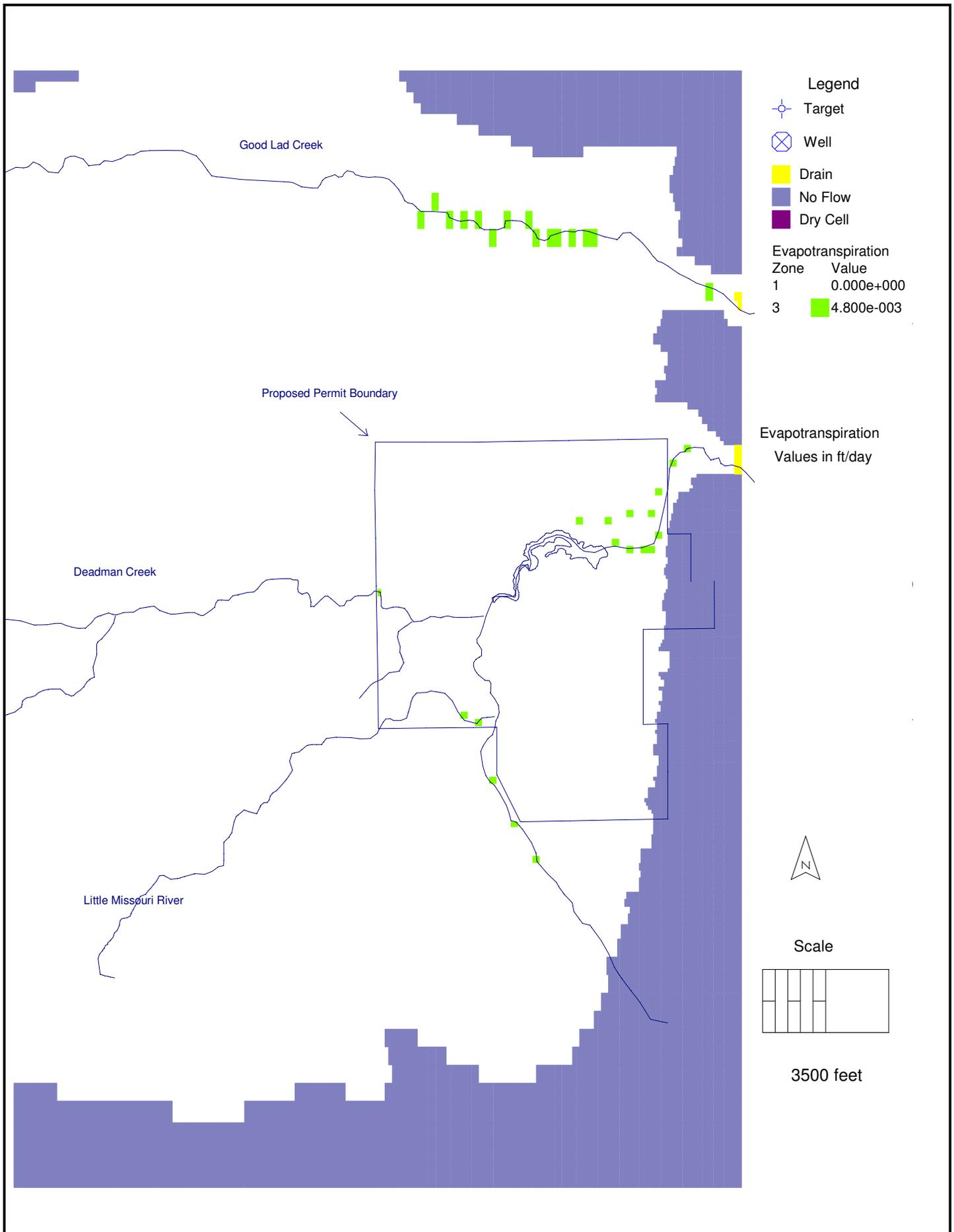
Figure 4.3-1 Spatial Distribution of Evapotranspiration and Drain Cells
