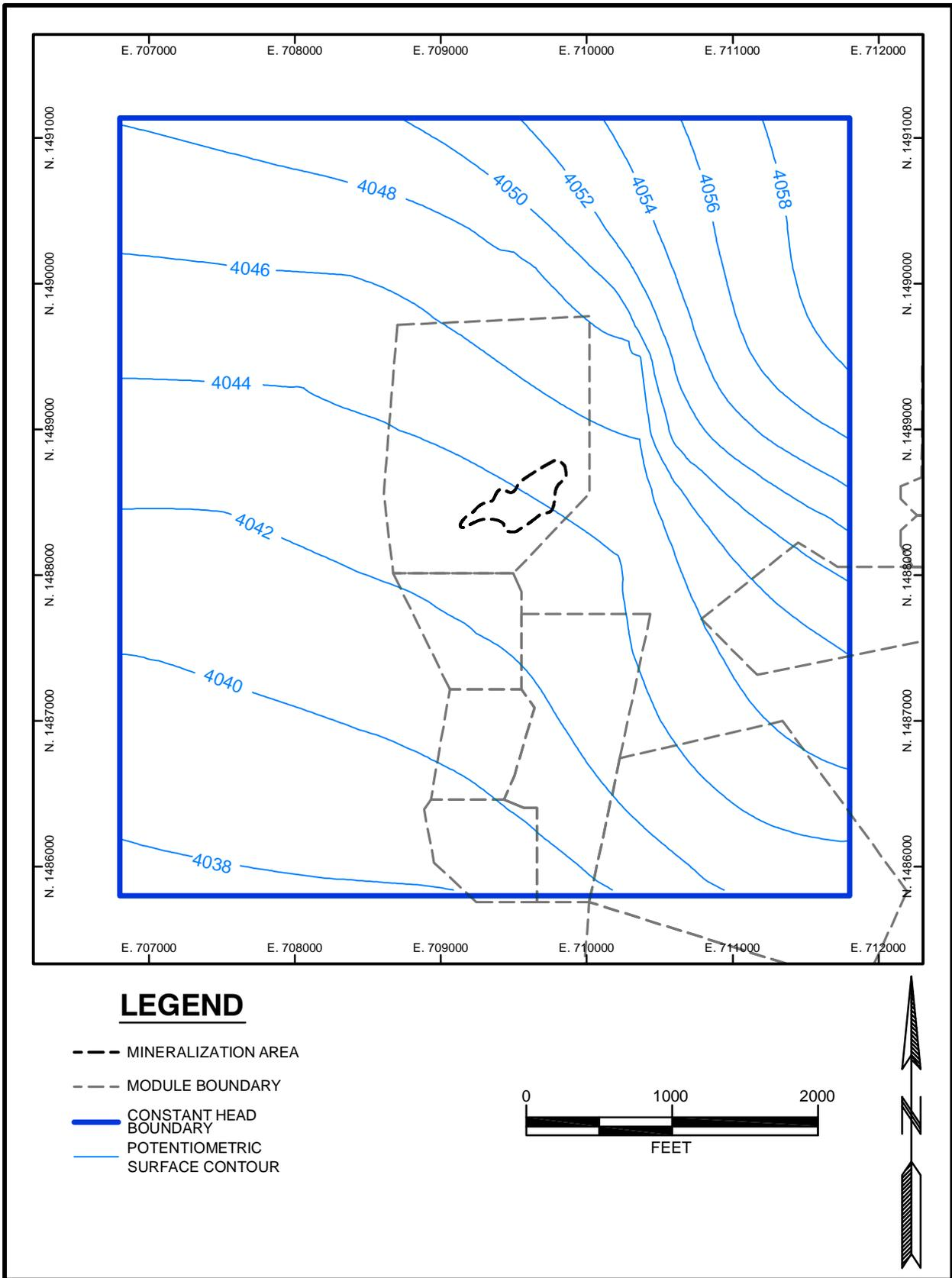
Figure 4.12-1. Refined Model Domain with Pre-ISR Potentiometric Surface
