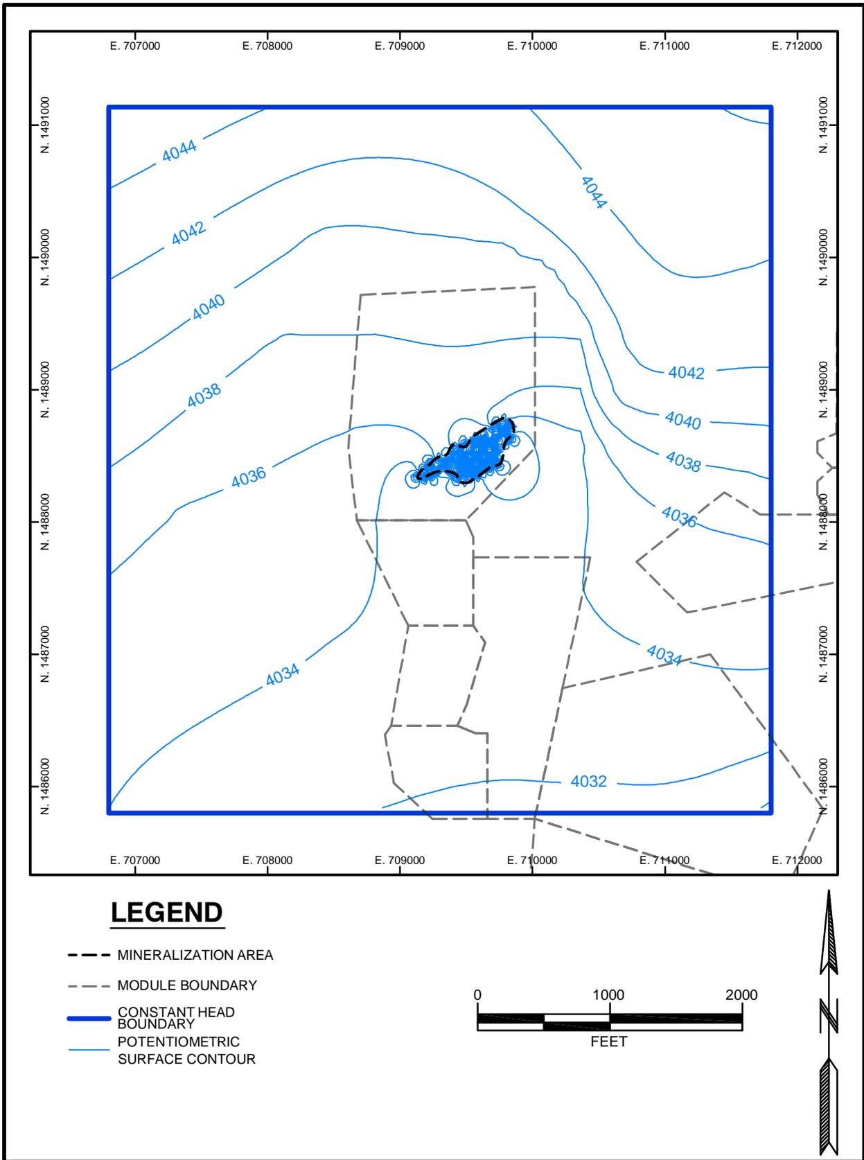
Figure 4.12-3. Potentiometric Surface After 21 Months of ISR Operations
