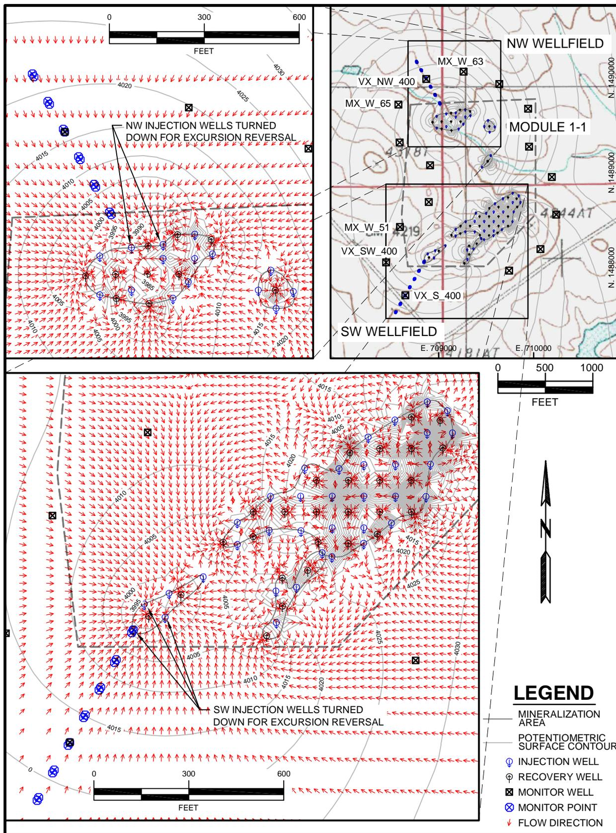
Figure 4.11-6. Groundwater Flow During Excursion Reversal in Module 1-1
