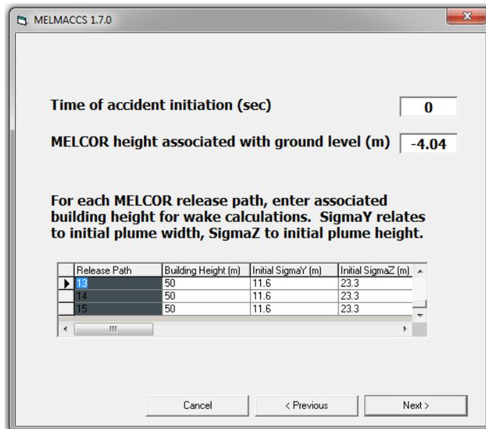
**Figure 4-3 MELCOR release paths into the environment, MELCOR time of accident initiation, height of ground level in MELCOR reference frame, and initial plume dispersion parameters**
