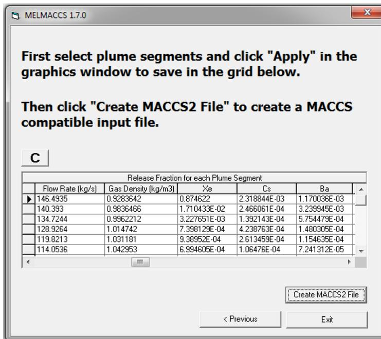
Figure 4-9 Definition of plume segments (flow rate through barium release fraction)
