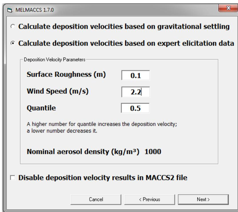
**Figure 4-4 MELMACCS parameters for calculating deposition velocity**
