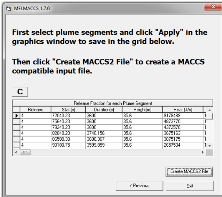
Figure 4-8 Definition of plume segments (release path through heat)
