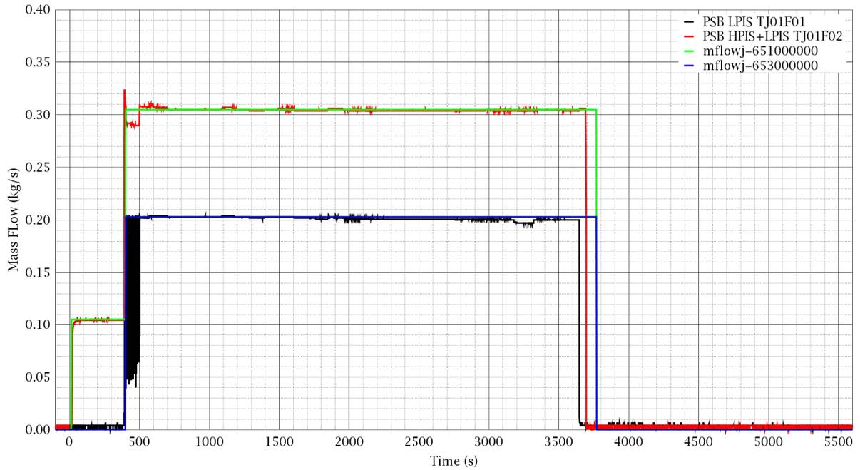
Figure D-5: HPIS + LPIS Flow (Boundary Condition)
