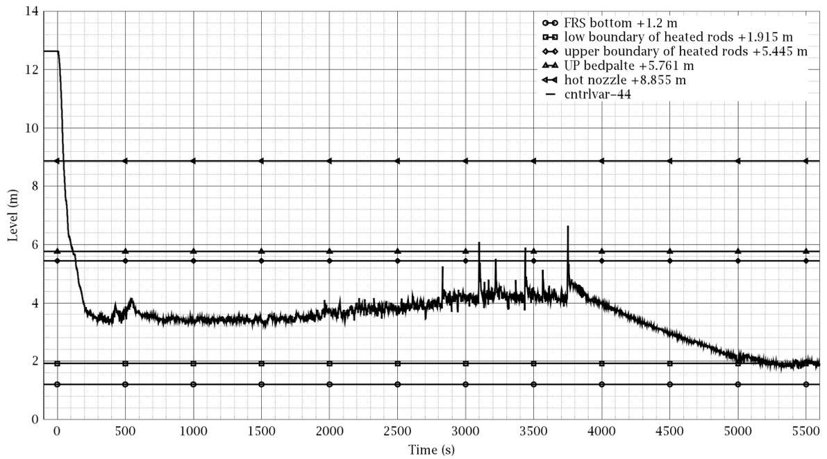
Figure D-22: Reactor Collapsed Level
