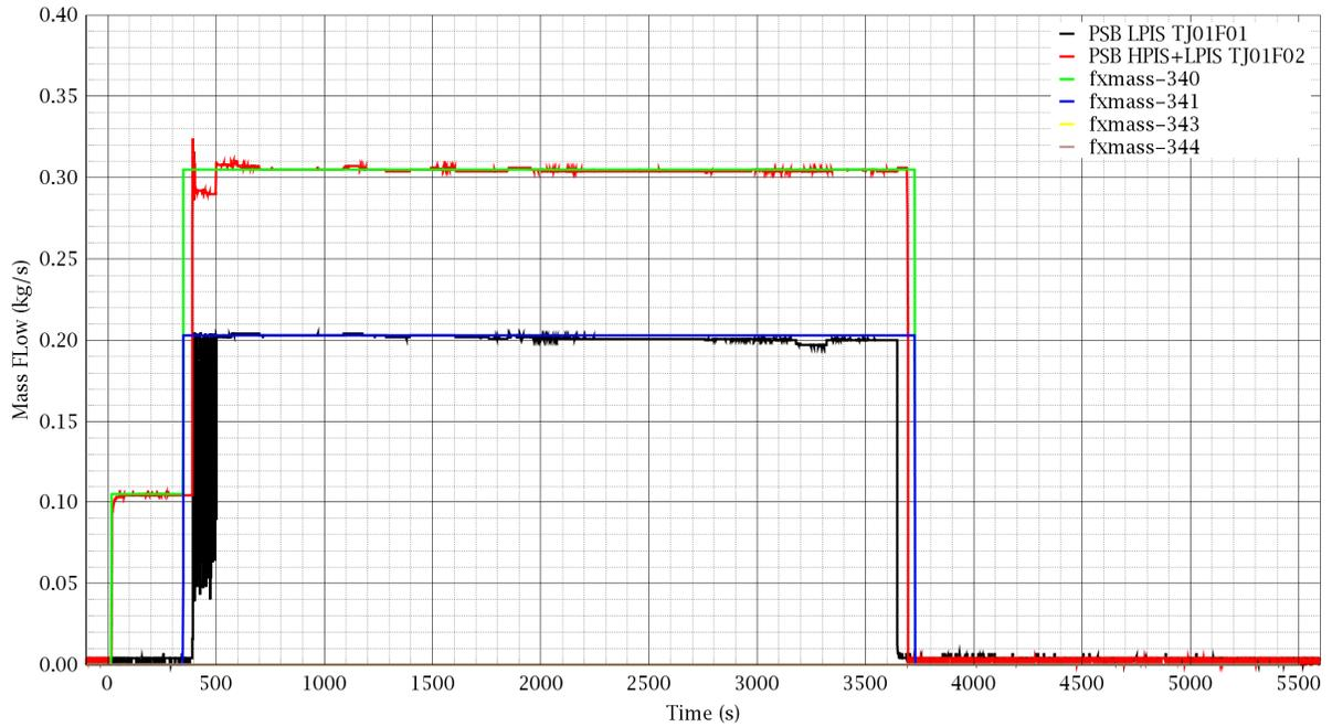
Figure C-5: HPIS + LPIS Flow (Boundary Condition)
