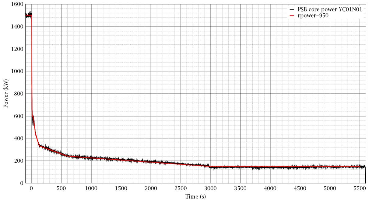
Figure C-9: Fuel Rod Simulator Power (Boundary Condition)
