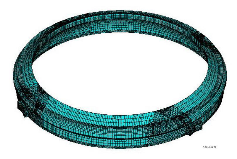
Figure 3E.1.3-2—Isometric View RCB Ring Girder
