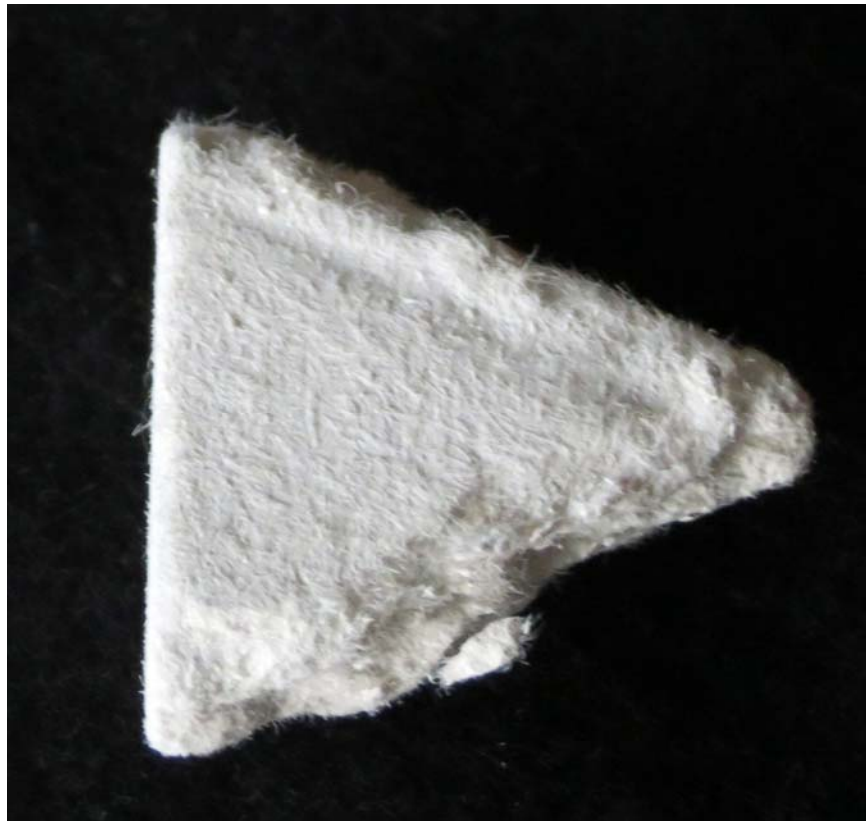
Figure 2: Marinite Board, ~3 centimeters long, Surface Roughness R_a = 6.3\text{ }\mu\text{m}
