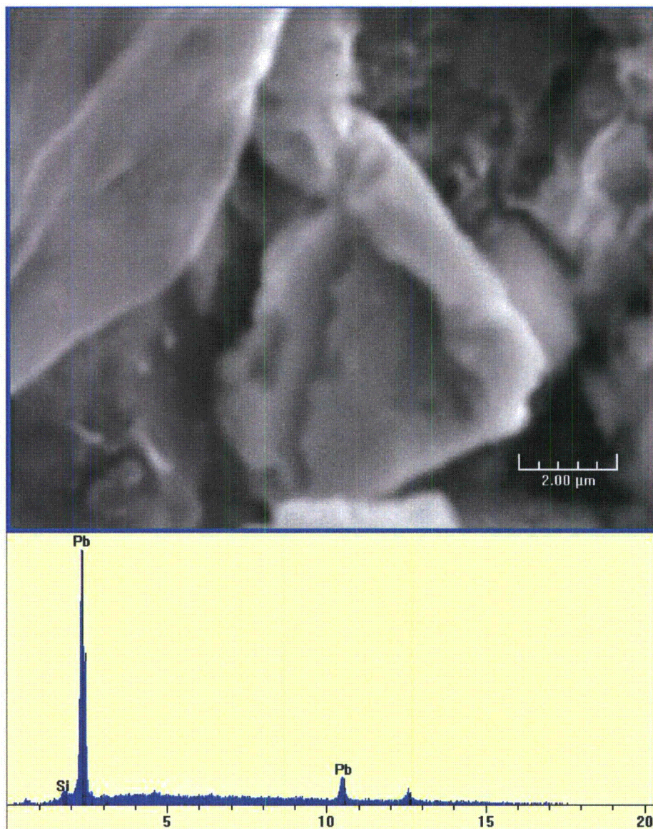
Client Sample No. CX-2 36.5-38 SEM image of a triangular grain of possible Pb carbonate – 8,500X.
