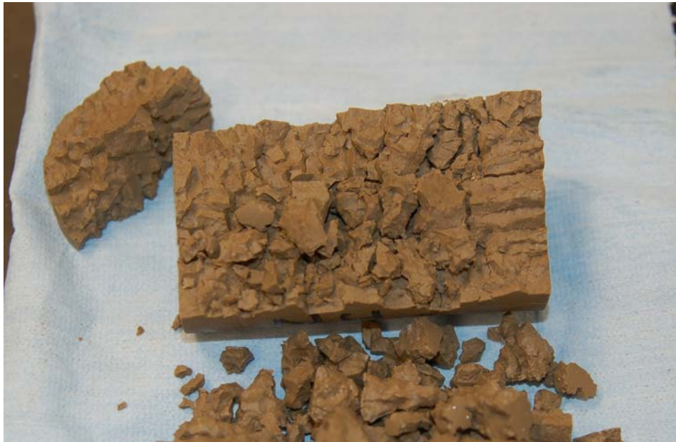
Figure 3-14 Cast cylinder of GVS111 after rehydration and cracking.
