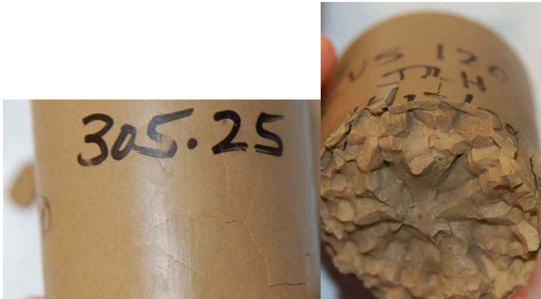
Figure 4-6 Photographs of GVS120 after drying and rehydration (left side) and breakage (right side).
