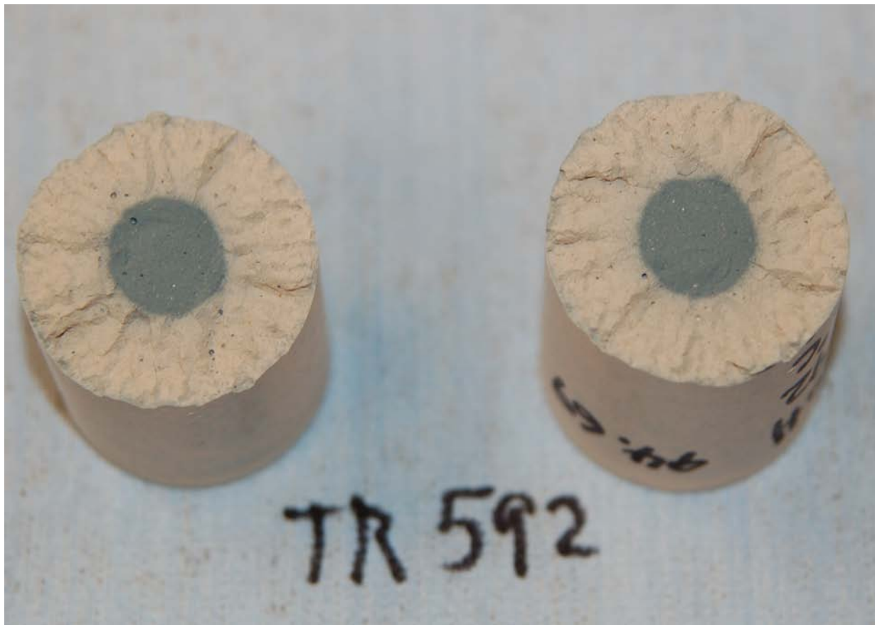
Figure 3-16 A partially dried cured sample (2 inch diameter) from premix and 3.0 M NaOH at 0.60 w/cm ratio and cured at 22 °C. This sample was easily broken by hand.
