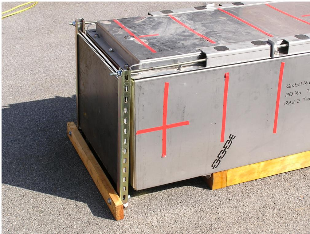
**Figure 2-24 Addition of Tare Weight to CTU 2**
