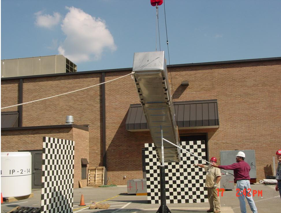
**Figure 2-26 Alignment for Oblique Puncture**
