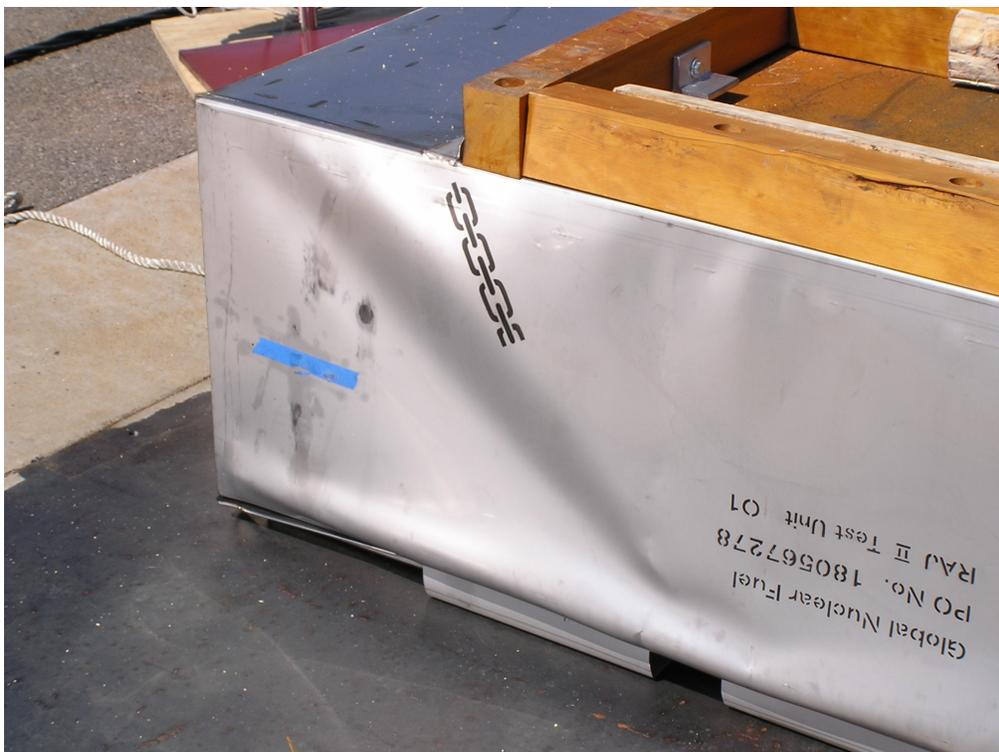
**Figure 2-30 Secondary Impact End Damage**
