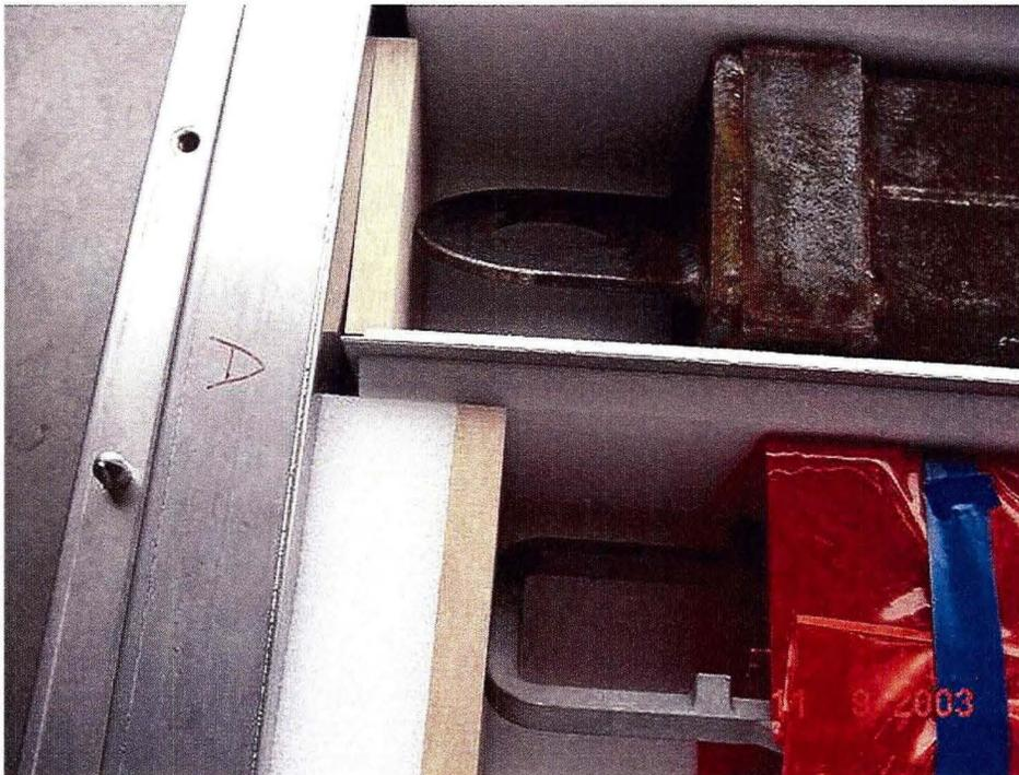
**Figure 2-18 Top End Fittings on Fuel in CTU 1**
