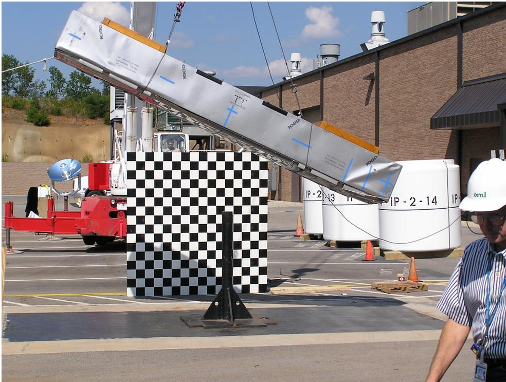
**Figure 2-27 Position for Puncture Test**
