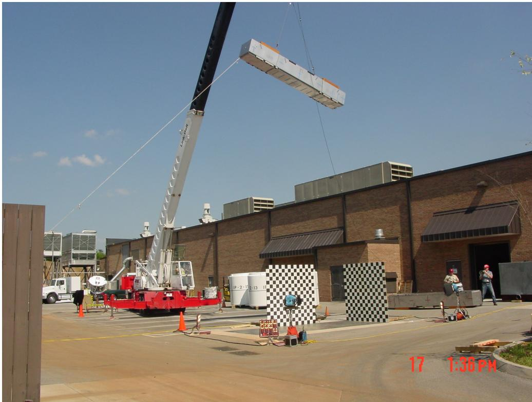
**Figure 2-25 CTU 1 Positioned for 15° 9-m (30-foot) Slap-down Drop**
