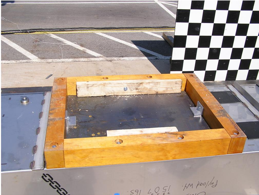
**Figure 2-23 Addition of Tare Weight to CTU 1**
