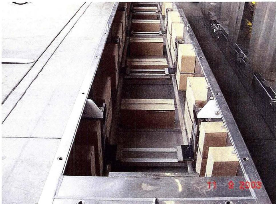
**Figure 2-20 Outer Container without Inner Container**
