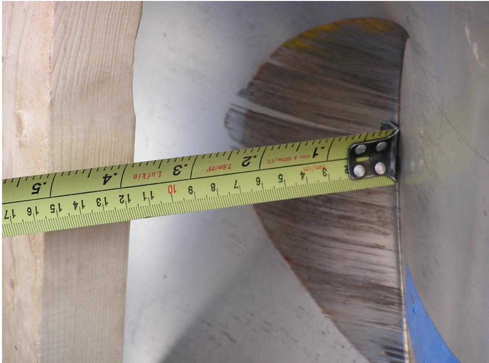
**Figure 2-32 Close Up of Puncture Damage**
