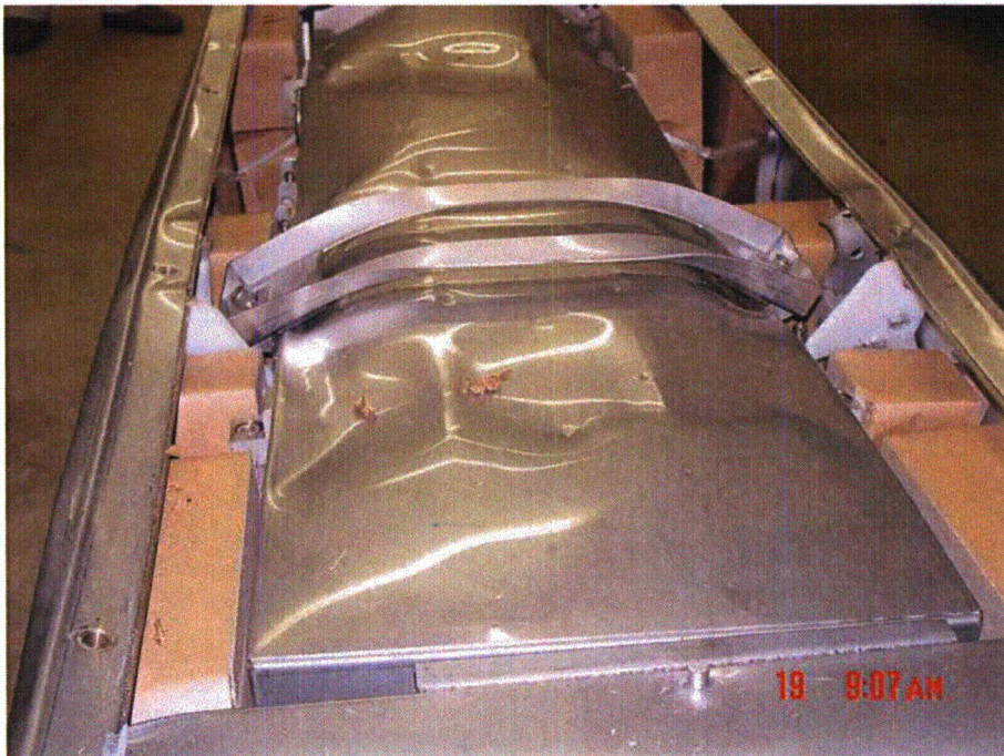
Figure 2-36 Damage Inside Outer Container to CTU 1
