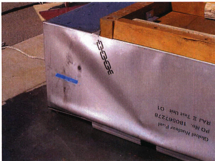
Figure 2-30 Secondary Impact End Damage
