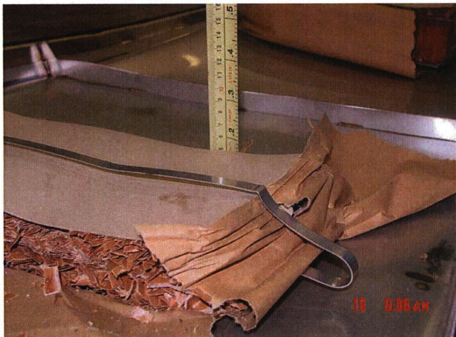
Figure 2-38 Lid Crush on CTU 1
