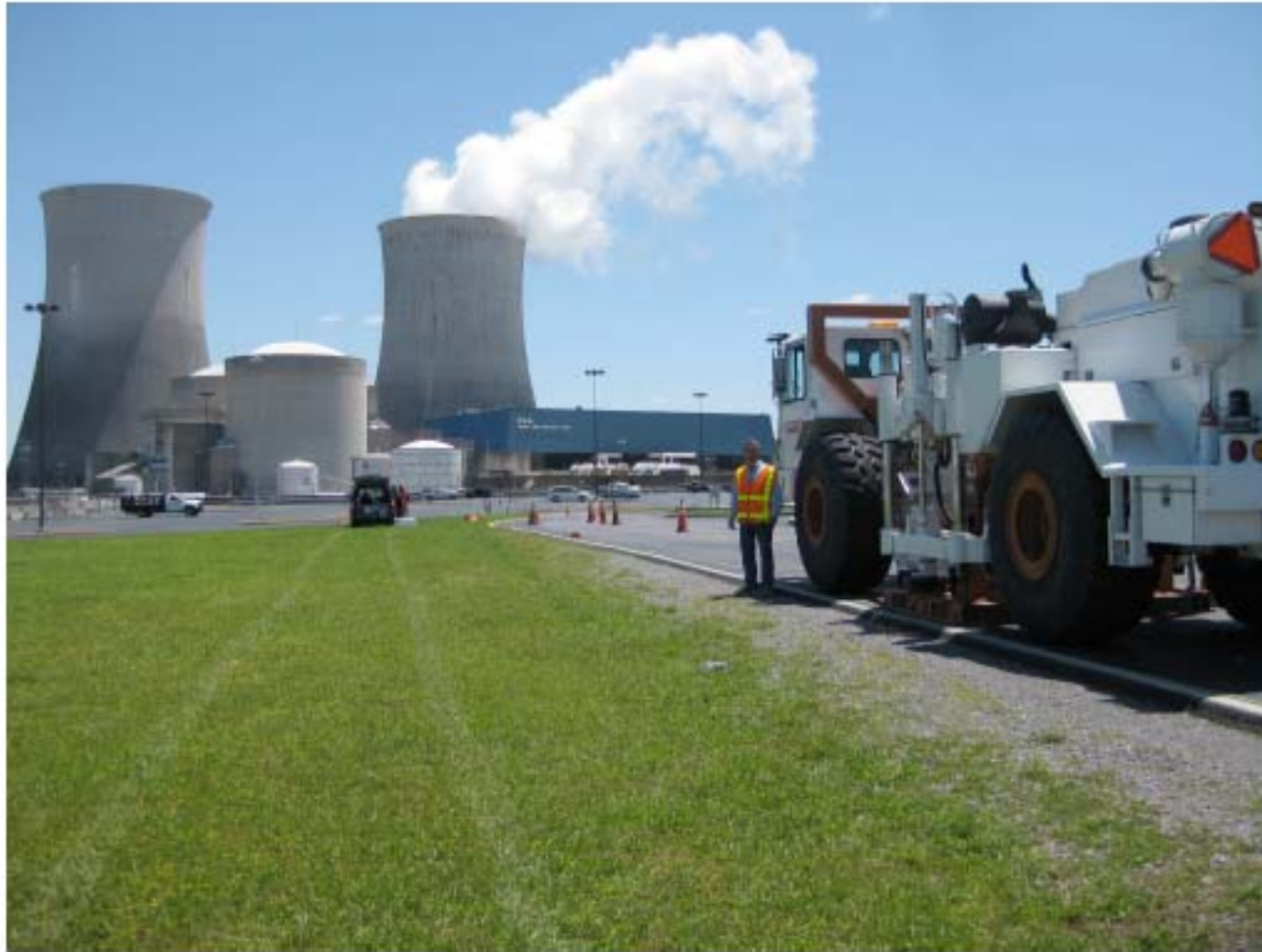
Figure 11 Photograph of Liquidator Used in SASW Testing at Site 8 at Watts Bar #2 Nuclear Power Plant
