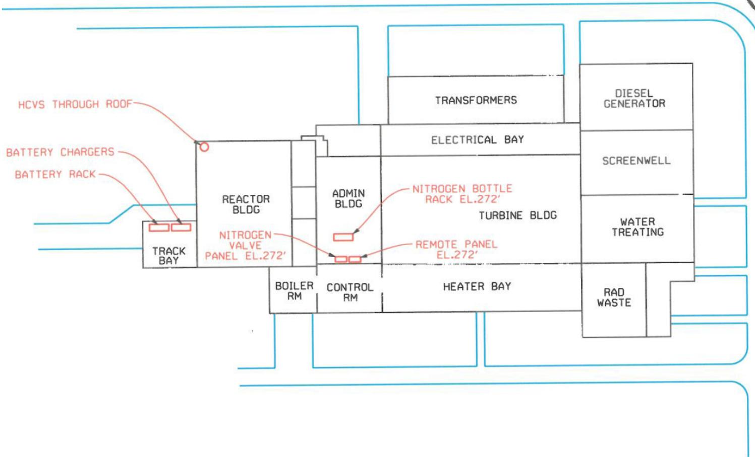
**Sketch 3.D: Plant Layout – Site Plan of HCVS Piping, ROS, N2 Bottle Station, and Battery Station**
