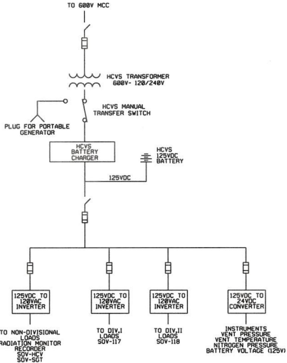
Sketch 1.A: Electrical Layout of System – One Line Diagram
