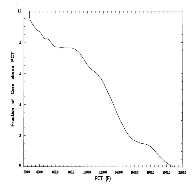
Figure 2.3 Fraction of Core Exceeding a PCT (Data taken from Reference 2.3.1 Switchover analysis for EOC Radial power conditions)
