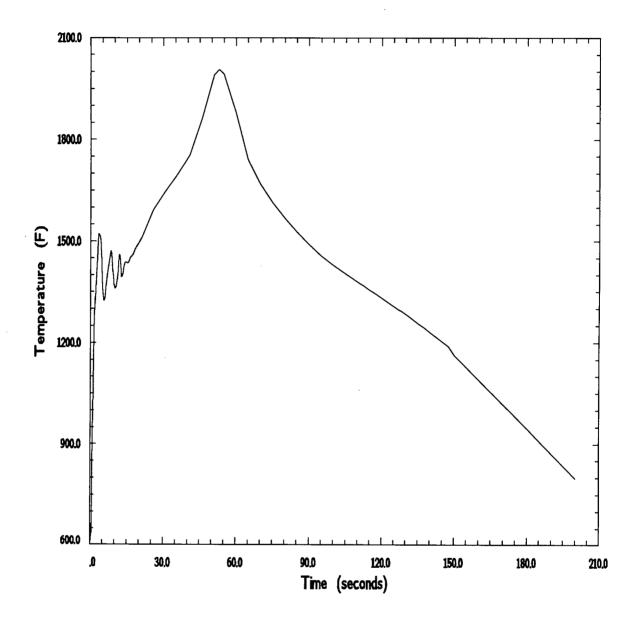
Figure 2.1 Cladding Temperature at PCT Node (8.75 ft) - Initial Phase (Data taken from Reference 2.3.4 LBLOCA initial blowdown phase)
