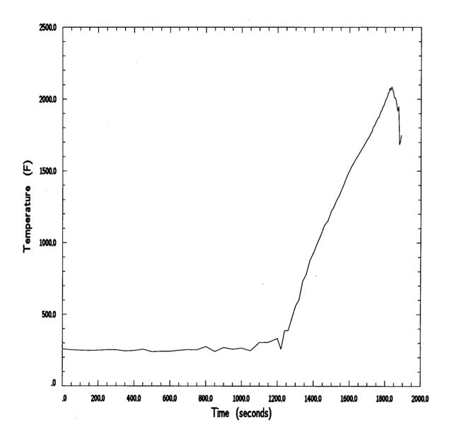
Figure 2.2 Cladding Temperature at PCT Node (8.75 ft) - Switchover Phase (Data taken from Reference 2.3.1 Switchover analysis)
