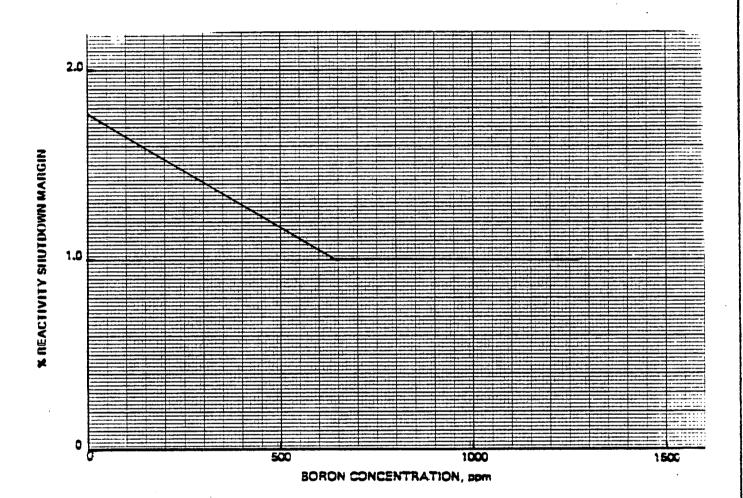
Figure 3.10-2 SHUTDOWN MARGIN VS BORON CONCENTRATION
