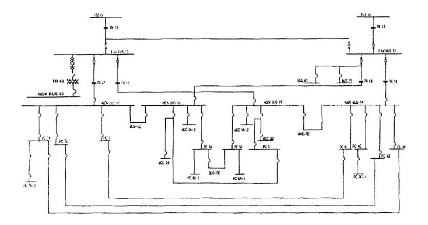
The Unit 1 4KV Power Distribution System is comprised of Transformer 12, Transformer 13, 4KV Bus 11 and 4KV Bus 12. The purpose of the Unit 1 4KV Power Distribution System is to distribute 4KV power to the Unit 1 480V Secondary Unit Substations 14, 15, 16, 17, the Station Blackout Facility and the Unit 2 TB outage Power Bus 43. There are no other loads connected to the Unit 1 4KV Power Distribution System.
