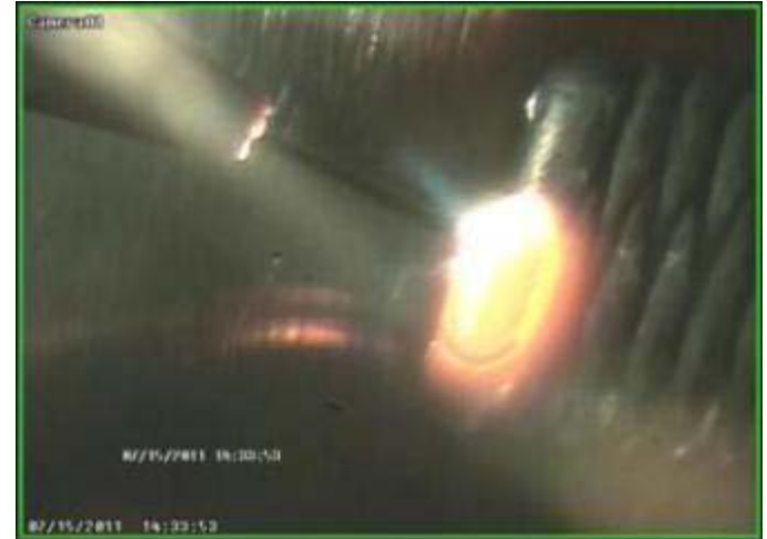
Low dilution laser welding process with constant wire feed.
