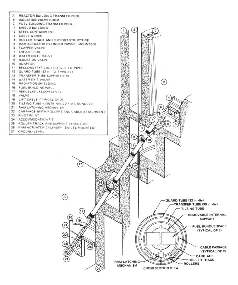
Figure 6.2-11 Mark III Inclined Fuel Transfer System (IFTS)
