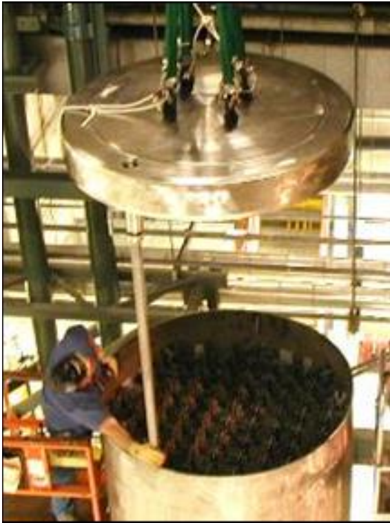
(a) MPC Lid Test Fit During Initial Preparation
