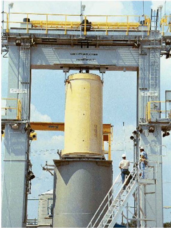
(a) Transfer of MPC from Hi-Trac to Hi-Storm
