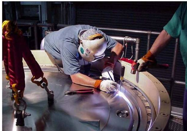
(c) MPC Lid Welding Operations
