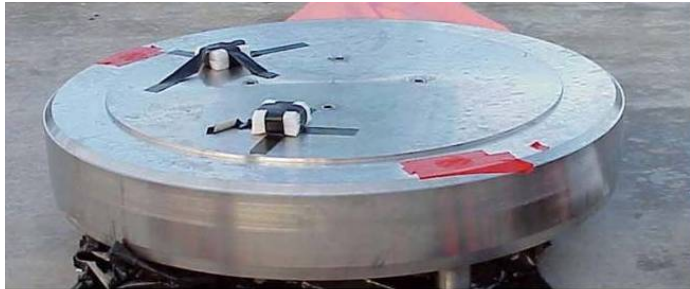
(a) Hi-Trac Raised While Being Drained
